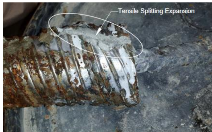
Figure 3.3: Splitting expansion failure of corrugated duct.
