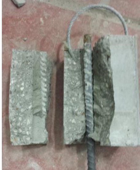
Figure 3.8: Tensile splitting of grout and surrounding concrete for specimen 12EN-2.
