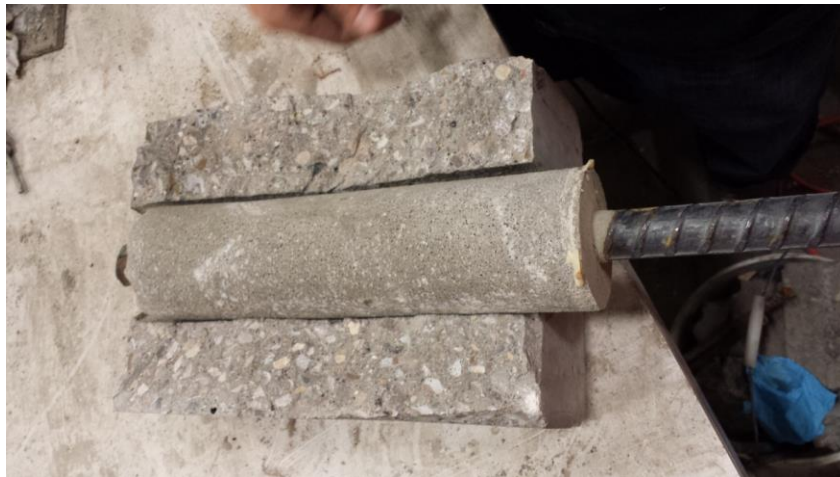
Figure 3.4: Tensile splitting failure of the concrete block for specimen 12CN-2.
