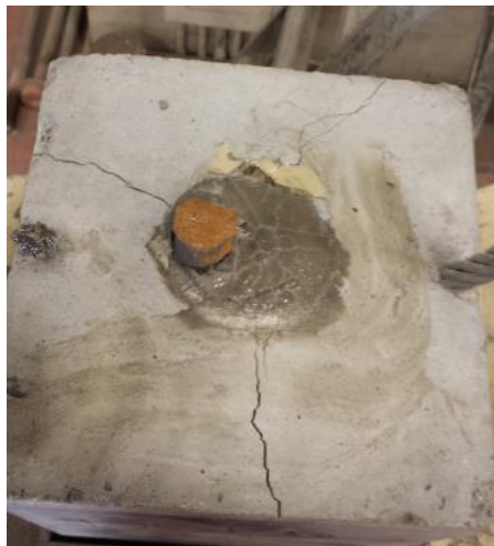
Figure 3.7: Tensile splitting of surrounding concrete for specimen 12ED-1.
