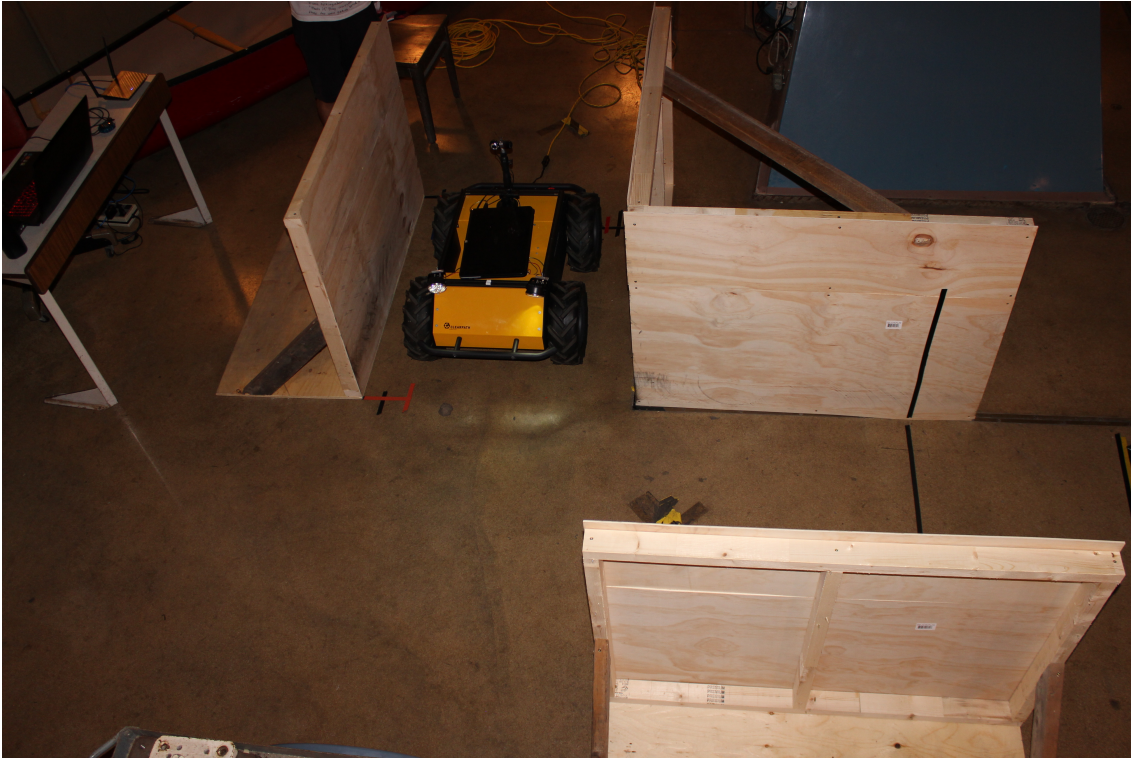
Figure 7.7: The corridor walls were higher than the field of view of the monocular camera. The tele-operator had to navigate around the corner using the limited spatial cues visible in the field of view, including placement of the walls. Shown with an aperture width of 95 cm
