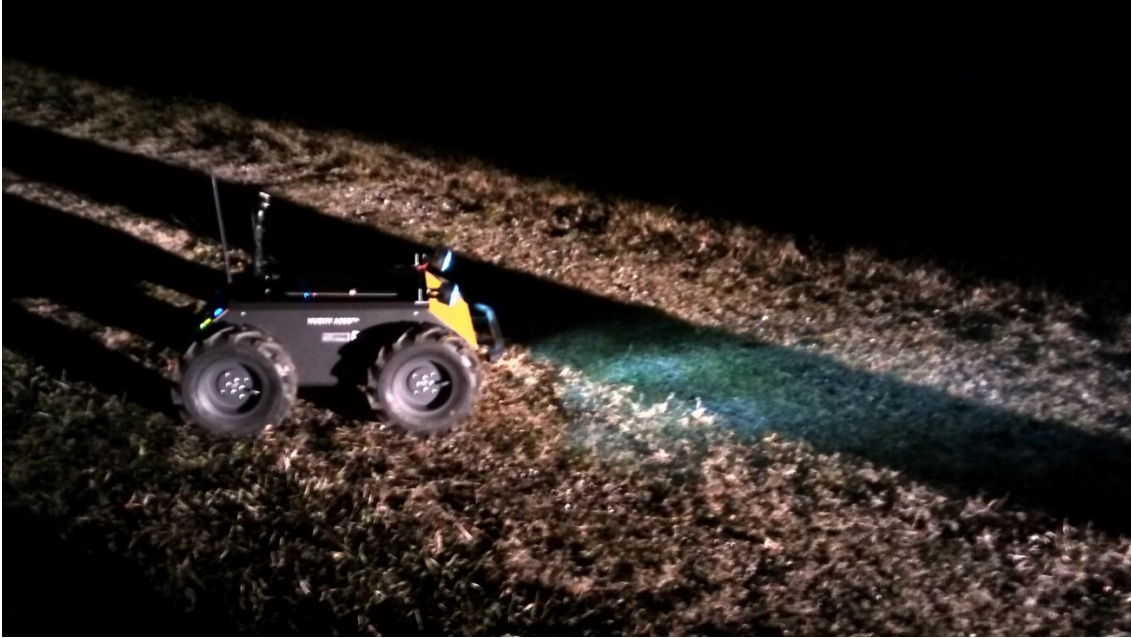
Figure 7.4: The tele-operated rover provides streaming video for the user.
