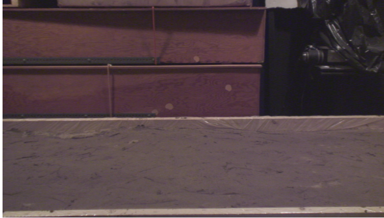
Figure 6.9: Flattened wet sand in the terrain box without the aggregate.
