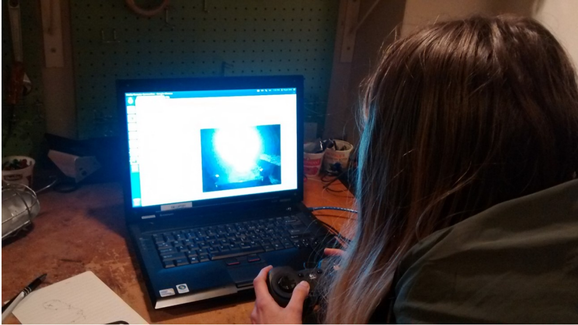
Figure 7.3: The user tele-operates the rover through an interface using a gamepad.
