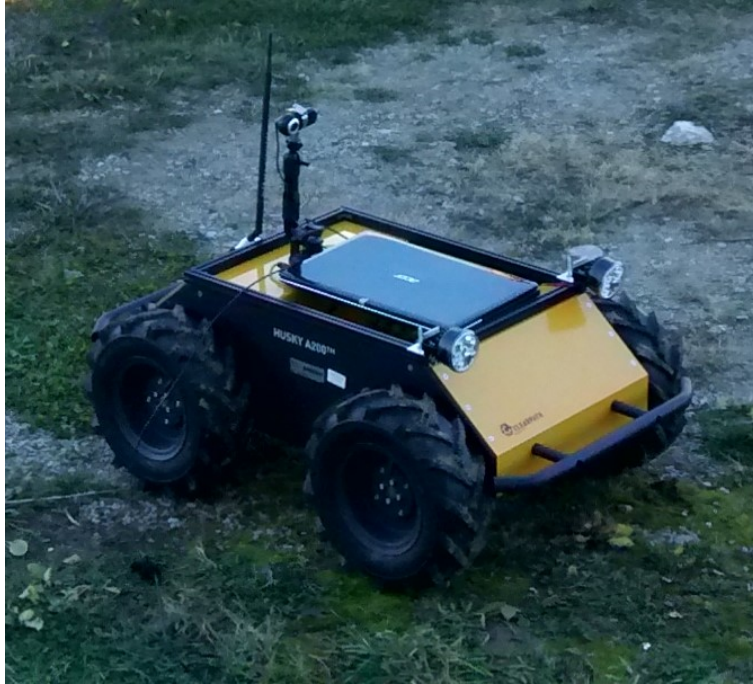
Figure 7.2: The Husky A200 mobile robot shown outdoors for the tele-operation testing.
