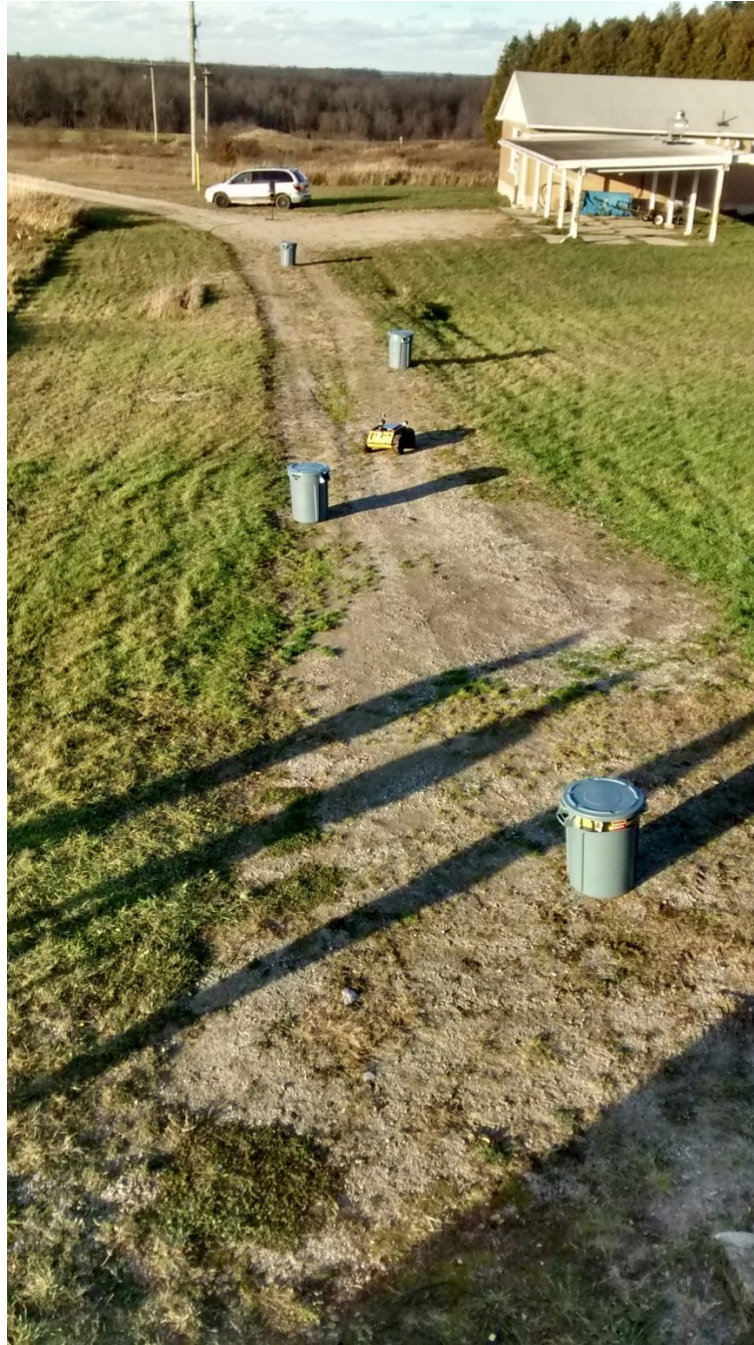
Figure 7.5: The first test circuit was a double figure 8; when repeated once the total drive distance is approximately 180 m .
