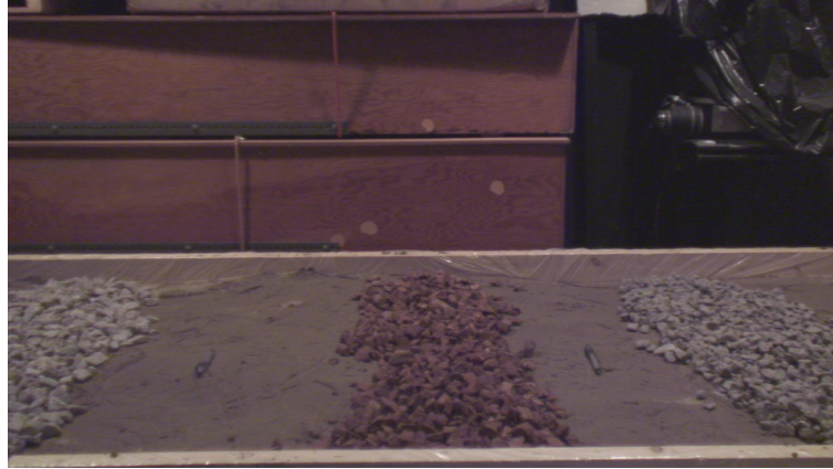
Figure 6.7: Three strips of aggregate laying upon flattened wet sand in the terrain box.
