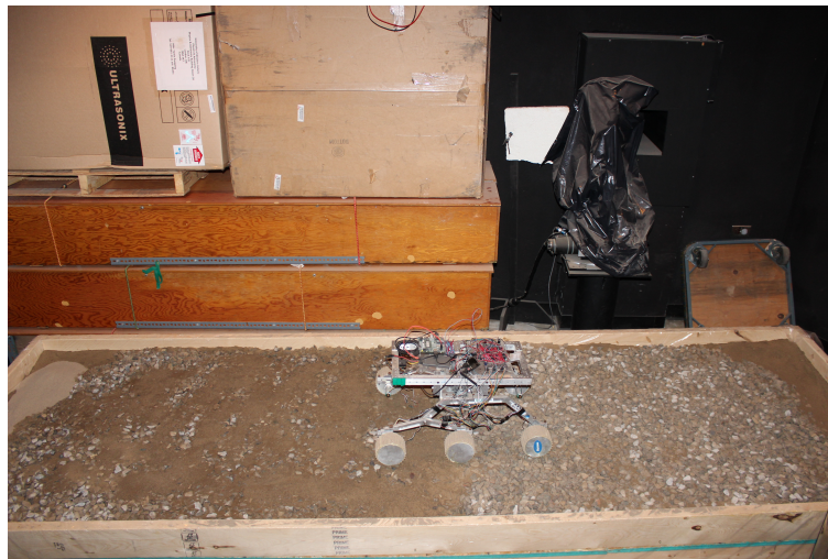
Figure 6.1: The terrain box contained a layer of sand and additional material was added and removed from it. The box rested on two jacks (right side, not shown) to raise and lower the box to create a 5°incline, shown in Figure 6.2. In this image, the gravel covered the bed with the left side covered in wet sand.
