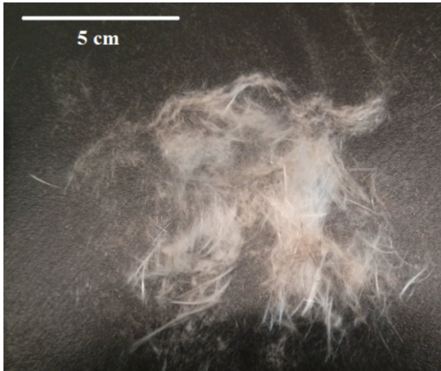
Figure 1.2: Fibers after a burn test from LFT-D charge.
