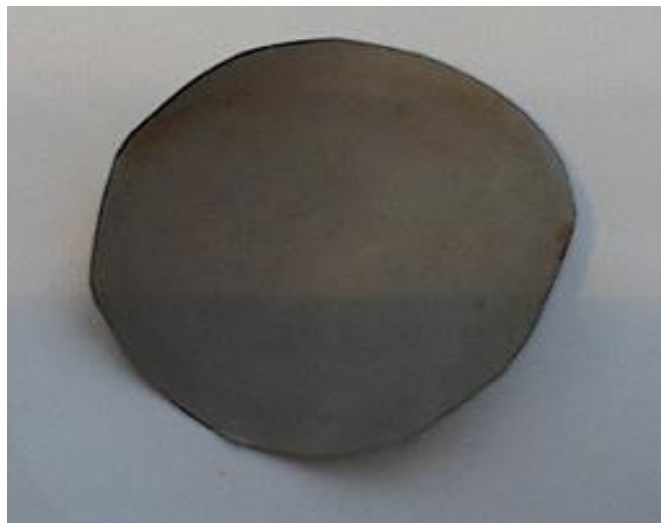
Figure 3.9: TFC membrane prepared on a support made with 0.1% modified MWCNTs and 20% PSF; the active skin layer is the result of the interfacial polymerization between 2% MPD and 0.1% TMC
