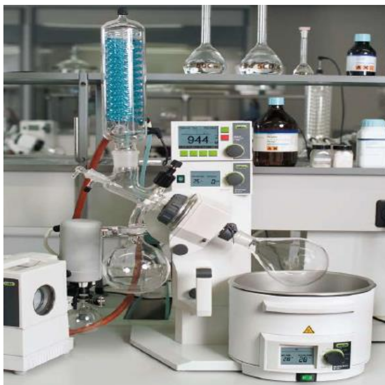
Figure 3.2: BÜCHI Rotavapor used to evaporate the sample obtained after LLE
