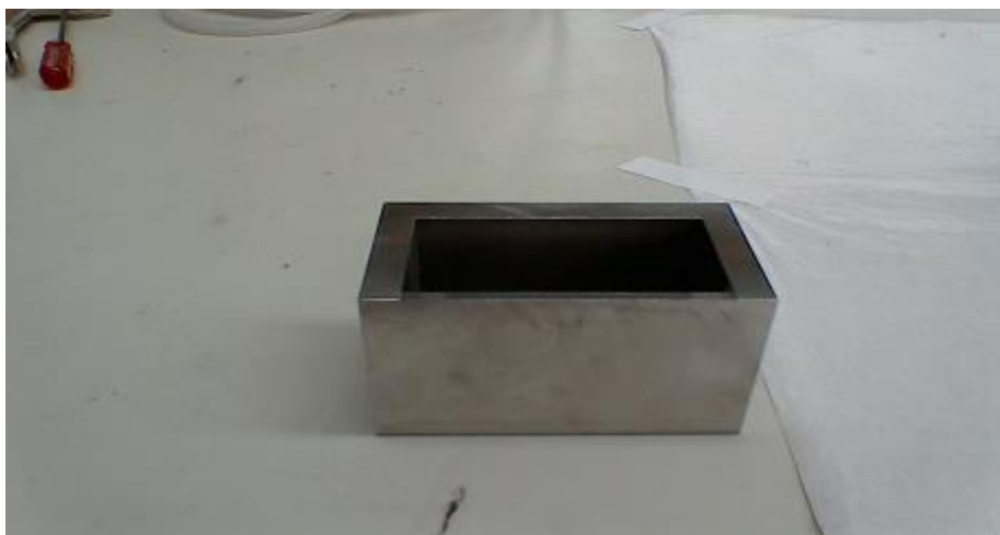
Figure 3.7: Custom-made Doctor Blade used to cast 20% PSF support membrane
