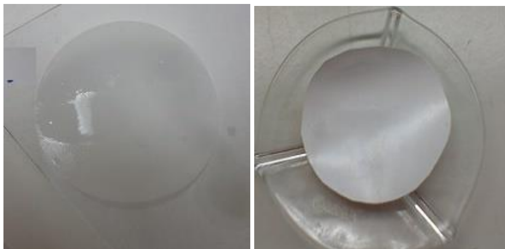
Figure 3.8: 2.5% PTFE/PDMS (left) and 2.5% PSF/PDMS (right) membranes prepared in lab. The shiny surfaces prove the cross-linked PDMS layer on the supports.
