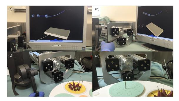
Figure 2.5: (a, b) A side-by-side view of the actual and virtual robot, which was programmed using the Virtual Reality Modeling Language (VRML) in Simulink. (c) The developed CTR prototype in a positioning task controlled by a haptic device. (d) The developed CTR prototype in a surface pattern tracking task.
