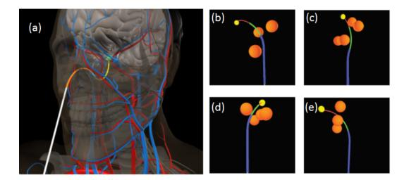
Figure 1.13: (a) Simulation of a CTR in a neurosurgery environment executing the motion plan that calculated from the proposed sampling-based approach based on the Rapidly-Exploring Roadmap. The robot is inserted through the nostril and guided toward the pituitary gland (highlighted in green) in the skull base while avoiding skin, bone, blood vessels, and healthy brain tissue. (b, c, d, e) Simulation of a CTR in four different spherical obstacle environment [54] (© 2011 IEEE).
