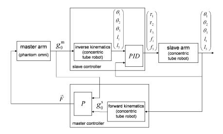
Figure 1.11: The unilateral control block diagram of a teleoperated CTR;  $\theta_i$  and  $l_i$  are the joint space variables of the  $i^{th}$  tube [1] (© 2010 IEEE).
