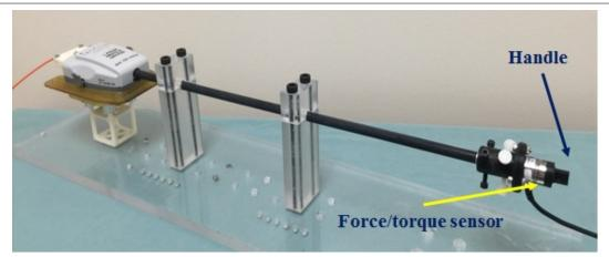
Figure A.12: Experimental setup for evaluating the performane of force sensing.
