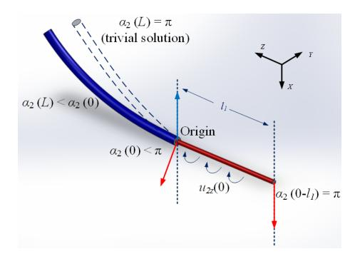
Figure 5.1: Demonstration of the possible multiple solutions for two tubes with a straight section. The blue and red arrows represent the rotational angles of the two tubes at that location.
