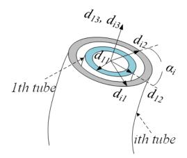
Figure 3.2: Body frames of tube i and the 1st.
