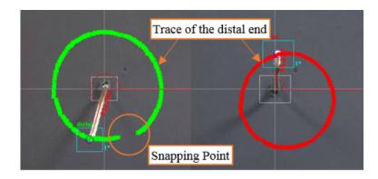
Figure 1.7: Snapping analysis through video tip tracking [32]. Green marks (left) show the traced distal end of an unstable tube pair that snaps at a certain point, and red marks (right) show the traced distal end of a stable tube pair (© 2014 IEEE).
