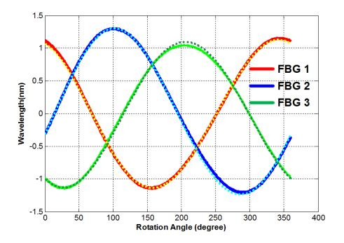
Figure 7.8: The solid lines are the wavelengths reflected from three FBG sensors that are helically-embedded in a curved tube. The wavelength output of each FBG was biased at the beginning of the test. The dashed lines are the corresponding values from the force-curvature-strain model using the calibrated parameters listed in Table 7.3.
