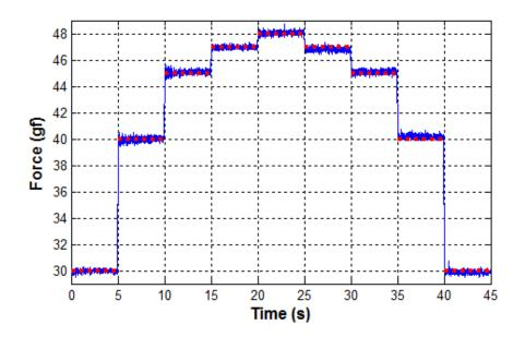
Figure 7.19: Comparision of the theoretical force values (red) and the measured force values from the sensorized CTR (blue).
