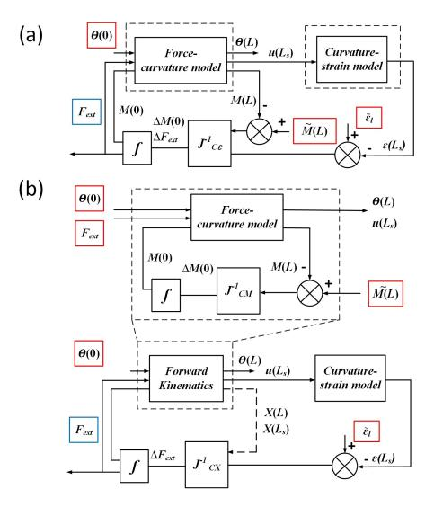
Figure 7.21: Signal flow diagram for two strain-force calculation methods. (a) Previous strain-force calculation method. (b) Alternative Strain-force calculation method. The red blocks represent the inputs of these calculations and the blue ones are outputs.
