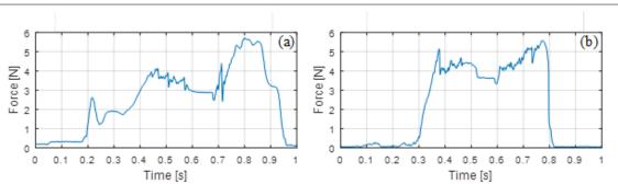
Figure A.9: The force profiles of one novice (a) and one expert surgeon (b) when performing Hem-O-Lock tightening, measured by the FBG sensors.
