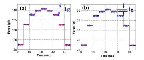
Figure 7.13: Two set of weights were put on the tube tip to test the resolution of the proposed force sensing technolgoy. In (a), the weights are 120g, 130g, 135g, 137g, 138g. In (b), the weights are 70g, 80g, 85g, 87g, 88g. The blue lines are the measured forces using FBG sensors and the red lines are the theoretical gravity values.
