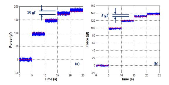
Figure A.14: Comparision of the theoretical force values (red) and the measured values from the sensorized instrument (blue).
