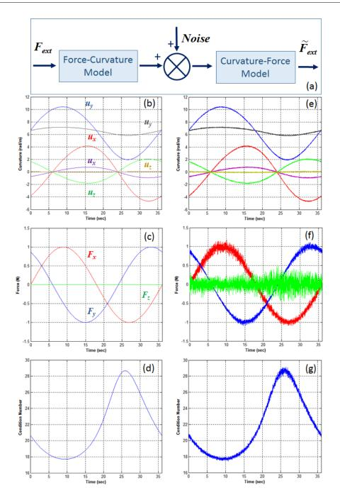
Figure 7.25: Simulation studies for 3D force sensing, using curvature measurements of two sensorized cross-sections. (a) Simulation signal flow. (b, c, d) Simulation results when the noise level is zero. (e, f, g) Simulation results when the noise level is around 2% of the curvature signals. (d, g) Condition numbers of  $J_{CX}$  in Eq. (7.46), which is the update strategy for the strain-force calculation.
