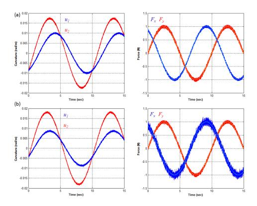
Figure 7.27: Demonstration of the relation between condition number and noise amplification in curvature-force calculations. (a) The condition number is 2.6; (b) the condition number is 5.8.
