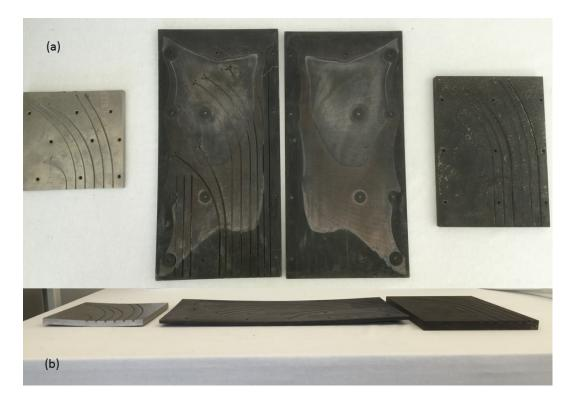
Figure 2.1: Molds used for shaping Nitinol tubes. From left to right, they are made of a half inch aluminum plate, two 1/4 inch low-carbon steel sheets (lid and the bottom pieces), and a half inch low-carbon steel plate. (a) Top view of the three molds (b) Side view of the three molds.
