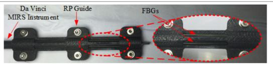
Figure A.3: Illustration of the 3D printed installation guide for FBG alignment.
