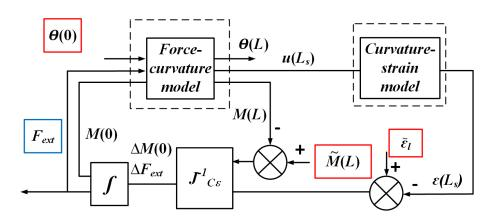
Figure 7.3: Signal flow digram for Strain-Force Calculation. The boundary conditions in red blocks are the inputs of the model chain. One of the outputs of this calculation is the tip force measurement (the blue block).
