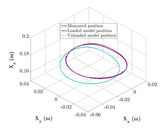
Figure 6.6: Model validation: comparison between measured and predicted tip positions using loaded and unloaded schemes.
