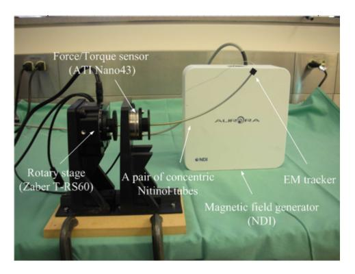
Figure 3.3: Experimental setup for evaluating kinematic model.
