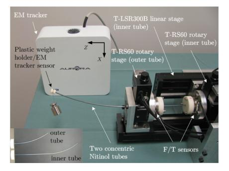
Figure 4.7: Our concentric-tube robot setup.
