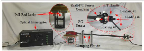
Figure A.4: The experimental setup for calibrating and evaluating the sensorized instrument.
