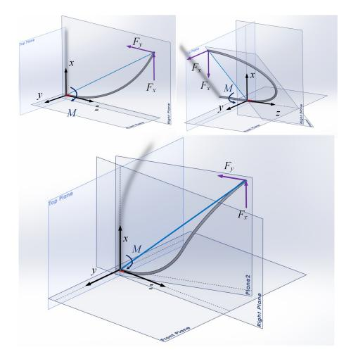
Figure 7.24: Three examples of unobservable forces. In these cases, the force vector cannot be decoupled into two elements by using strain sensors on a single cross-section.
