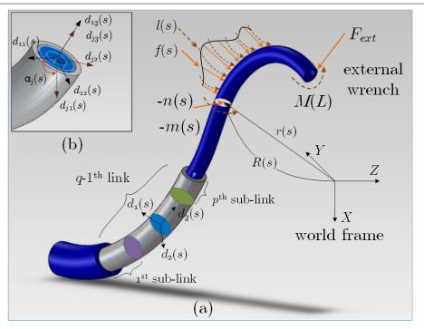
Figure 6.1: (a) A loaded concentric-tube robot consisting of q links or tubes each of which is composed of p sub-links [3]; (b) the robot's cross section showing coordinate frames associated with the 1<sup>st</sup> and the j<sup>th</sup> tubes [9].
