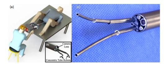
Figure 1.5: An illustration of the robotic system for HoLEP. The surgeon is able to position and angle the endoscope while simultaneously controlling two CTRs that extend from its tip. (a, b) The CAD design of the robotic surgical setup. (c) Distal end of the actual CTRs and endoscope [15] (© 2014 IEEE).
