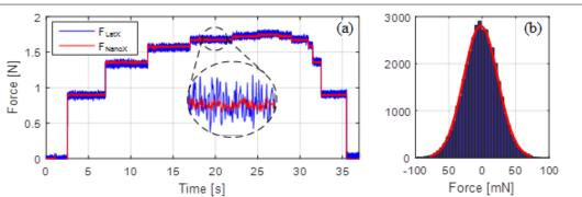
Figure A.5: (a) Force values measured from the FBG and Nano17 sensors in response to a series of weights applied to the sensorized instrument (b) Error histogram of the FBG force measurement.
