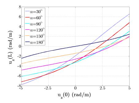
Figure 4.4: The relationship between boundary conditions:  $u_{iz}(L)$  with respect to  $u_{iz}(0)$  as a function of the rotation angle in a two-tube robot.
