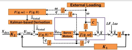
Figure 6.2: Control block diagram for the proposed tracking algorithm.
