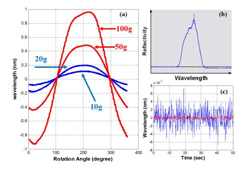
Figure 7.7: (a) Demonstration of the effects of increased bending on the distortion of the FBG sensor output signal. (b) An example of a reflected spectrum with peak distortion. (c) Comparison between the noise from a 1 mm FBG (blue line) and a 5 mm FBG (red line).
