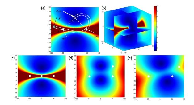
Figure 7.28: Condition number map for designing the shape of a sensorized continuum robot; (a) two sensorized cross-sections for measuring 2D unobservable forces; (b) two sensorized cross-sections for 3D force sensing; (c, d, e) three sensorized cross-sections for measuring 2D unobservable forces.
