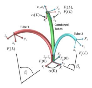
Figure 1.6: Effect of torsional twisting when two curved tubes are combined. Tube coordinate frames are denoted by  $F_i(s)$ . The relative z-axis twist angle between frames  $\alpha(s)$  varies from a maximum  $\alpha(0)$  at the base to a minimum  $\alpha(L)$  at the tip. The central angles  $\beta_i$  are proportional to the precurvature and to the tube length L [1] (© 2010 IEEE).
