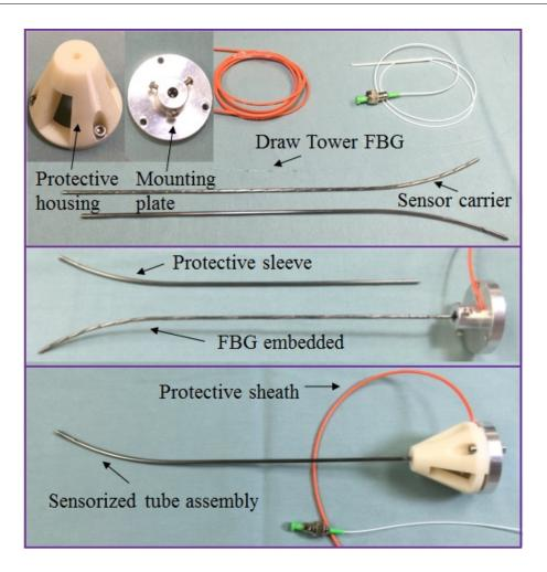
Figure 7.15: The sensorized tube assembly and components.
