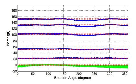
Figure 7.12: The red lines represent the amount of gravity force applied at the tube tip while the motorized stage rotates a full revolution. The blue lines are the force measurements in the direction of gravity  $(F_x)$  while the green lines are the force measurements in the other direction  $(F_y)$ .
