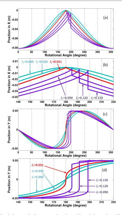
Figure 5.2: Simulation results for a two-tube robot with straight sections. Note that a large number of different  $l_1$  were tested in the program, only a few of them were plotted here. (a) position of the robot tip in X direction; (b) magnified view of (a) around the snapping area; (c) position of the robot tip in Y direction; (d) magnified view of (c) around the snapping area. X and Y axes are defined in Fig. 5.1
