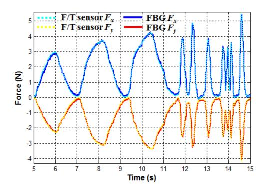
Figure A.13: Comparision of the force measurements from the force/torque sensor (dot) and the sensorized instrument (solid).
