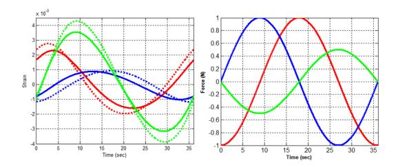
Figure 7.2: (a) The dashed lines are the strain values calculated from the previous model in subsection 7.2.2; the solid lines are from the new model; (b) the time-varing force that applied at the tip of the robot.
