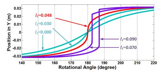
Figure 5.4: Tip position (in Y direction) of a three-tube robot with straight parts. Note that a large number of different  $l_1$  were tested in the program, only a few of them were plotted here.
