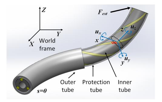
Figure 7.14: Demonstration of the design concept of a sensorized concentric-tube robot.
