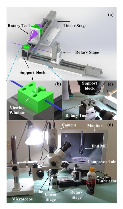
Figure 7.4: (a) The CAD model of the engraving system. (b) A magnified view of the support block. (c) The 3D-printed support block. (d) The actual customized engraving system.
