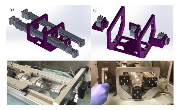
Figure 2.4: (a) The CAD design of the CTR drive unit for teleoperated operations. The components in grey are commercial products and the ones in purple are custom designed parts. (b) The CAD model except for the linear stages (c, d) Side view and front view of the actual 6 DOF robotic setup controlled by a haptic device (Touch X, Geomagic, United States).
