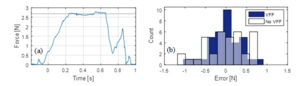
Figure A.8: Illustration of the definition of the mean peak force, representing the applied tension to the suture. (b) Histogram of the force error measured from a group of six subjects performing one-handed suturing tasks with and without VFF.
