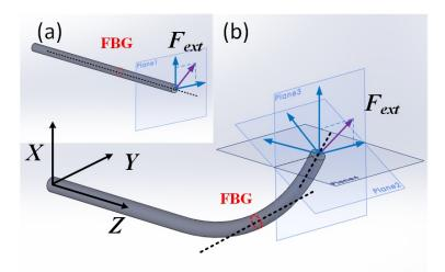
Figure 7.23: Lateral and axial forces for straight robotic tools (a) and pre-curved robotic tools (b).
