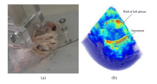
Figure 1.9: Continuum robot inserted inside a porcine heart. (a) Experimental set up; (b) 3D ultrasound image showing both the left atrium and the curved robot [39] (© 2012 IEEE).
