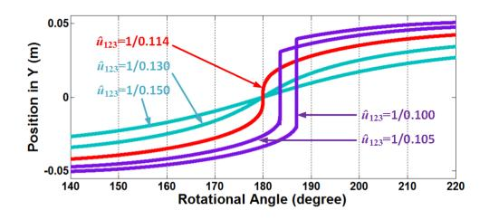
Figure 5.3: Tip position (in Y direction) of a three-tube robot without straight parts. Note that a large number of different  $\hat{u}_{123}$  were tested in program, only a few of them were plotted here.
