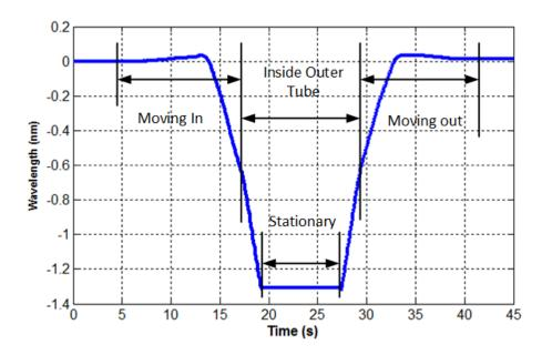
Figure 7.18: The wavelength output when the inner tube translates relative to the outer tube (biased at the beginning).
