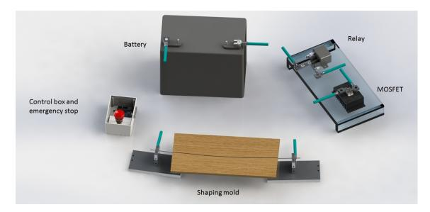
Figure 8.1: Conceptual design of an electric tube shaping setup.
