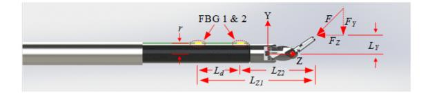
Figure A.2: A side view of the sensorized da Vinci Instrument.
