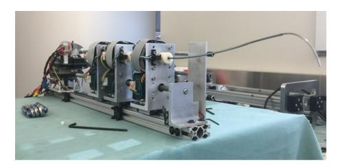
Figure 2.7: Assembly of the third prototype of CTR drive unit (except for the outer case)
