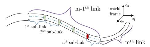
Figure 4.2: Links and sub-links of a concentric-tube robot.
