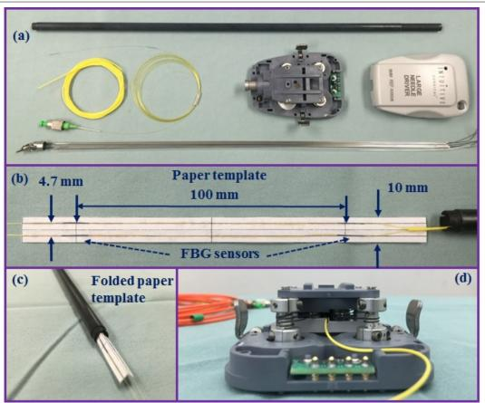
Figure A.11: (a) Disassembled da Vinci instrument; (b) paper template; (c) folded paper template (d) rear view of the sensorized instrument after reassembly.
