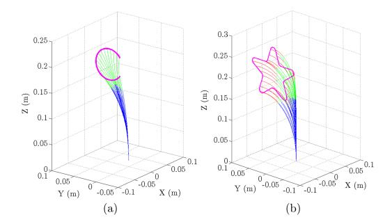
Figure 4.5: Trajectory tracking using (a) two-tube (blue:outer tube, green: inner tube) (b) three-tube concentric-tube robots (blue:outer tube, green: middle tube, red: inner tube).
