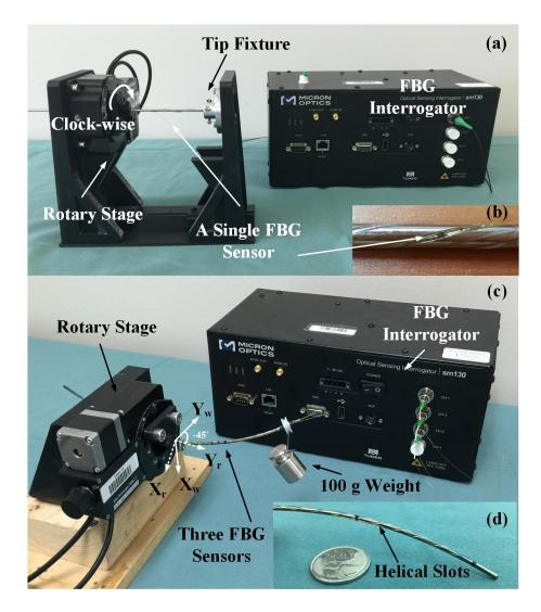
Figure 7.5: (a) Experimental setup for straight-tube torsion validation. (b) Magnified view of fiber embedded in grooved tube. (c) Experimental setup for pre-curved tube analyses. The robot base denoted  $(X_r, Y_r)$ , and is rotated  $-45^\circ$  with respect to the world frame  $(X_w, Y_w)$ . (d) Magnified view of the pre-curved tube with helical grooves.
