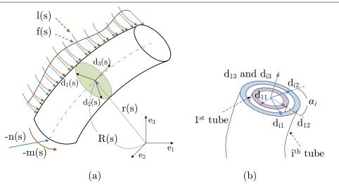
Figure 4.1: (a) Cosserat beam (b) cross section of a concentric-tube robot showing coordinate frames associated with the  $1^{st}$  and the  $i^{th}$  tubes.
