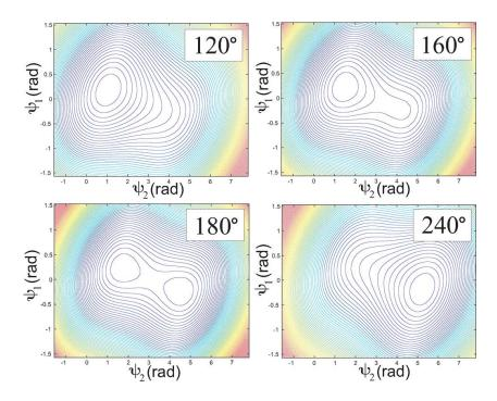
Figure 1.8: Contour plots of the energy landscape as the angular difference between the tube bases is increased. Angular difference between the base inputs of the two tubes is listed in the upper right corner of each plot. For small angular differences, there is only one global minimum. As the angular difference approaches  $180^\circ$ , two appear. Beyond  $180^\circ$ , the new minimum becomes the global minimum, and eventually the only minimum [2] (© 2009 IEEE).
