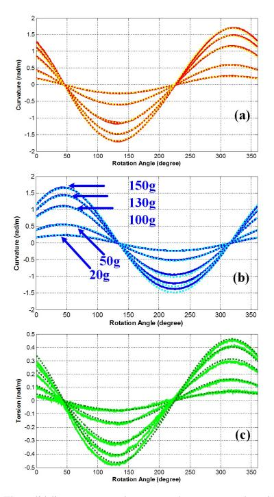
Figure 7.9: The solid lines represent the measured curvature and torsion values using helically-wrapped FBG sensors. The dashed lines are the theoretical values calculated from the model described in subsection 7.2.4. (a) plots the measured and theoretical values of  $(u_x - \hat{u}_x)$  under a series of loading; (b) and (c) display  $(u_y - \hat{u}_y)$  and  $(u_z - \hat{u}_z)$ , respectively.
