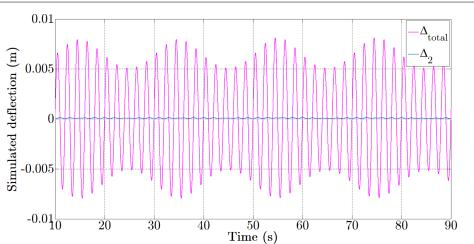
Figure 6.4: Simulation of the tip deflection: comparison between the total deflection and the Jacobian-related component.
