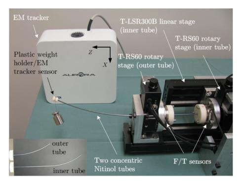
Figure 6.5: A view of our concentric-tube robotic system.
