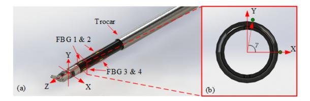
Figure A.1: (a) A 3D view of the sensorized da Vinci instrument (b) A cross-sectional view of the sensorized tool with two FBG sensors located with an angular difference of  $\gamma$ .
