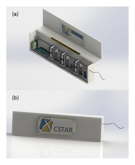
Figure 2.6: CAD design of a low-cost and compact CTR drive unit. (a) View of the main components of the proposed drive unit. (b) View of the overall robot.
