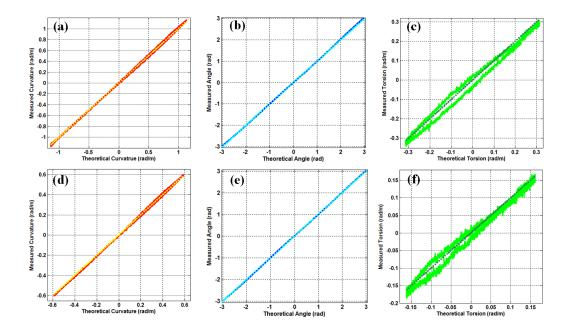
Figure 7.10: Demonstration of the accuracy and repeatability in bending curvature and torsion measurement. A weight of 100 g was used at the distal tip of the pre-curved Nitinol tube for (a), (b) and (c). A weight of 50 g was used for (d), (e), and (f). The red, blue, and green solid lines are the measurements of  $u_x$ ,  $\alpha_b^1$ , and  $\tau$ , divided by the theoretical value. A ratio of 1 between the measured and theoretical value is denoted by a dashed line.
