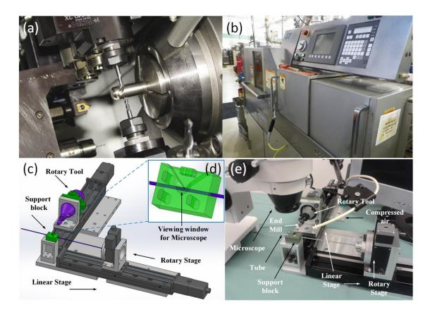
Figure 2.2: (a) A commercially available Swiss-type CNC lathe, Citizen-Cincom K16 (Marubeni Citizen-Cincom Inc., United States). (b) A view of the machine's full size. (c, d) The CAD design of our desktop micro-engraver (e) The actual setup of the developed desktop micro-engraver. The machining process can be monitored using a microscope through the viewing window on the support block.
