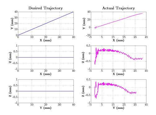
Figure 4.8: Desired and experimental trajectories in XY, XZ, and YZ planes (linear trajectory, final tip position =  $[41.59 \ 37.51 \ -0.31]^T$  mm).
