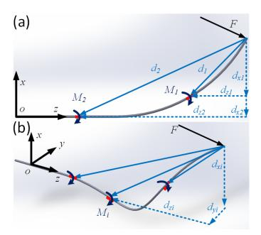
Figure 7.26: Pre-curved continuum robots with multiple sensorized cross-sections for 2D or 3D force sensing. The red marks represent the sensorized cross-sections.
