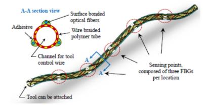
Figure 1.10: Schematic of wire braided polymer tube with surface mounted optical fibers [44] (© 2014 IEEE).
