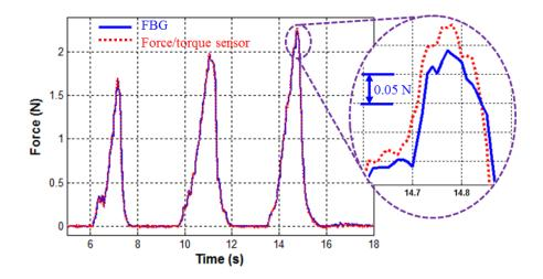
Figure 7.20: Comparision of the force values measured using Nano17 (red) and the sensorized CTR (blue).
