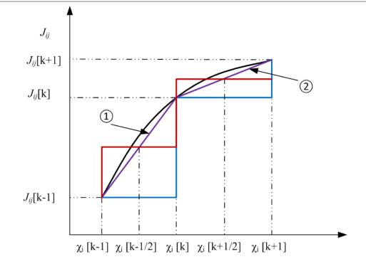
Figure 4.3: Function approximation using a multi-step approach.
