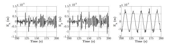
Figure 6.10: Tip tracking error using the proposed dual-layer control approach.
