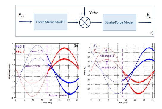
Figure 7.22: Demonstration of the performances of the two proposed strain-force calculation methods with and without added noise. (a) The signal flow of the simulations. (b) The strain values of the FBG sensors when the robot is under load. (c) Force measurements using these strain-force calculation methods developed.
