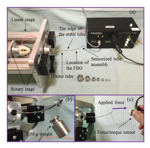
Figure 7.17: (a) The experimental setup for force sensing calibration and validation; (b) vertical loading senario; (c) horizontal loading scenario.
