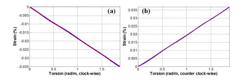
Figure 7.6: The torsion measurements (blue) when the motorized stage rotates in a clockwise direction (a) and a counter-clockwise direction (b). The red lines are the linear best-fit to the measurement data.
