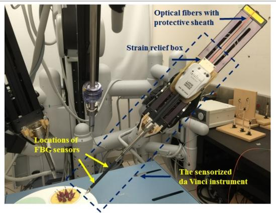
Figure A.10: Sensorized instrument mounted on a da Vinci robot
