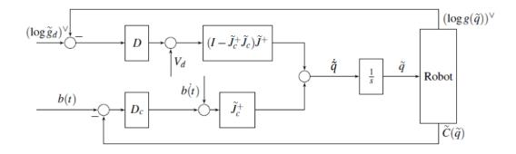
Figure 1.12: The control block diagram of the closed-loop system. The inequality constraints on the joint space variables  $C(q) \leq b$  are converted into equal constrains  $\tilde{C}(\tilde{q}) = b$ , then applied to the inverse kinematic control algorithm. D and  $D_c$  are positive definite diagonal matrices,  $\tilde{J}_c$  is the augmented constraints Jacobian matrix and  $(\log g)^{\vee}$  returns the 6D vector representation of g [51] (© 2014 IEEE).
