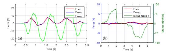
Figure A.6: Demonstration of the performance of the two cross-section FBG sensing under different loading disturbances. (a)  $F_X$  values measured from FBG and Nano17 sensors under a varying axial loading (b)  $F_X$  values measured from FBG and Nano17 sensors under varying force coupling about the Y axis.
