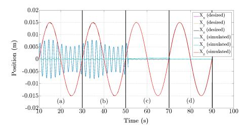
Figure 6.3: Simulation of the tip position  $X = [X_x \ X_y \ X_z]^T$  tracking using four control strategies: (a) unloaded Jacobian, (b) loaded Jacobian J, (c) loaded Jacobian J plus  $\dot{\Delta}_{total}$ , and (d) the dual-layer approach.
