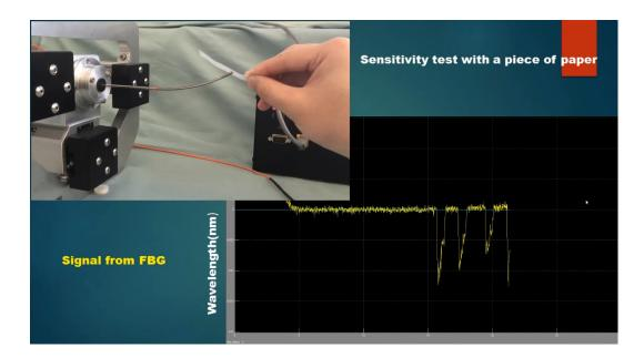
Figure 7.16: Illustration of the sensitivity of the sensorized CTR in force sensing
