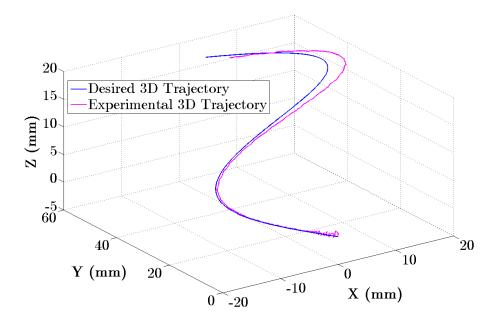
Figure 4.10: Desired and experimental trajectories in 3D (final tip position =  $[2.329 \ 47.79 \ 19.65]^T$  mm, final desired position =  $[0 \ 50 \ 20]^T$  mm).
