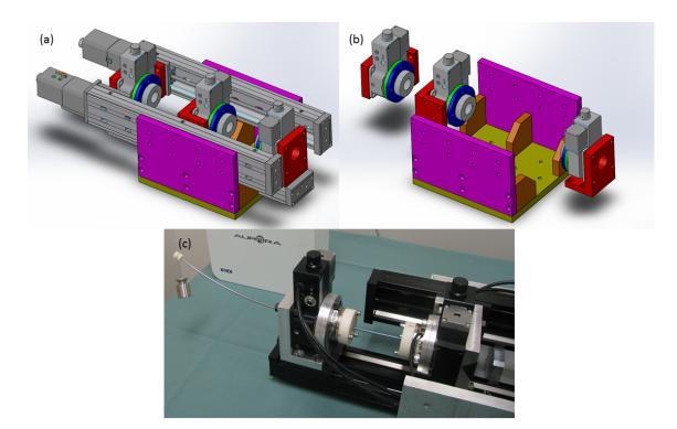
Figure 2.3: (a, b) The CAD design of a 6DOF CTR drive unit using high precision linear and rotary stages. The parts in grey are commercial products and the rest of the parts are custom built. (c) The actual robotic setup using two linear and two rotary stages.
