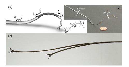
Figure 1.1: (a) Demonstration of the concept of a CTR [1] ( $\bigcirc$  2010 IEEE). (b) A 3-tube CTR [2] ( $\bigcirc$  2009 IEEE). (c) A CTR with an micro-grasper attached at the tip [5]( $\bigcirc$  2012 IEEE).
