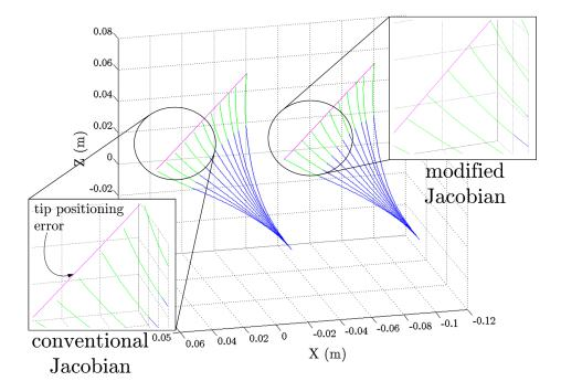
Figure 4.6: Trajectory tracking using conventional Jacobian and modified multi-step Jacobian approach in the two-tube robot.
