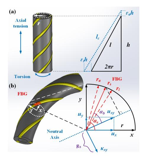
Figure 7.1: Demonstration of the curvature-strain model for helical-wrapped FBG sensors.  $\kappa_{xy}$  is the curvature vector commonly used for representing the bending radius and the direction of bending.  $u_{xy}$  is the curvature vector used for deriving the curvature-strain model presented in this work. Note that  $||u_{xy}|| = ||\kappa_{xy}|| = R_b$ .
