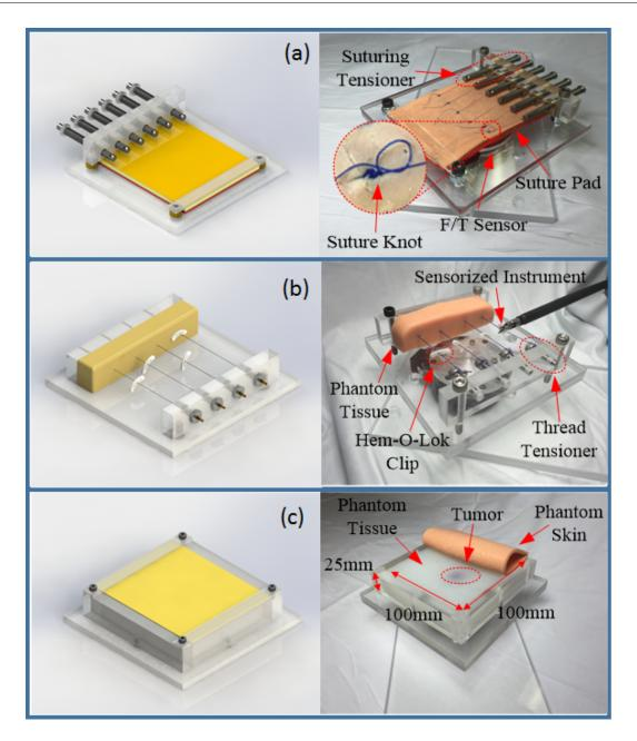
Figure A.7: Demonstration of custom made testbeds for three surgical tasks. (a) Onehanded suture knot tightening testbed (b) Hem-O-Lok tightening testbed (c) Tumor localization by palpation testbed.
