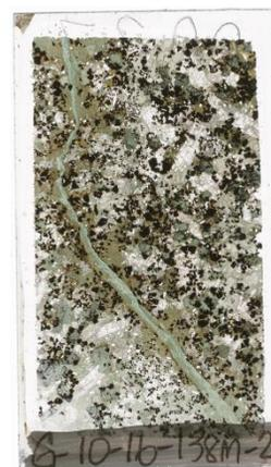
Cumulate fine grained magnetite, section is cross-cut by a carbonate-chl vein.
