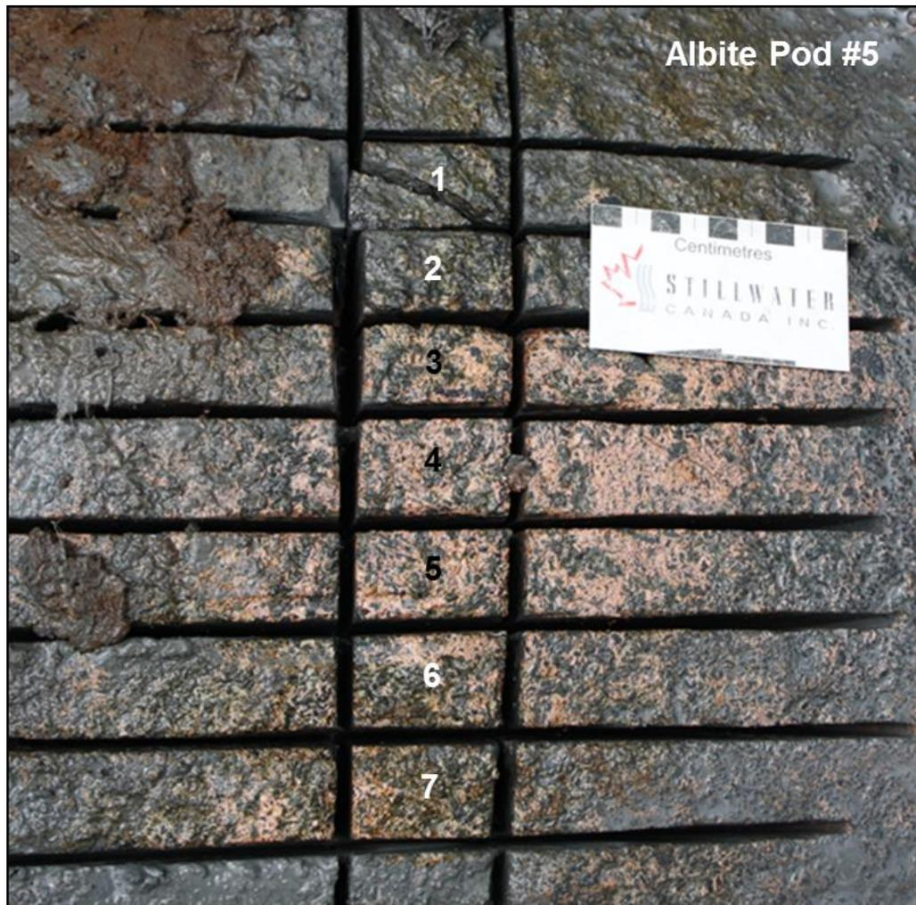
**Figure 3.4** – Transect of Albite Pod #5, also showing the cuts that were made. Blocks 1 and 2 contain little to no surface albitization, while block 7 is moderately albitized on surface. Blocks 3, 4, 5, and 6 are pervasively albitized on surface.
