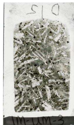
Plagioclase laths weakly aligned perpendicular to the core length, plagioclase grains on average  $\sim <1.5$ cm, interstitial clinopyroxene and no olivine. Magnetite is subhedral forming rounded clusters of  $\sim 0.5$ cm.
