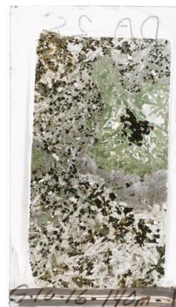
Plagioclase laths weakly aligned perpendicular to the core length, plagioclase grains on average  $\sim <1.5\text{cm}$ , interstitial clinopyroxene and very little to no olivine. Magnetite is subhedral forming rounded clusters of  $\sim 0.5\text{cm}$ .
