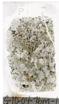
Consists primarily of euhedral plagioclase with interstitial clinopyroxene. Section is x-cut by a carbonate fracture.
