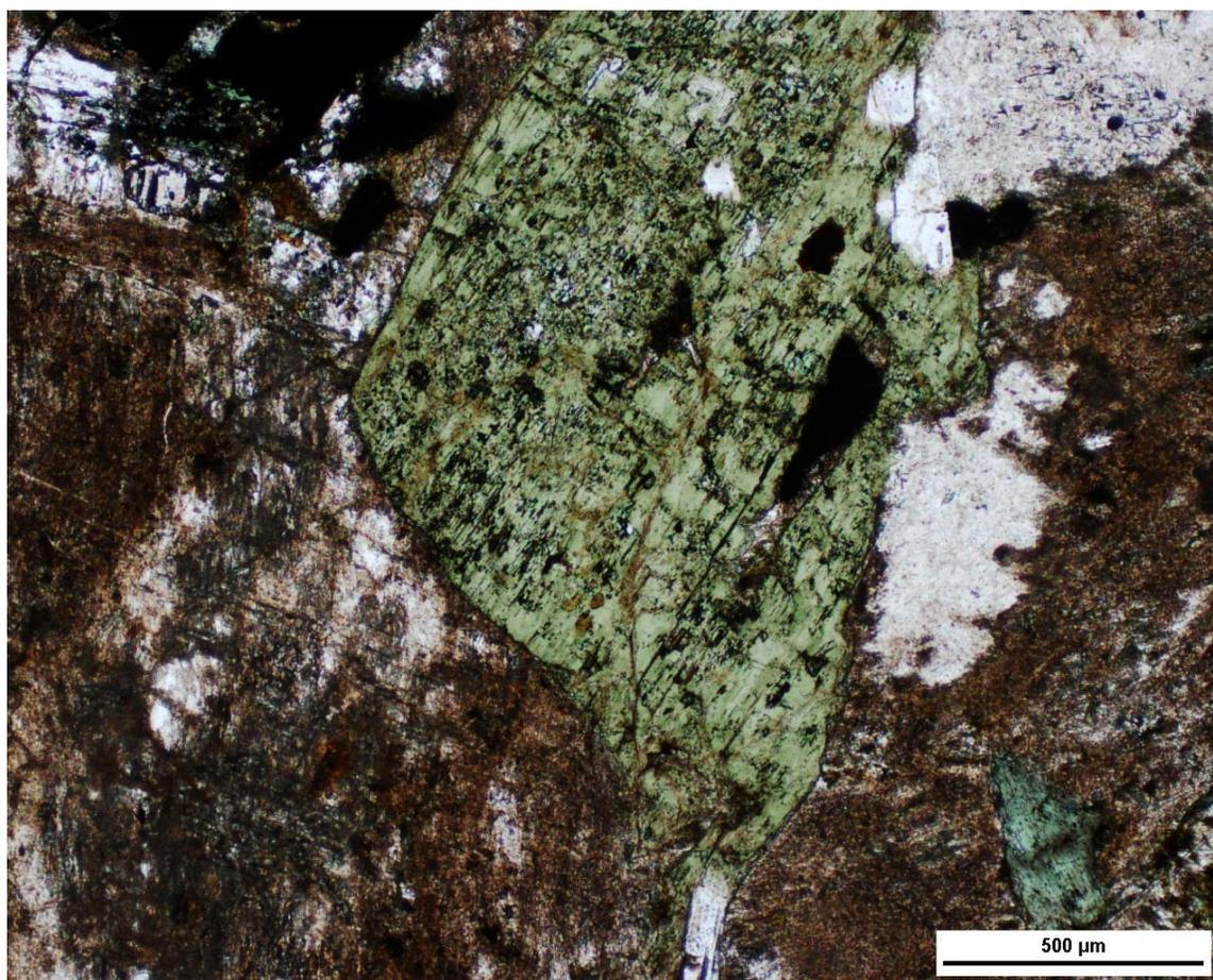
General texture of alteration in this sample. Middle grain (light green) is a serpentinized olivine grain, and it is enveloped by albite. An actinolite grain (forest green) is also contained by albite alteration.
