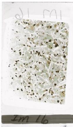
Plagioclase laths weakly aligned perpendicular to the core length, plagioclase grains on average  $\sim <1.5\text{mm}$ , with interstitial clinopyroxene. Magnetite is subhedral forming rounded clusters of  $\sim 0.5\text{cm}$ .
