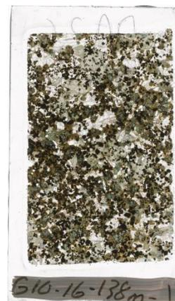
Sample contains abundant fine-grained magnetite and sugary-white apatite. Some sections of the sample contain higher proportions of clinopyroxene and plagioclase.
