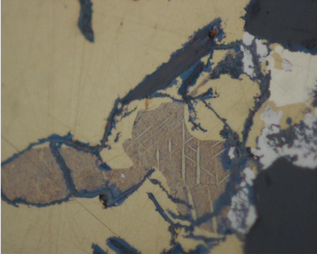
A close up of the image above, showing bornite (brownish-purple) within a chalcopyrite grain. The fractures of the chalcopyrite grain contain covellite (blue). In reflected light. The white coloured grains are pentlandite (grey-white), and galena (bright white).
