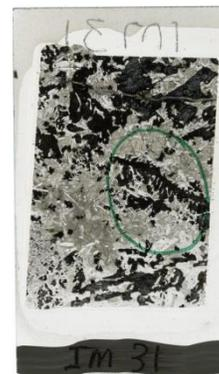
Medium to mainly coarse grained dark grey to black skeletal olivine grains with interstitial frosty white plagioclase inter-grown with minor light grey clinopyroxene. Appears to have very minor actinolite (green) alteration. Very trace disseminated chalcopyrite is visible in the slightly greener (actinolite altered) patches of plagioclase.
