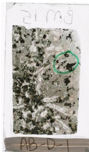
There is some very fine disseminated chalcopyrite visible. Blue-grey plagioclase laths comprise most of the sample with interstitial black clinopyroxene or magnetite. Apatite is also common, resulting in a fairly sugary texture.
