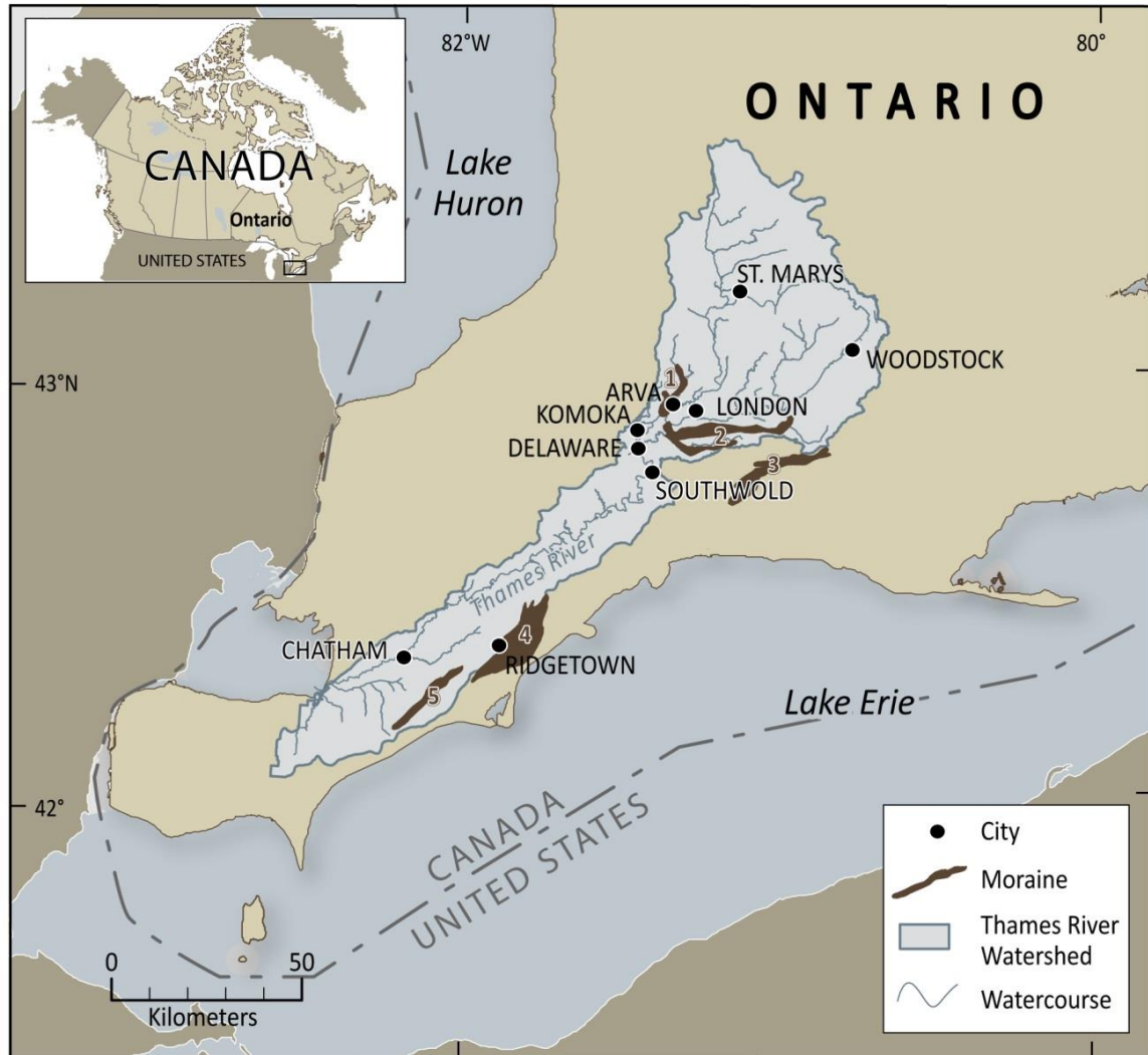
Figure 1. Location of Thames River watershed, major cities and locations mentioned in text. Major moraines within the watershed are indicated: 1. Arva Moraine, 2. Ingersoll Moraine and adjoining Westminister Moraine to the south, 3. St. Thomas Moraine, 4. Blenheim Moraine and 5. Charing Cross Moraine. Adapted from Chapman and Putnam (1984) and Goff and Brown (1981).
