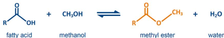
**Figure 4-1** Esterification reaction to produce biodiesel (Johnson, 2016)
