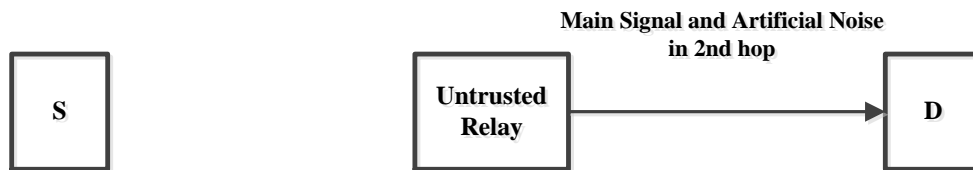
Figure 2.9: Second hop of secure communication with untrusted relay via using cooperative jamming.
