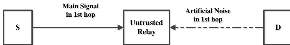
Figure 2.8: First hop of secure communication with untrusted relay via using cooperative jamming.
