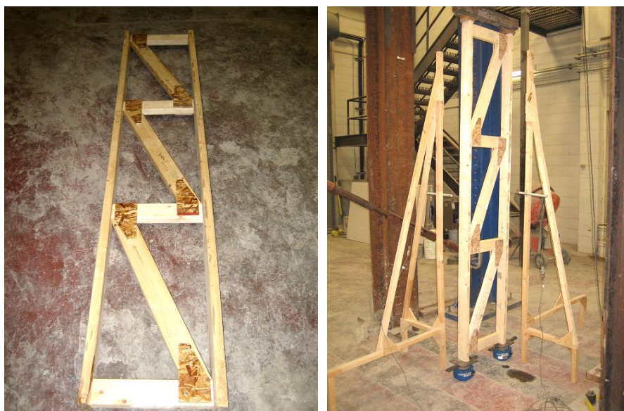
(a) Braced pair of studs
