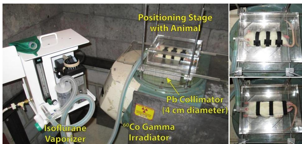
**Figure 2-3:** Photograph of  $^{60}\text{Co}$  irradiator with animal positioning system and isoflurane vaporizer (left). Positioning system seen from top view showing custom-built animal positioning stage and lead collimator with rat in prone (top-right) and supine (bottom-right) positions.
