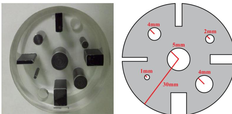
**Figure 2-1:** Photograph of the acrylic resolution phantom (left) and a corresponding schematic diagram with shown dimensions. The  $^{129}\text{Xe}$  gas resides in the empty space of the phantom container.
