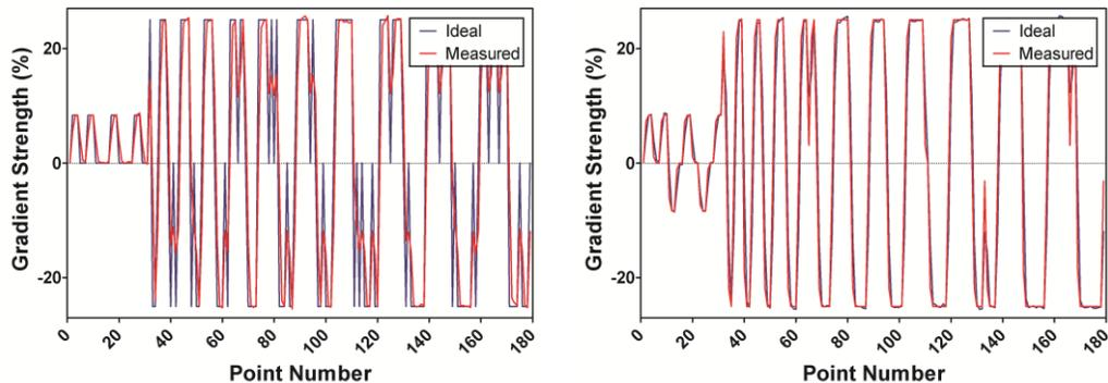
**Figure A-7:** Representative input (blue) and measured (red) *Sectoral* trajectories through  $k$ -space, or frequency-encoding waveform, for the  $x$ -axis gradient of the 11<sup>th</sup> sector (left) and the  $y$ -axis gradient of the 12<sup>th</sup> sector (right).
