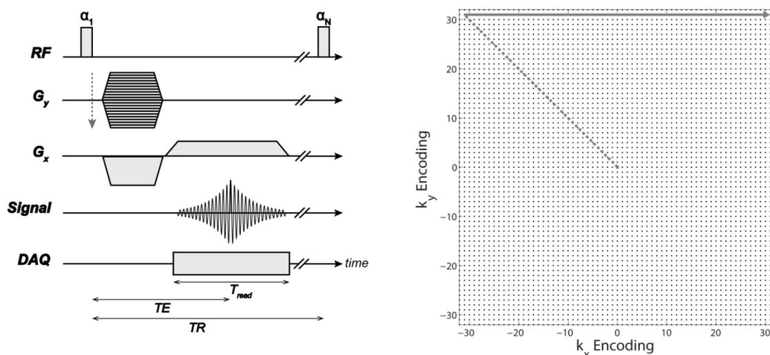
**Figure 1-9:** A pulse sequence diagram (left) and  $k$ -space trajectory (right) for the example of a FGRE Cartesian  $k$ -space acquisition.
