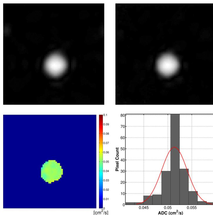
**Figure 3-3:** Representative diffusion-weighted MB-*Sectoral* <sup>129</sup>Xe phantom results filled with pure <sup>129</sup>Xe. Shown are: un-weighted image (top-left), diffusion-weighted image (top-right), corresponding ADC-map (bottom-left) and histogram (bottom-right). *Mean* ADC =  $0.051 \pm 0.003$  cm<sup>2</sup>/s and FWHM ADC =  $0.008$  cm<sup>2</sup>/s.
