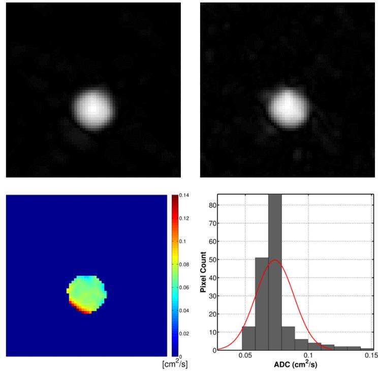
**Figure 3-4:** Representative diffusion-weighted MB-Sectoral  $^{129}\text{Xe}$  phantom results with 6.4 ml of  $\text{N}_2$  added. Shown are: un-weighted image (top-left), diffusion-weighted image (top-right), corresponding ADC-map (bottom-left) and histogram (bottom-right). *Mean* ADC =  $0.073 \pm 0.015 \text{ cm}^2/\text{s}$  and *FWHM* ADC =  $0.037 \text{ cm}^2/\text{s}$ .
