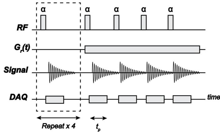
**Figure A-2:** Pulse sequence diagram for the MFGM acquisition to measure the gradient waveform. Small tip angle RF pulses were applied to produce a FID from the phantom. A series of points for each acquisition during phase-encoding time  $t_p$  were sampled.
