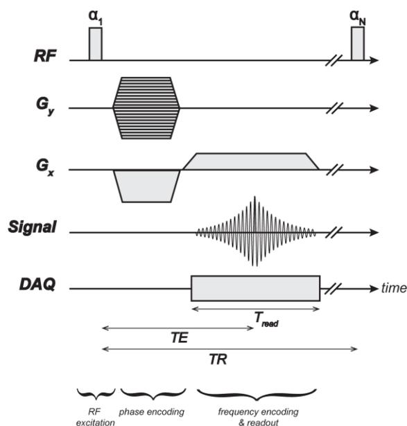
**Figure 1-5:** An example of an MRI pulse sequence diagram. The vertical axis is the amplitude and the horizontal axis is time. A pair of frequency and phase encode gradients are shown prior to the echo of the MRI signal. A readout gradient on  $G_x$  is switched on when the echo signal appears and the signal is digitized during data acquisition (DAQ).
