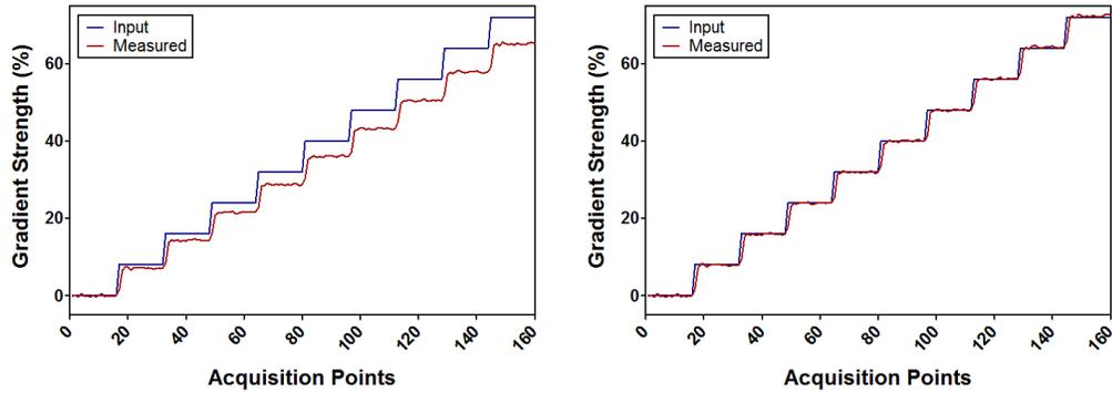
**Figure A-6:** Measured gradient waveforms without (left) and with (right) coefficient correction. The prescribed input waveform (blue) was stepwise with each gradient step corresponding to 24 points (24  $\mu$ s) and measured waveform (red) experienced within the sample space.
