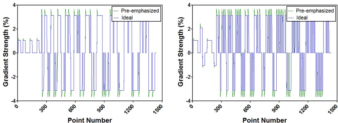
**Figure A-3:** Pre-emphasized (green) and ideal (blue) trajectories through  $k$ -space, or frequency-encoding waveform, for the  $x$ -axis (left) and  $y$ -axis (right) gradient of the 11<sup>th</sup> sector.
