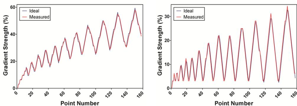
**Figure A-8:** Representative ideal (blue) and measured (red) *Sectoral* trajectories through  $k$ -space, or pure phase-encoding waveform, for the  $x$ -axis gradient of the 11<sup>th</sup> sector (left) and the  $y$ -axis gradient of the 12<sup>th</sup> sector (right).
