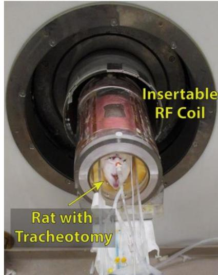
**Figure 2-7:** Insetable RF coil with tracheostomized rat.
