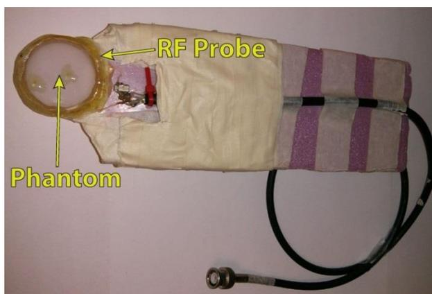
**Figure A-1:** A photograph of the probe head setup with phantom for gradient waveform mapping. The plastic circular phantom contained 2.0 ml of water and 1.0 ml of Magnevist and was placed within a small surface coil wound from Litz wire.
