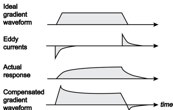
**Figure 1-8:** A schematic of gradient pulses. The eddy currents induce a magnetic field that adds to the ideal gradient waveform to form a manifested response. A compensated gradient waveform (i.e. pre-emphasis) reduces the effect of eddy currents in the desired waveform.
