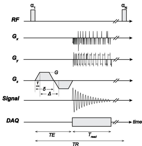
**Figure 1-12:** A diagram of the diffusion-weighted *Sectoral* pulse sequence including a bipolar trapezoidal gradient pulse with diffusion time,  $\Delta$ , lobe duration,  $\delta$ , ramp time,  $\tau$ , and gradient magnitude,  $G$ .
