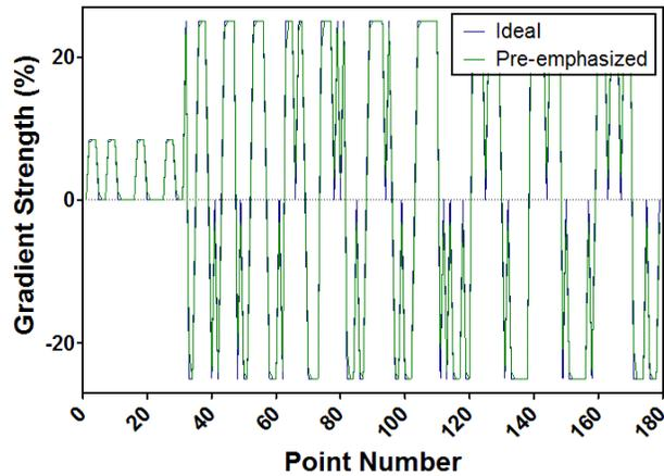
**Figure A-4:** Reduced pre-emphasized (green) and ideal (blue) trajectories through  $k$ -space, or frequency-encoding waveform, for the  $x$ -axis gradient of the 11<sup>th</sup> sector.
