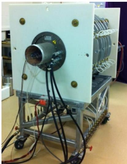
**Figure 2-5:** Low magnetic field (74 mT) MRI system.
