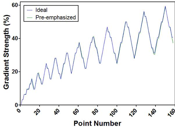
**Figure A-5:** Pre-emphasized (green) and ideal (blue) trajectories through  $k$ -space, or pure phase-encoding waveform, for the  $x$ -axis gradient of the 11<sup>th</sup> sector.
