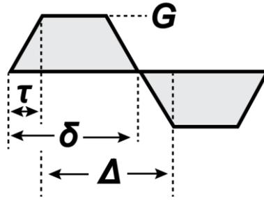
**Figure 1-7:** The diffusion bipolar trapezoidal gradient with amplitude  $G$ , ramp time  $\tau$ , lobe duration  $\delta$ , and diffusion time  $\Delta$ .
