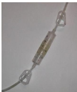
**Figure 2-2:** Photograph of the flow-through syringe phantom.
