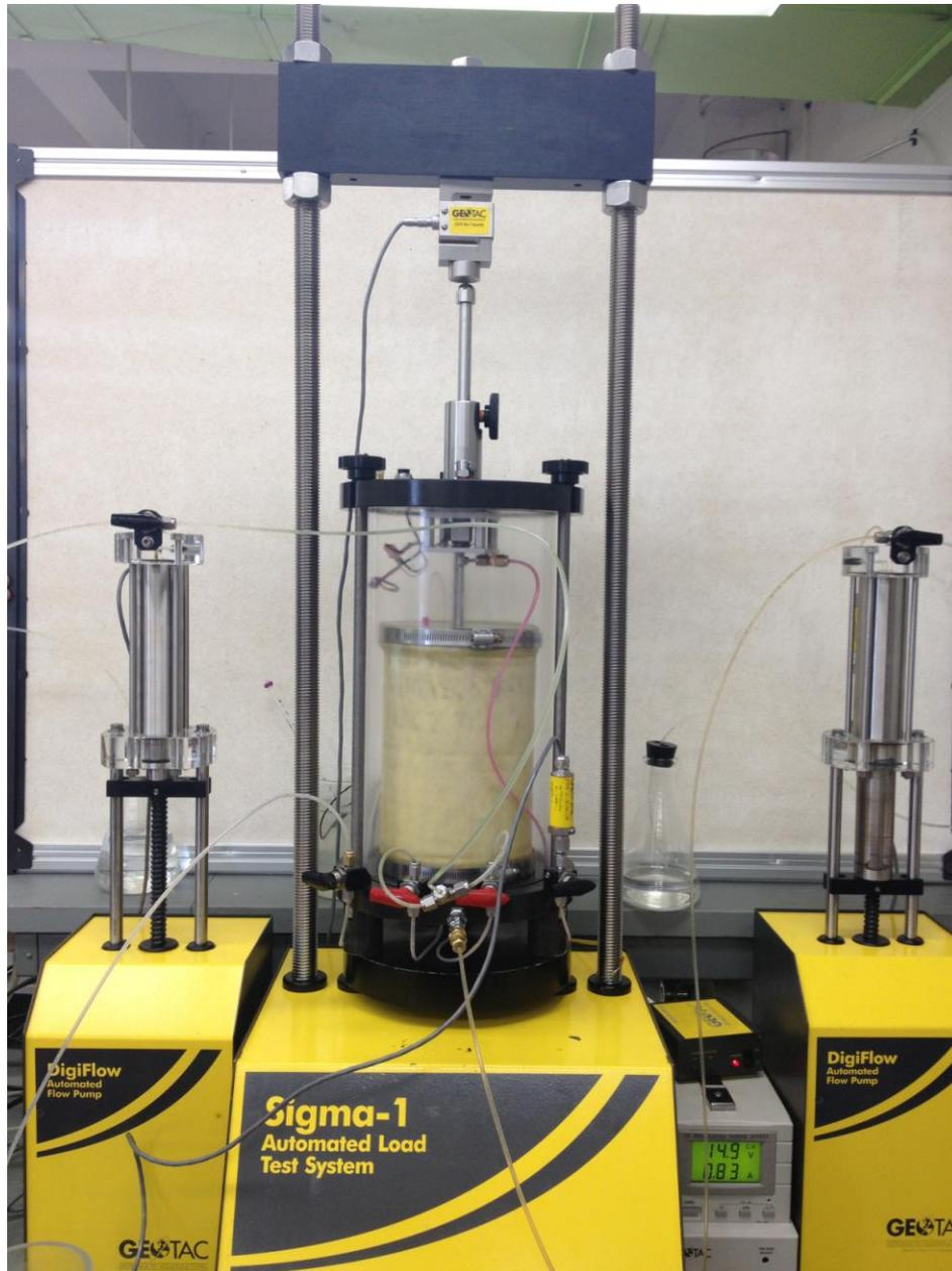
Figure B-2: Miniature cone calibration chamber assembly
