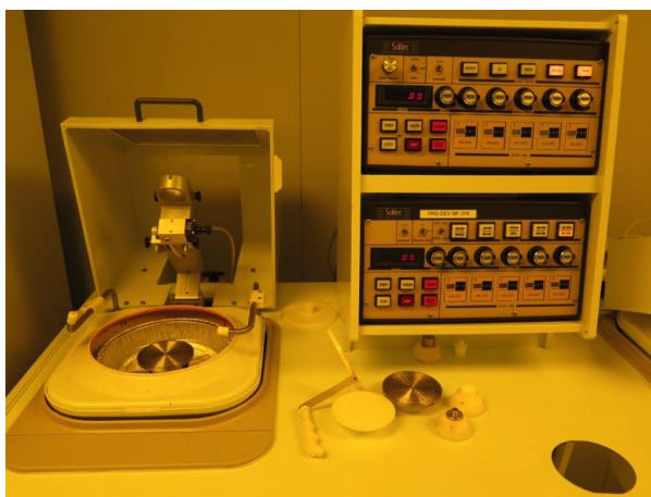
Figure 3-11 Solitec 5110 spinner in Western Nanofab
