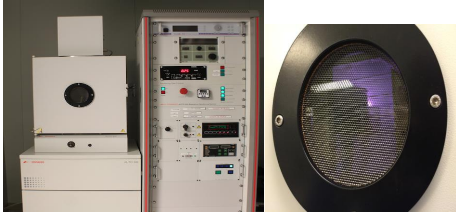
Figure 3-9 The Edwards Auto500 sputtering system in Western Nanofab
