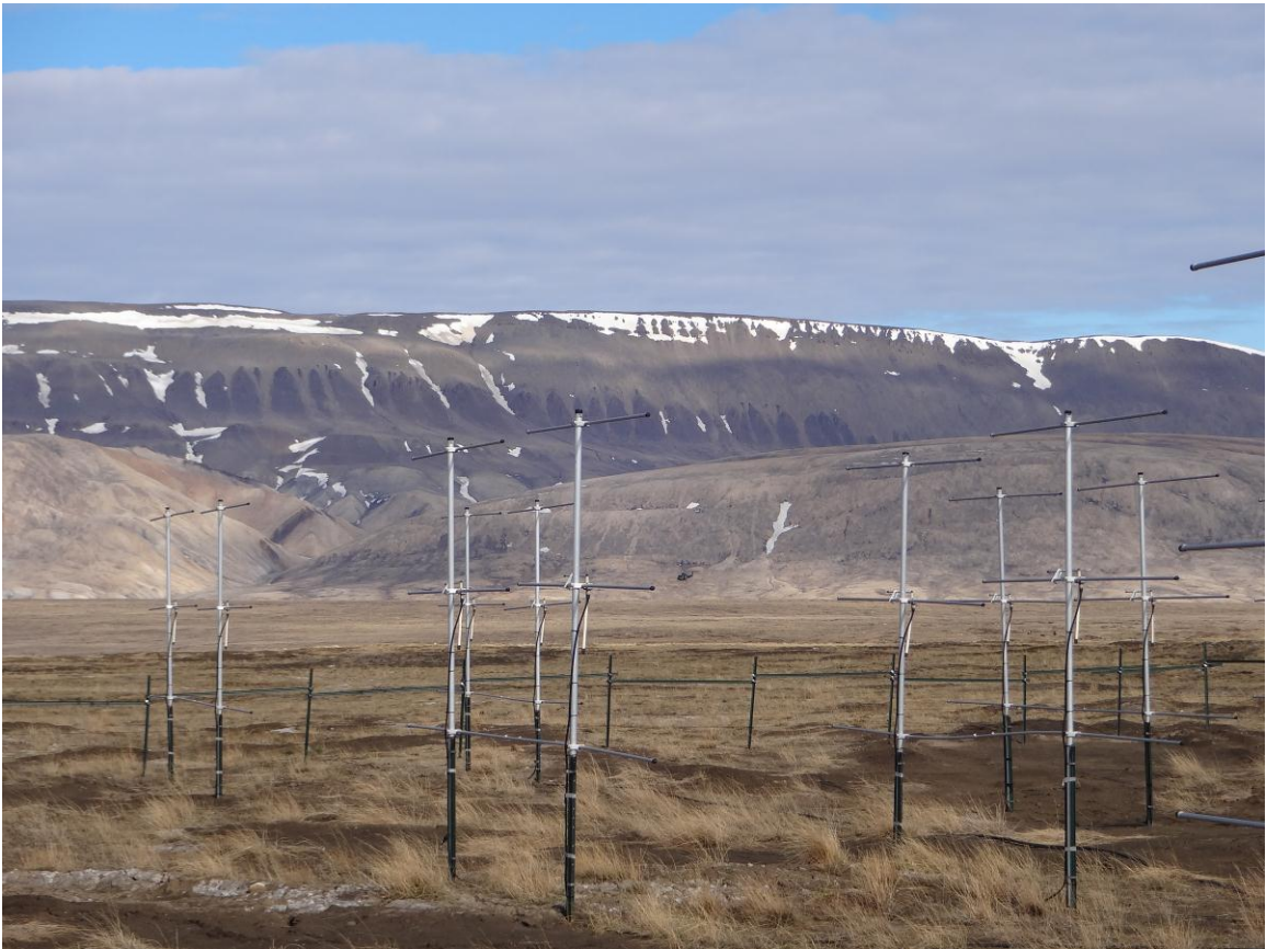
Figure 3.1: Yagi antennas. Part of the antenna array located at Eureka, NU.
