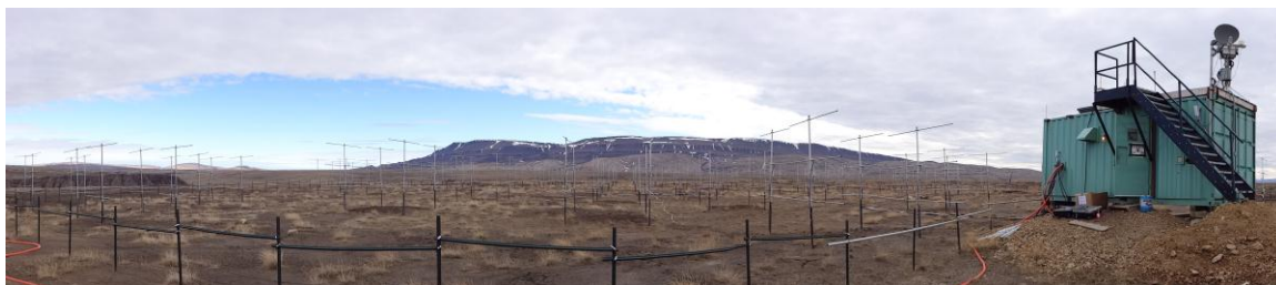
Figure 3.6: A panoramic view of the radar station at Eureka, NU with Blacktop mountain in the distance. The computer and transmitter are located inside the blue-green building to the right.
