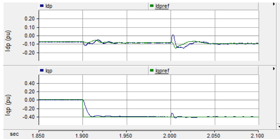
Figure 3.6 Positive sequence current (in dq frame) for different time constant ( T_{iq\_p} )
