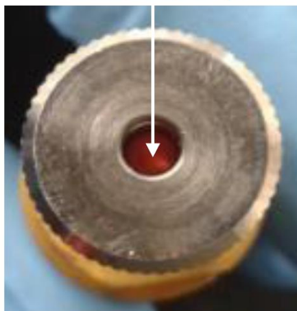
Figure 3.4: PTFE silicon septum placed over the stainless steel cell during sampling.
