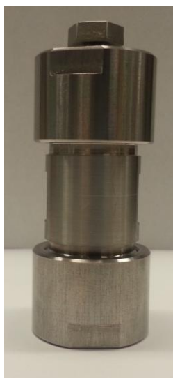
Figure 4.7: Stainless-steel radiolysis cell.
