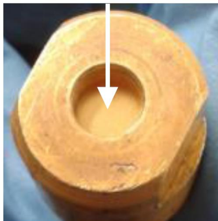
Figure 3.3: Gold-plated stainless steel cell cap showing gold foil in the center.
