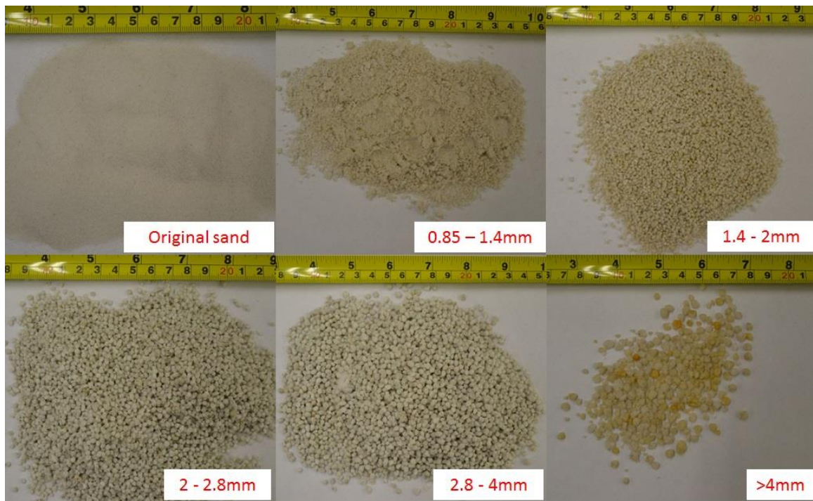
Figure 4-10: Agglomerates obtained in the BFB tests with 0.8 wt% KOH in the bed material at 3.9U_{mf}
