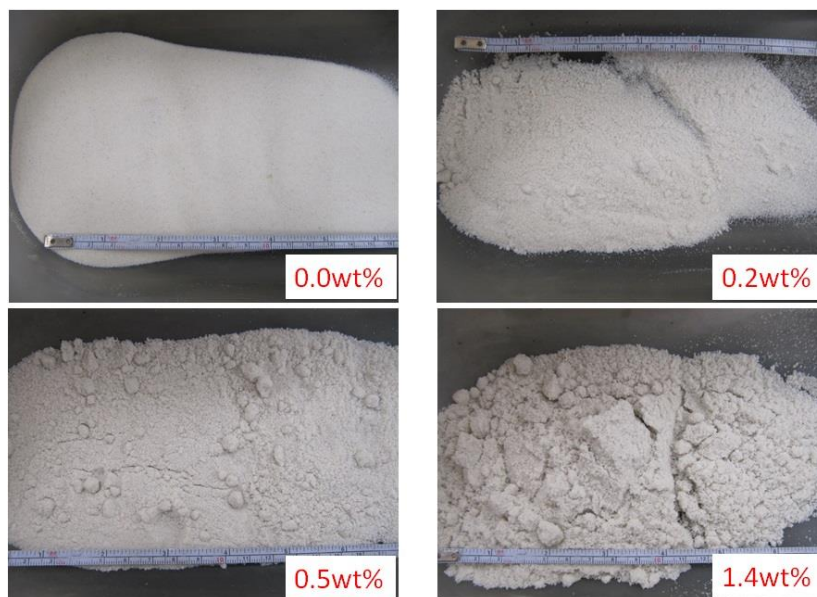
Figure 3-6: Samples of bed materials after fluidization at different glycerol-water (30% v/v) injection amounts
