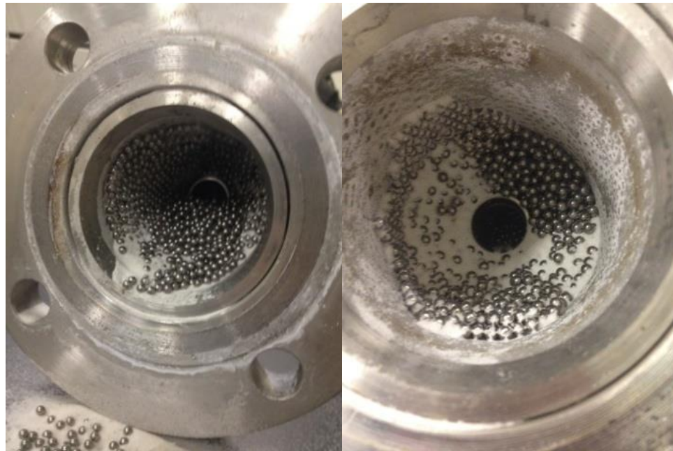
Figure A-6: Wind box blocked with bed materials particles (silica sand)
