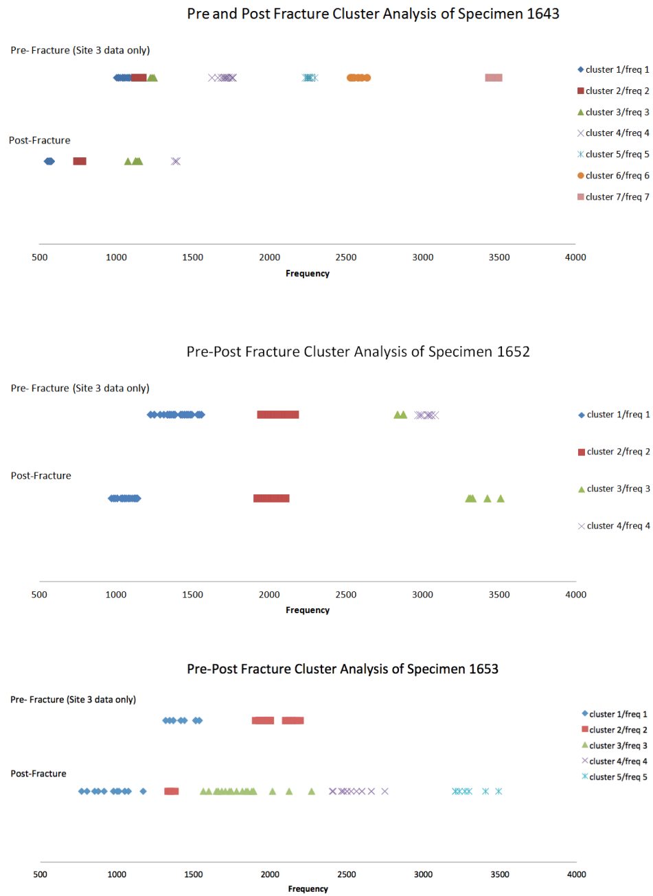
Figure 3.9: Pre and post cluster analysis results of specimens 1643, 1652 and 1653
