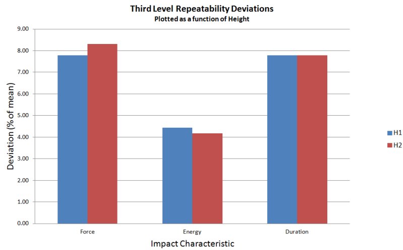
(b) Average impact deviation of the first and last three strikes of all sites and characteristics (impact force, impact energy and impact duration) per height
