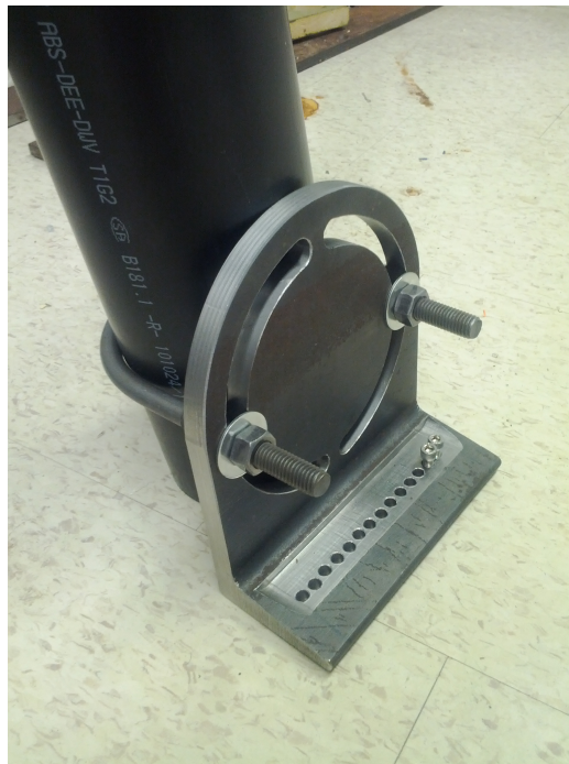
Figure 2.3: Custom bracket designed for specimen constraint
