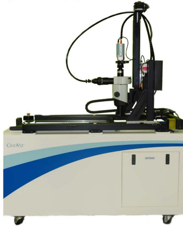
Figure 1.1: CryoViz™ cryo-imaging system used for sectioning and optical imaging of frozen mouse volumes
