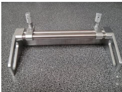
**Figure 3-3 Knife spreader (Mitutoyo, TQC Co.) used in this study to laminate MPLs and CLs. Height of the knife is adjustable to obtain different uniform thicknesses**
