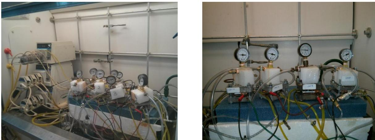
**Figure 3-6 BioGenerator fuel cells laboratory set-up**
