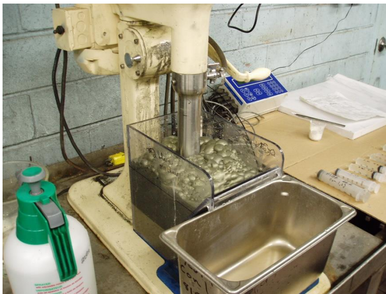
Figure 2-2 Example of the “Denver” flotation equipment used in the testing.
