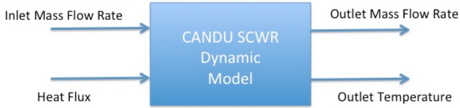
Figure 5.2: Dynamic model for the CANDU SCWR
