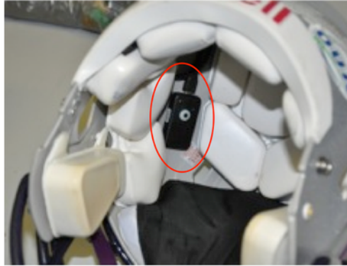
Figure 4.1: Illustration showing a GFT device, circled in red, mounted on the left side of the crown bladder inside a football helmet
