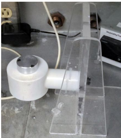
Figure 20: Collector electrode for unaligned fibers
