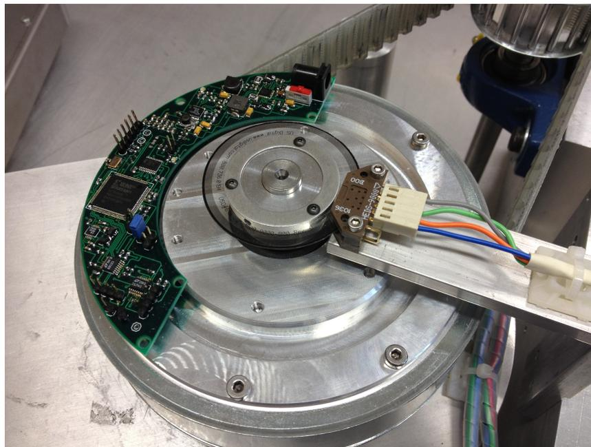
Figure 2.21: Embedded FPGA board inside MR clutches.
