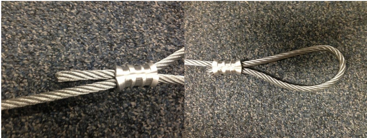
Figure G4a (LEFT) - An unfailed swaged cable connection . Figure G4b (RIGHT) - The swaged cable connection post failure
