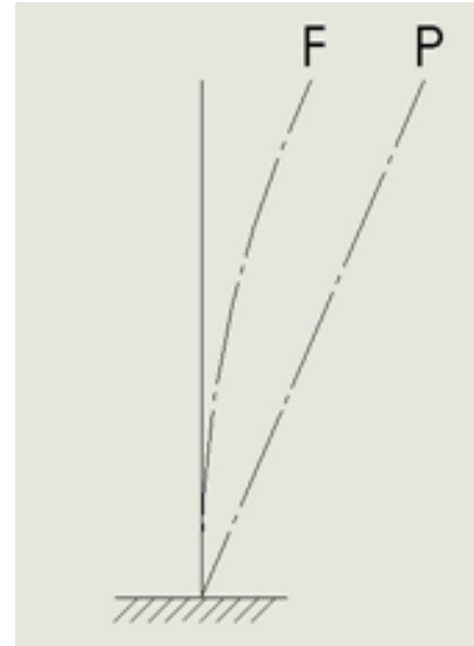
Figure 8.3 - Deflection difference due to fixity.
