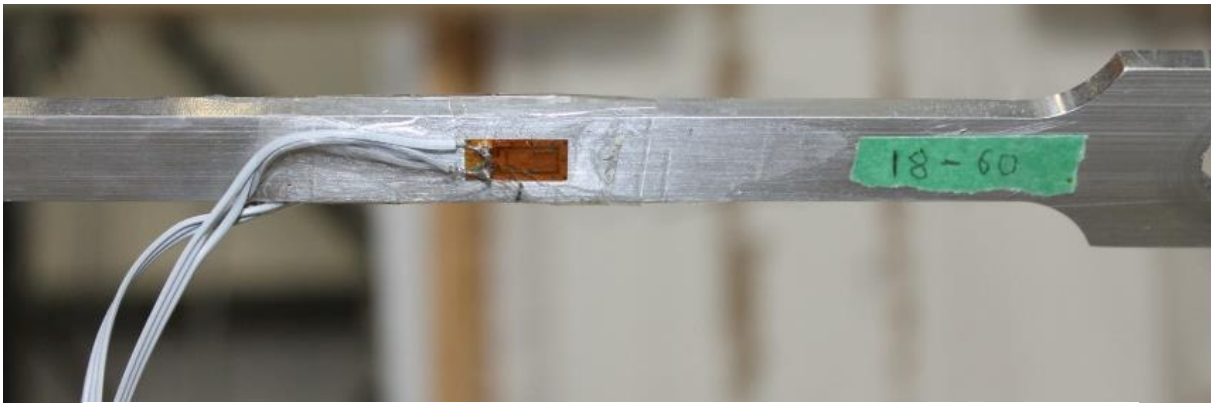
Figure A2 - Aluminum load cell with strain gage attached.
