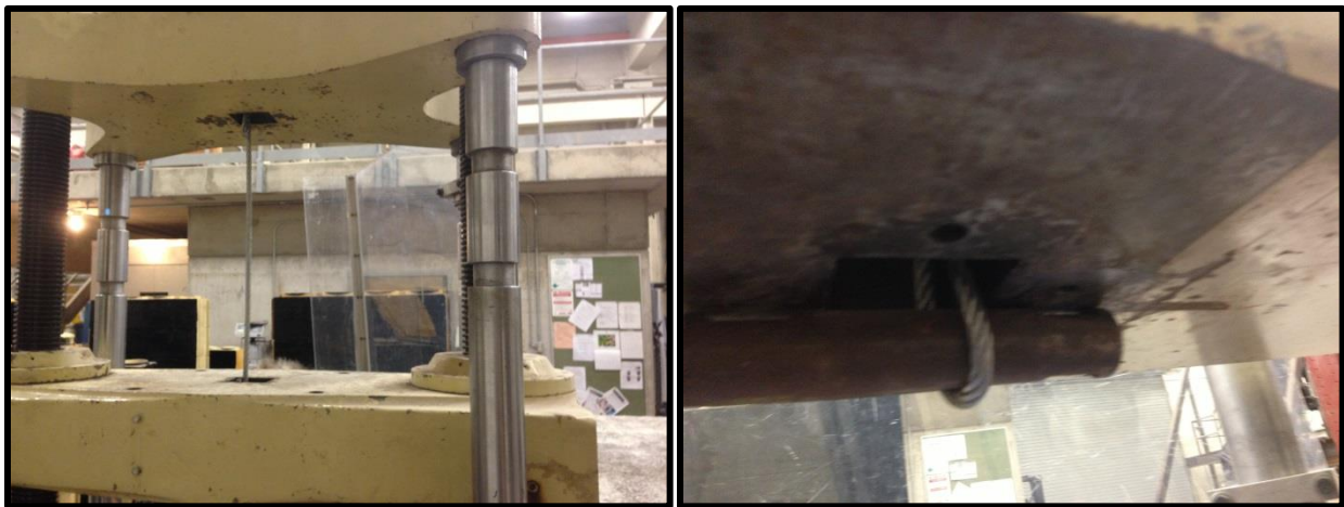
Figure G2 (LEFT) - The experimental setup. Figure G3 (RIGHT) - Bottom of experimental setup, showing how the loop was held in place
