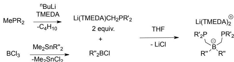
Scheme 1-1: General synthesis of the bis(phosphino)borate ligand class following the methodology developed by Jonas Peters and coworkers.
