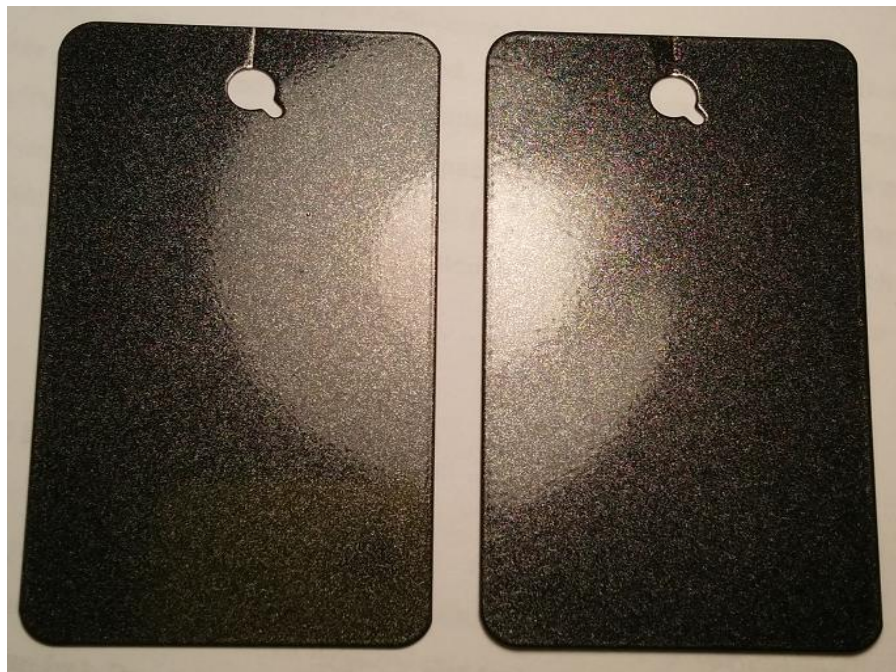
Figure 9-5: The coatings obtained from the new sample (left) and the control sample (right)
