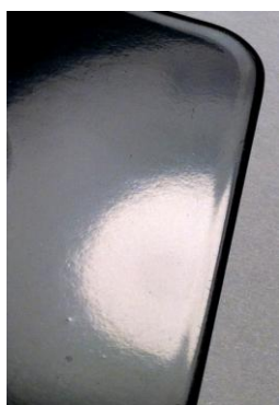
c. Coating surface with small roughness
