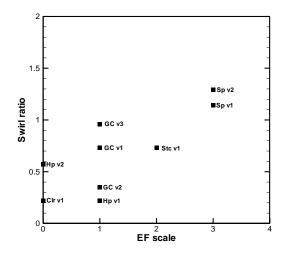
Figure 6-10: Potential relationship between swirl ratio and EF-Scale.
