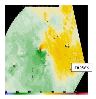
Figure 5-2: Doppler velocity (m/s) contour map of the Happy, TX 2007 tornado at 0203:20 UTC (Hp v2) and at 0.3° radar beam angle showing the tornado vortex location relative to the Doppler radar.
