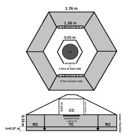
Figure 6-4: Schematic drawing of the MWD demonstrating TC, RC and CC zones.
