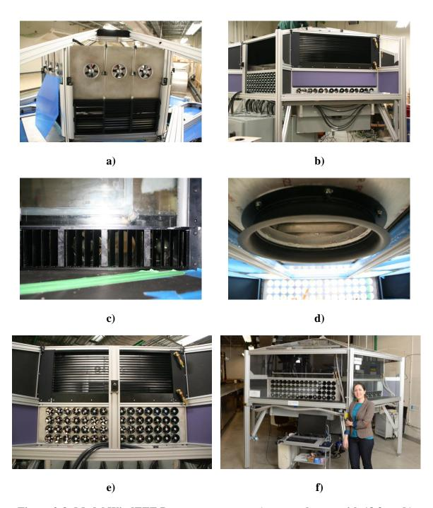
Figure 2-8: Model WindEEE Dome components: a) upper plenum with 18 fans, b) lower chamber with 100 fans, c) directional vanes at the periphery, d) bell-mouth, e) wall of 60 fans with heat exchangers on the top, f) relatively large scale of the simulator after completion.
