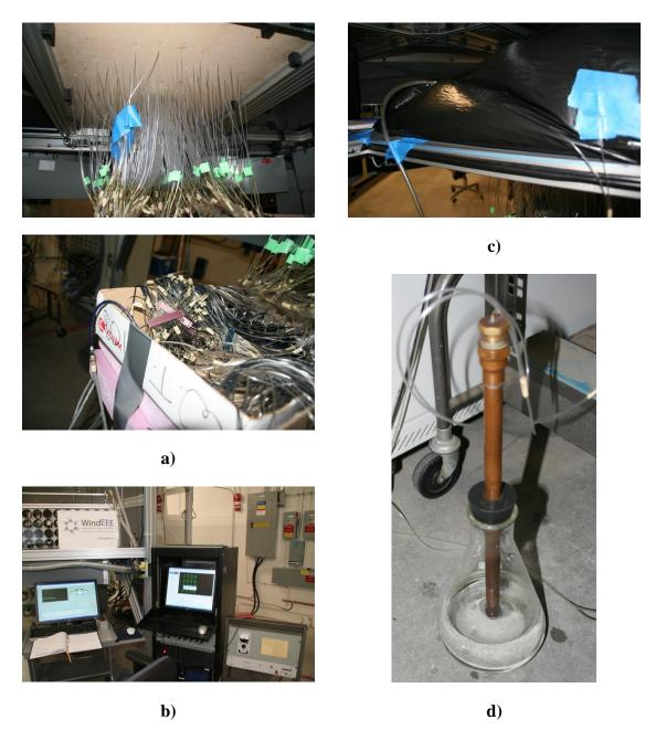
Figure 3-3: Static pressure test setup: a) pressure tubes and scanners arrangement, b) pressure bottle, c) pressure system, Barocel and simulator controllers and ) bag test.
