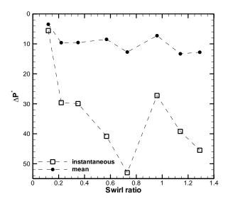
Figure 4-11: Time-dependent (square symbols) and time-averaged maximum surface pressure deficits as a function of swirl ratio for  $Re_r$ =6.7×10<sup>4</sup>.
