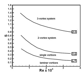
Figure 2-14: Critical (transition) swirl ratio as a function of radial Reynolds number; L-T → laminar to turbulent, 1-2 → Single-celled to two-celled vortices, 2-3 → two-celled vortices to three-celled vortices – image from [6].
