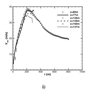
Figure 6-7: Comparison between simulated (lines) and full-scale (symbols) tangential velocity profiles at various heights for nine radar volumes after applying the velocity and length scales; a) Clr v1: S=0.22, b) Hp v2: S=0.57, c) Hp v1: S=0.22, d) GC v1: S=0.73, e) GC v2: S=0.35, f) GC v3: S=0.96, g) Stc v1: S=0.73, h) Sp v1: S=1.14 and i) Sp v2: S=1.29.
