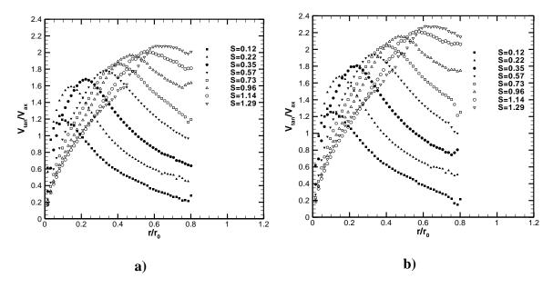
Figure 4-5: Radial profiles of the tangential velocity normalized with the axial velocity for various swirl ratios at z=5 cm: a)  $Re_r=6.7\times10^4$  and b)  $Re_r=8.4\times10^4$ .
