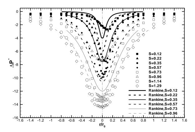
Figure 4-10: Surface static pressure deficits, averaged over time and azimuth for various swirl ratios at  $Re_r$ =6.7×10<sup>4</sup>.
