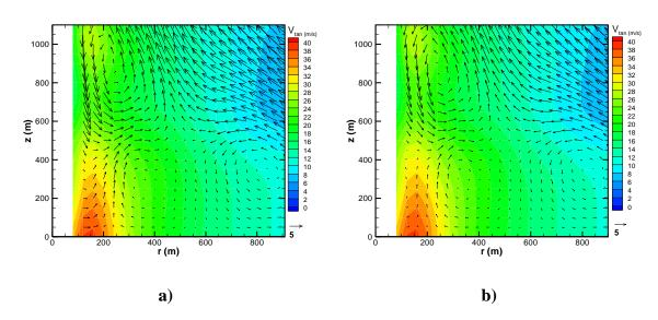
Figure 5-3: GBVTD retrieved structure of the Hp v2 at 0203:20 UTC, vertical velocity vector maps superimposed on tangential velocity contours, a) without and b) with correction for centrifuging.
