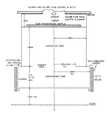
Figure 2-4: Schematic of the Purdue TVC – image from [6].
