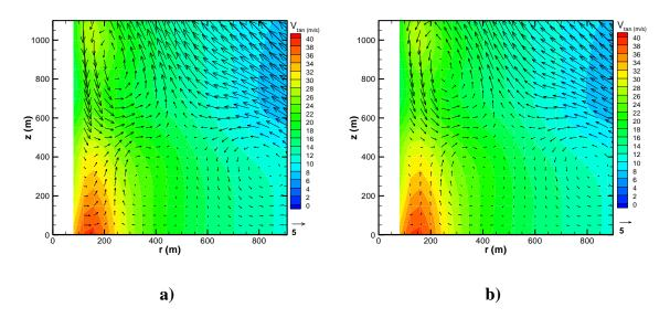
Figure 5-6: Vertical structure of the vortex along with the tangential velocity contours for Hp v2 at 0203:20 UTC with a)  $C_{max}$ =0 m/s and b)  $C_{max}$ =2 m/s.
