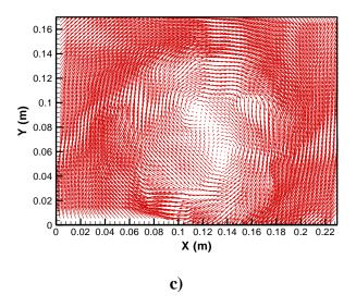
Figure 3-13: Instantaneous horizontal velocity vector maps obtained from PIV measurements at z=3.5 cm for a)  $\theta=10^{\circ}$ , b)  $\theta=20^{\circ}$  and c)  $\theta=30^{\circ}$ .
