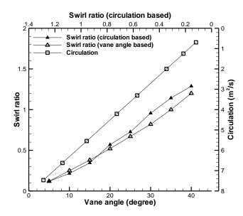
Figure 4-4: Swirl ratio variation with the vane angle as well as circulation as a function of the swirl ratio.
