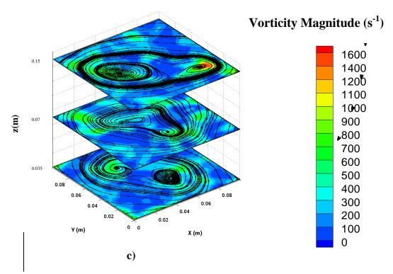
Figure 4-17: Streamlines superimposed on the instantaneous vertical vorticity contour maps at z=0.035, 0.07 and 0.15 m for a) S=0.22, b) S=0.57 and c) S=0.96.
