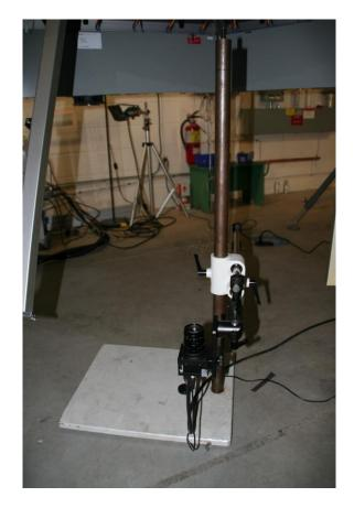
Figure 3-6: Camera setup for horizontal plane measurements.
