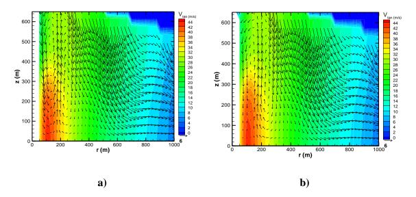
Figure 5-9: Vertical velocity vector maps superimposed on tangential velocity contours for GC v3 at 2218:50 UTC with a)  $C_{max}$ =0 m/s and b)  $C_{max}$ =2 m/s.
