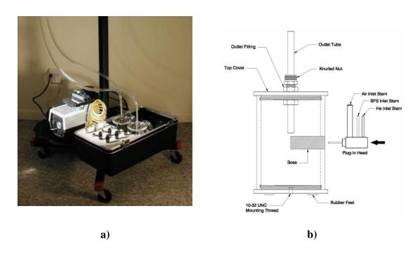
Figure 3-1: a) Helium bubble generator console and b) Mini vortex filter.
