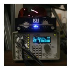
Figure 3-11: Frame grabber (top) and pulse/delay generator (bottom).
