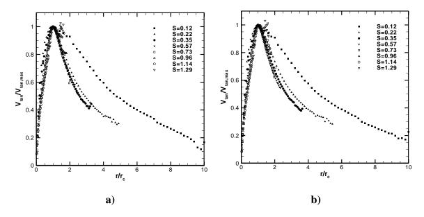
Figure 4-7: Normalized tangential velocities vs. radius for various swirl ratios at z= 5 cm: a)  $\text{Re}_r = 6.7 \times 10^4 \text{ and b}$ )  $\text{Re}_r = 8.4 \times 10^4$ .
