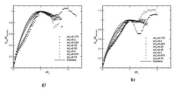
Figure 4-13: Radial profiles of the normalized tangential velocity at various heights and for a) S=0.12, b) S=0.22, c) S=0.35, d) S=0.57, e) S=0.73, f) S=0.96, g) S=1.14 and h) S=1.29.
