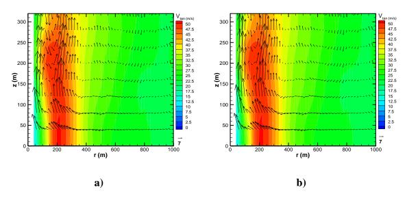
Figure 5-10: Vertical velocity vector maps superimposed on tangential velocity contours for Stc v1 at 2240:26 UTC with a)  $C_{max}$ =0 m/s and b)  $C_{max}$ =2 m/s.
