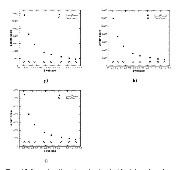
Figure 6-5: Geometric scaling ratio as a function of swirl ratio for various volumes of full-scale data; a) Clr v1, b) Hp v2, c) Hp v1, d) GC v1, e) GC v2, f) GC v3, g) Stc v1, h) Sp v1 and i) Sp v2.
