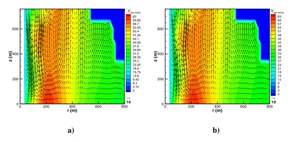
Figure 5-12: Vertical velocity vectors superimposed on tangential velocity contours for Sp v2 at 0140:02 UTC with a)  $C_{max}$ =0 m/s and b)  $C_{max}$ =2 m/s.
