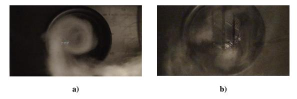
Figure 4-9: Converging flow close to the surface visualized using dry ice; a) single-celled and b) two-celled tornado-like vortex.
