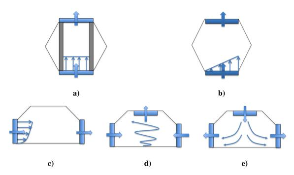
Figure 2-7: Five operational scenarios for WindEEE Dome include a) uniform straight flows, b) shear flows, c) boundary layer flows, d) tornado flows with translation and e) downburst flows with translation.
