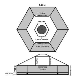
Figure 4-3: Schematic drawing of the MWD.
