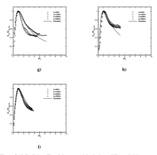
Figure 5-13: Radial profiles of the tangential velocity at different heights compared with Modified Rankine vortex model for a) Clr v1, b) Hp v1, c) Hp, v2, d) GC v1, e) GC v2, f) GC v3, g) Stc v1, h) Sp v1 and i) Sp v2.
