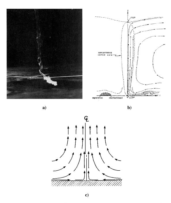
Figure 2-10: a) laminar core of a simulated vortex [6] and schematic drawing of the flow structure showing the separation-reattachment regions proposed by b) Snow [18] and c) Davies-Jones [20].
