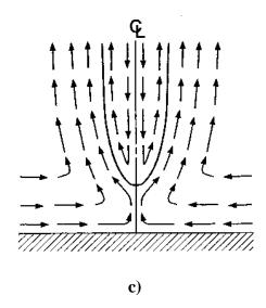
Figure 2-11: a) smoke-traced flow with breakdown aloft [10] and drawing of a vortex configuration at breakdown stage proposed by b) Snow [19] and c) Davies-Jones [20].
