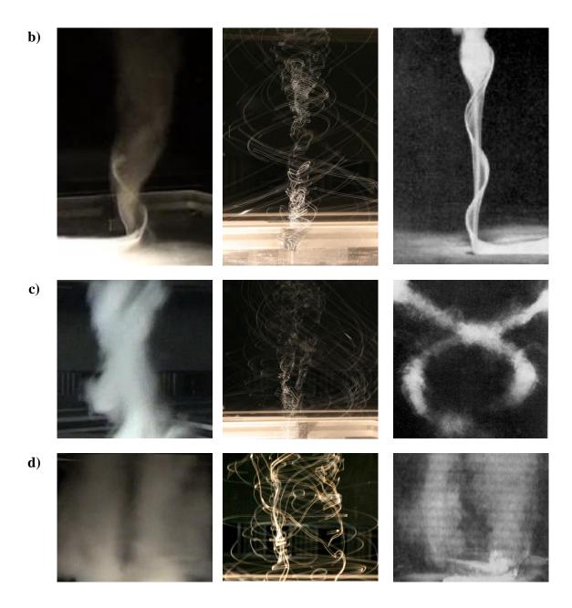
Figure 4-8: Tornado-like vortex produced in MWD and compared with previous works in TVCs: a) laminar core, S=0.12, b) vortex breakdown and touch-down, S=0.35-0.57, c) intertwined helical vortices, S=0.57-0.96 and d) two-celled vortex, S=0.96-1.29. (i) dry ice, MWD, (ii) helium bubbles, MWD and (iii) smoke, TVCs. Figures a(iii) [22] b(iii) [11] c(iii) [22] d(iii) [11] ©American Meteorological Society. Used with permission.
