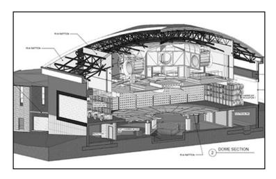
Figure 4-1: Cross-section of WindEEE Dome.
