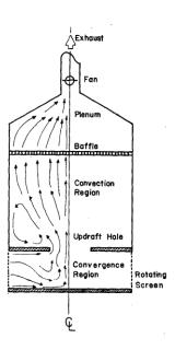
Figure 2-3: Schematic of the major components of the Ward-type TVC – image from [6].
