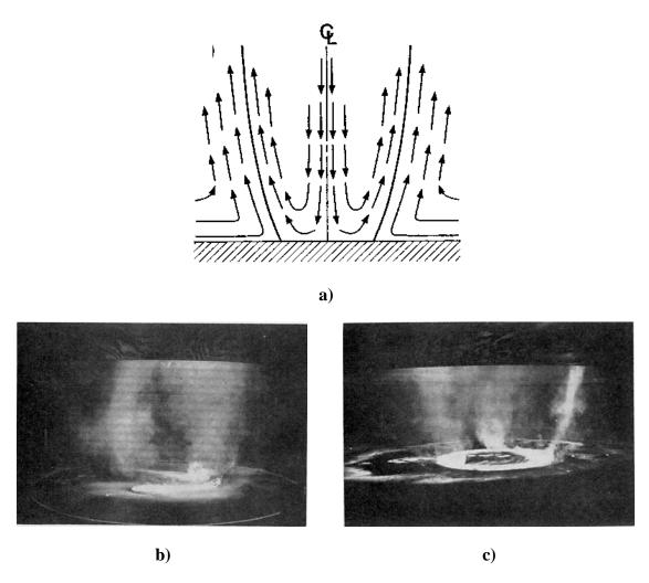
Figure 2-13: a) Vertical structure of a two-celled vortex – image from [20] and a family of b) two- and c) three-celled vortices simulated in TVCs – image from [10].
