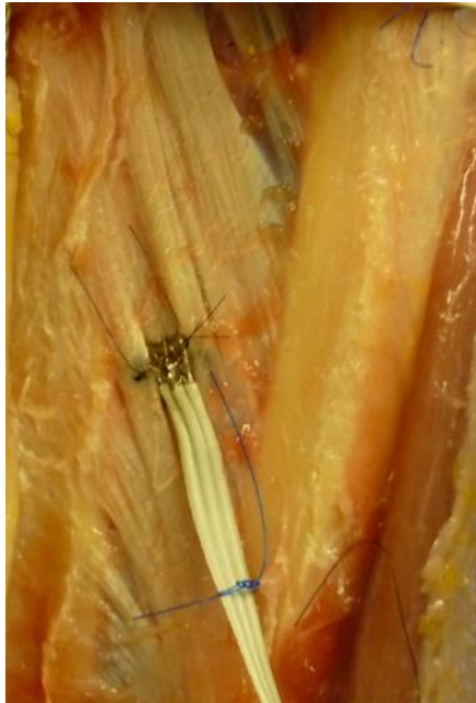
Figure 4.2: Load cell sutured to the IOM after being woven into the central band of the IOM
