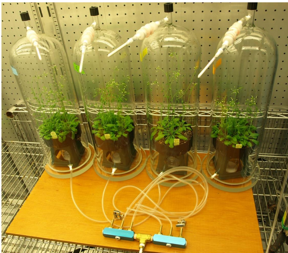
Figure 3: Collection of the headspace volatiles from six-week-old Arabidopsis plants. Headspace volatiles were collected over a 24 h period from flowering Arabidopsis plants onto Porapak Q columns.
