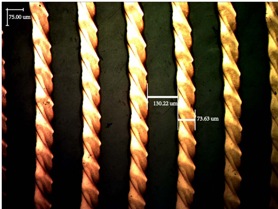
Figure 16: Microscope image of a part of micro inductive coil fabricated by the proposed method
