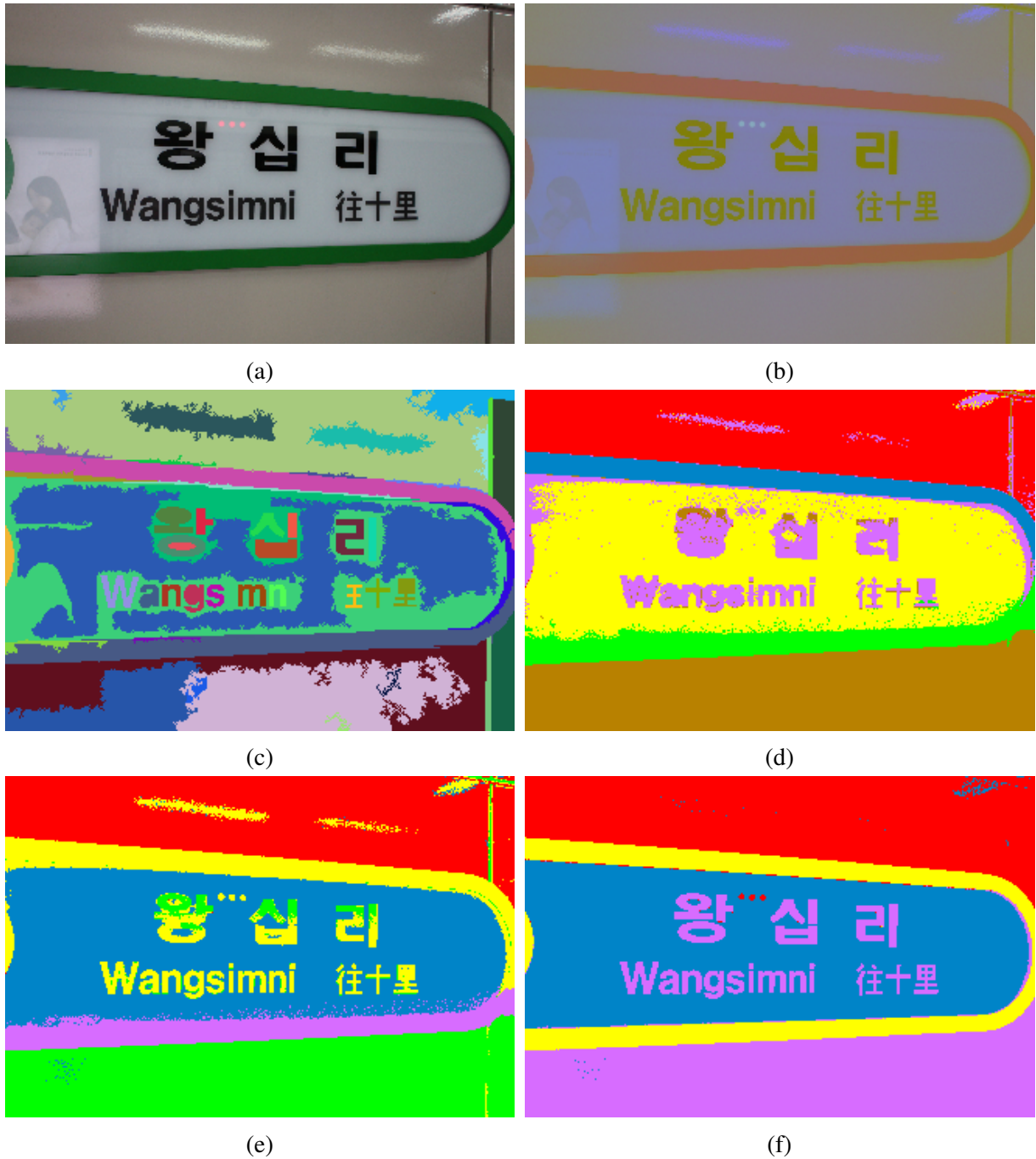
Figure 4.6: Signboard fitting. Example 2. a) input image, b) image in Lab color space, c) super pixels, d) first iteration of signboard fitting, e) intermediate iteration and f) final result.
