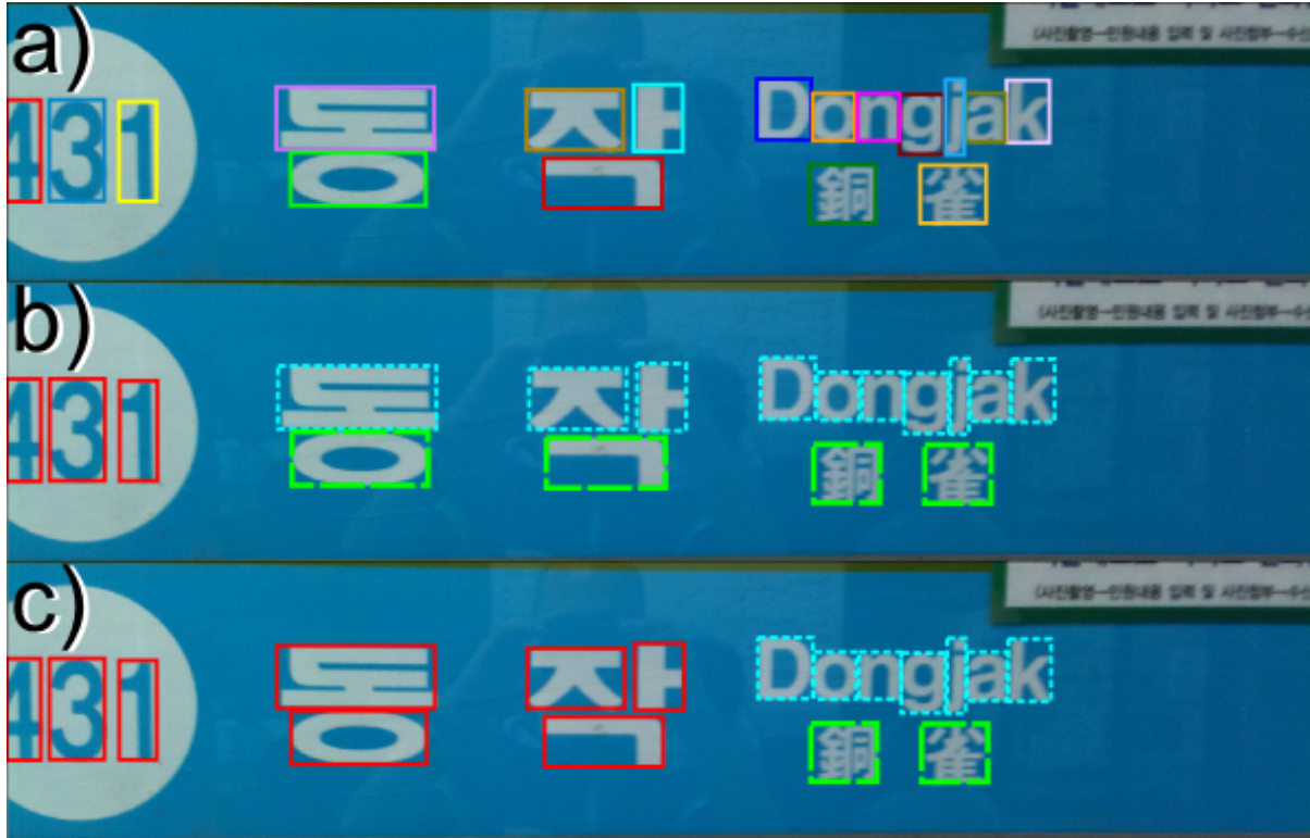
Figure 1.2: Korean characters introduce ambiguity to text line detection. a) Boxes show isolated blobs detected in the image. b) Blobs are split into text lines incorrectly: two Korean words in the center are cut. c) Correct text lines: one line on the left and two lines on the right.
