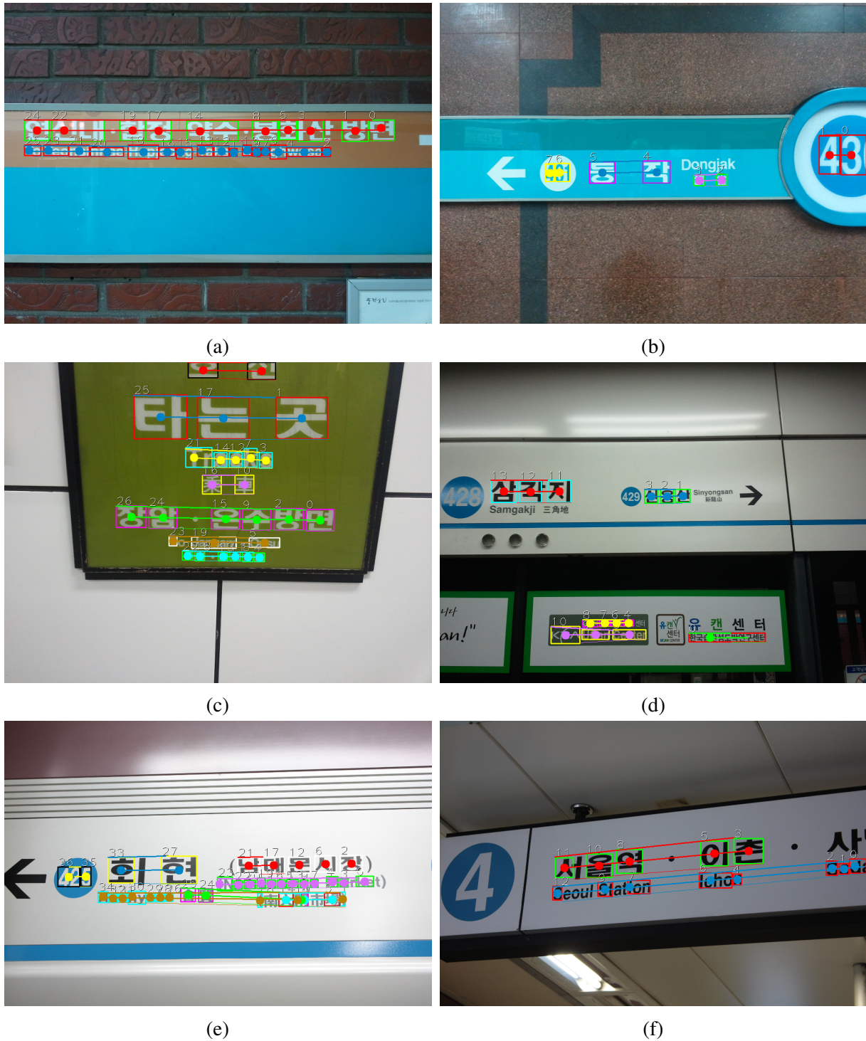
Figure 7.1: Results of text line detection. Triplet of lines in one colour shows one line. Circles mark centres of text blobs. Some blobs were misclassified in b),d),e) and f).
