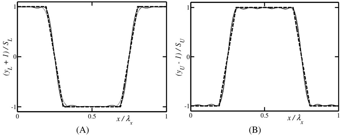
**Figure 4-18:** The optimal shapes for the equal depth grooves placed on both walls. Solid line identifies  $S_L = S_U = 0.2$  and  $\alpha = 0.1$ , whilst dotted line is for  $S_L = S_U = 0.5$  and  $\alpha = 1$ . Thick lines illustrate the best-fitted trapezoids with  $a = b = 1.25\lambda/11$  and  $c = d = 4.25\lambda/11$ .
