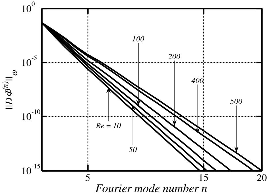
**Figure 2-5:** Variations of the Chebyshev norm  $\|D\phi^{(n)}\|_{\infty}$  defined by Eq. (2.2.53) as a function of the Fourier mode number  $n$  for the model geometry described by Eq. (2.2.52) with the ribs' amplitude  $S = 0.04$ , the ribs' wave number  $\alpha = 2$  and the average radius of the inner cylinder  $R_1 = 1.5$  for selected values of the flow Reynolds number  $Re$ . Calculations have been carried out using  $N_M = 20$  Fourier modes and  $N_T = 70$  Chebyshev polynomials.
