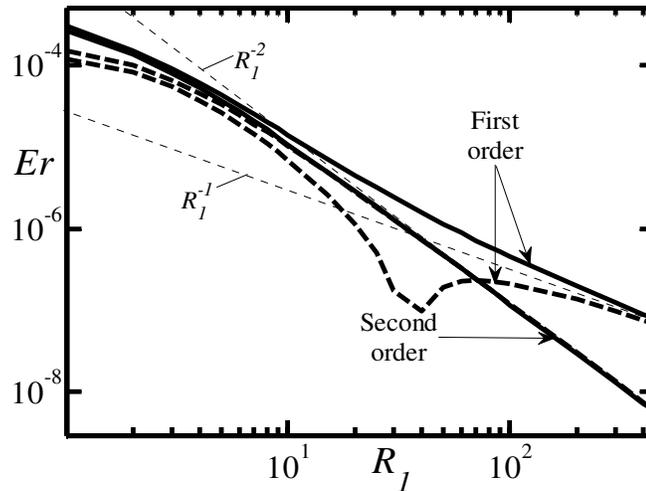
**Figure 3-2:** Variations of the error of the asymptotic approximation for  $R_1 \rightarrow \infty$ . Solid lines correspond to grooves placed at the inner cylinder (Eq. 3-6) with  $M = 8$  and  $S_{in} = 0.15$  and dashed lines correspond to the same grooves placed at the outer cylinder (see Eq. B-1).
