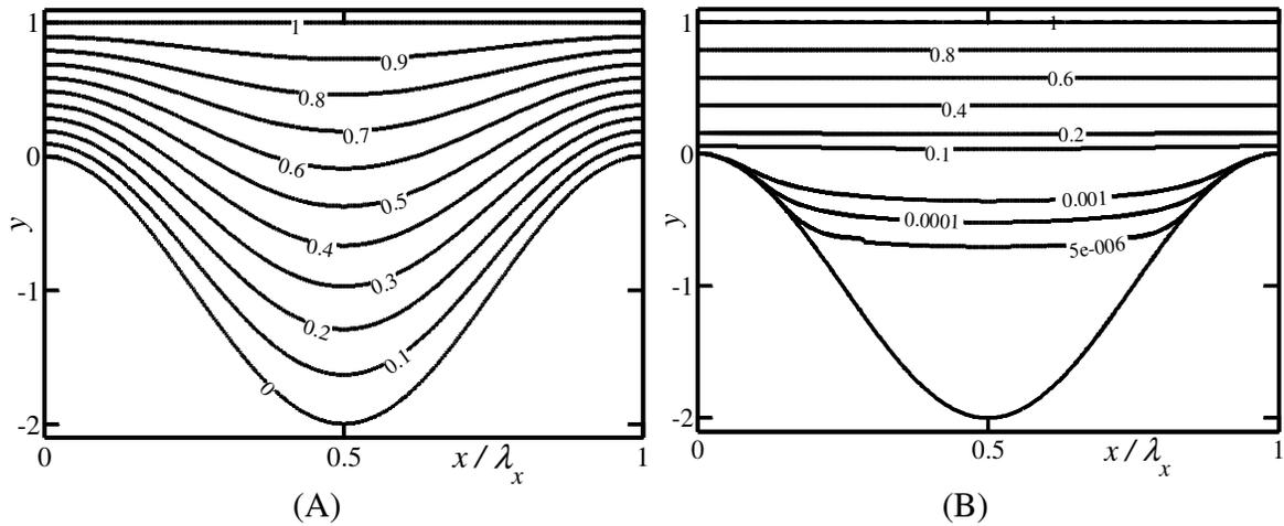
**Figure 4-3:** Temperature distribution inside the channel for the grooves described by Eq. (4.4.1) with the amplitude  $S_L = 1$  and the wave number  $\alpha = 0.5$  (Figure 4-3A) and  $\alpha = 30$  (Figure 4-3B).
