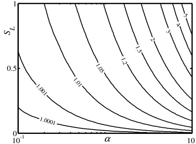
**Figure 4-6:** Variations of the wetted surface area  $A/A_0$  (see Eq. (4.3.13)) as a function of the groove amplitude  $S_L$  and the wave number  $\alpha$  for the groove geometry described by Eq. (4.4.1).
