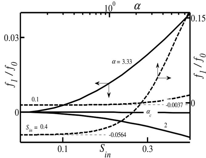
**Figure 3-10:** Variations of the normalized modification friction factor  $f_1/f_0$  induced by the grooves placed at the inner cylinder with the shape defined by Eq. (3.5.3) with  $S_{ave,out} = S_{ave,in} = S_{out} = 0$  and  $M = 4$ , as a function of the amplitude  $S_{in}$  (solid lines) and as a function of the wave number  $\alpha = M/R_1$  (dashed lines).
