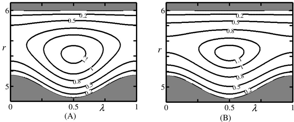
**Figure 3-14:** Distribution of the axial velocity component in an annulus with the geometry defined by Eq. (3.5.3) with  $S_{in} = 0.3$ ,  $R_1 = 5$ ,  $S_{ave,out} = S_{ave,in} = S_{out} = 0$  and  $M = 5$  (Figure 3-14A) and  $M = 15$  (Figure 3-14B).
