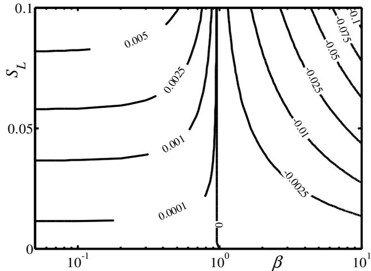
**Figure 5-3:** Variations of the pressure gradient correction  $Re dp_1/dx$  as a function of the groove wave number  $\beta$  and the groove height  $S_L$  for groove geometry described by Eq. (5.2.21).
