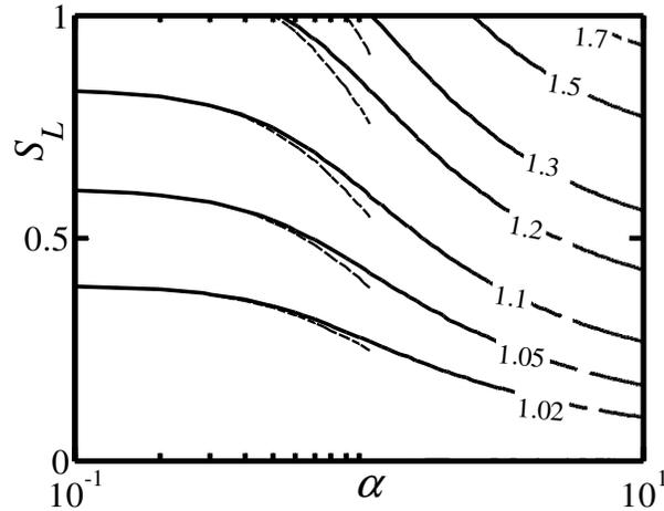
**Figure 4-2:** Variation of  $Q/Q_0$  as a function of the groove amplitude  $S_L$  and the wave number  $\alpha$  for the geometry described by Eq. (4.4.1). Dashed lines identify asymptotic values for  $\alpha \rightarrow 0$ .
