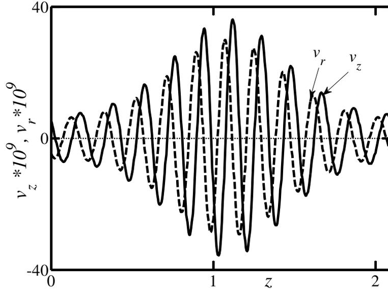
**Figure 2-7:** Distributions of the velocity components  $v_z$  and  $v_r$  evaluated along the inner cylinder for the model geometry described by Eq. (2.2.52) with the ribs' wave number  $\alpha = 3$ , the ribs' amplitude  $S = 0.05$  and the average radius of the inner cylinder  $R_1 = 1$ . Calculations have been carried out for the flow Reynolds number  $Re = 50$  using  $N_M = 10$  Fourier modes and  $N_T = 40$  Chebyshev polynomials.
