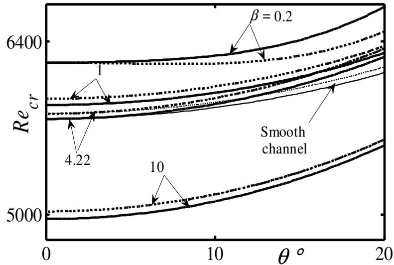
**Figure 5-8:** Variations of the critical Reynolds number of disturbances with the wave vector  $\mathbf{q} = (\delta, \mu)$  of constant magnitude as a function of its inclination angle  $\theta$  for the groove geometry described by Eq. (5.2.21) with the amplitude  $S_L = 0.05$ . Solid lines correspond to  $|\mathbf{q}| = 1.02$  and dotted lines to  $|\mathbf{q}| = 1.0$ .
