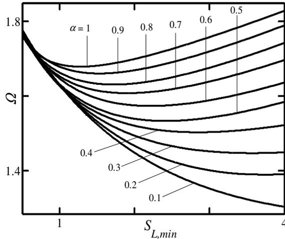
**Figure 4-20:** Variations of the thermal enhancement factor  $\Omega$  for a channel with the smooth upper wall and the optimal grooves with height  $S_{L,max} = 1$  placed at the lower wall as a function of the depth of the grooves  $S_{L,min}$ .
