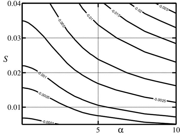
**Figure 2-13:** Variations of the additional pressure loss generated by the ribs with geometry defined by Eq. (2.2.52) as a function of the rib's amplitude  $S$  and the ribs' wave number  $\alpha$  for the flow Reynolds number  $Re = 10$  and the average radius of the inner cylinder  $R_1 = 1$ .
