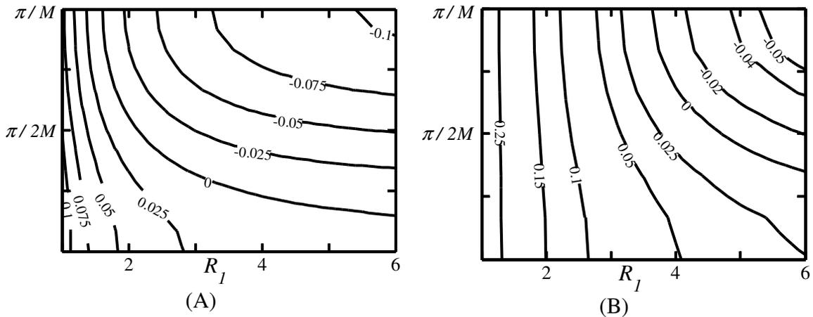
**Figure 3-12:** Variations of the normalized modification friction factor  $f_1/f_0$  as a function of the groove phase difference  $\varphi$  and the radius of the inner cylinder  $R_1$  for the grooves described by Eq. (3.5.3) with  $S_{in} = S_{out} = 0.3$  and  $S_{ave,out} = S_{ave,in} = 0$ . Results for  $M = 5, 10$  grooves are displayed in Figure 3-12A and Figure 3-12B, respectively.
