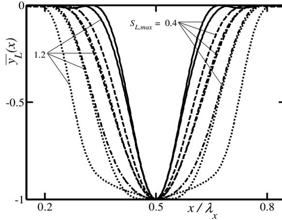
**Figure 4-22:** Shapes of the unequal-depth grooves with height  $S_{L,max}$  corresponding to the optimal depth placed at the lower wall. The y-coordinate is scaled using the groove peak-to-bottom distance  $\bar{y}_L(x) = [y_L(x) - S_{L,min}]/(S_{L,max} - S_{L,min}) - 1$ . Solid, dashed, dash-dotted, and dotted lines correspond to  $\alpha = 0.1, 0.5, 0.8, 1.0$ , respectively.
