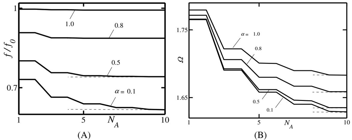
**Figure 4-12:** Variations of the normalized friction factor  $f/f_0$  and the thermal enhancement factor  $\Omega$  for the equal-depth grooves with amplitude  $S_L = 1$  as a function of the number of Fourier modes  $N_A$  used in the description of the groove geometry.
