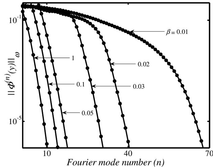
**Figure 5-5:** Variations of the Chebyshev norm  $\|\Phi^{(n)}(y)\|_{\omega}$  (see Eq. (5.3.14)) as a function of the Fourier mode number  $n$  for the groove geometry described by Eq. (5.2.21) with  $S_L = 0.05$ , for flow Reynolds number  $Re = 6500$  and disturbance wave numbers  $\delta = 1.02$ ,  $\mu = 0$ .
