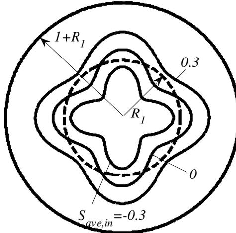
**Figure 3-4:** Sketch of the test configuration used to demonstrate the effect of the average position  $S_{ave,in}$  of the grooves. Four grooves ( $M = 4$ ) with the shape defined by Eq. (3.5.3) with  $S_{in} = 0.3, S_{out} = 0, S_{ave,out} = 0$  are placed at three different average locations: Case A –  $S_{ave,in} = 0.3$ ; Case B –  $S_{ave,in} = 0$ ; Case C –  $S_{ave,in} = -0.3$ . See text for details.
