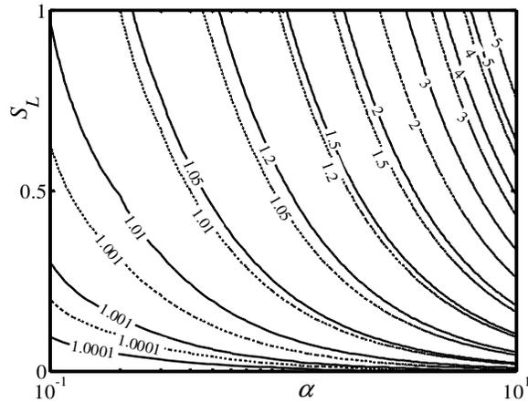
**Figure 4-16:** Variations of the wetted surface area  $A/A_0$  (see Eq.(4.3.13)) as a function of the groove wave number  $\alpha$  for the same grooves as used in Figure 4-15. Dashed lines identify results for the simple sinusoidal grooves.
