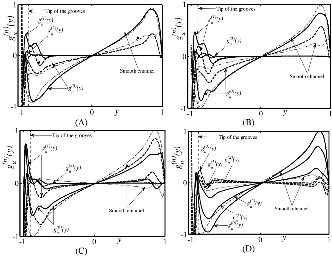
**Figure 5-10:** Eigenfunctions  $g_u^{(n)}(y)$ ,  $n = 0, 1, 2$ , describing two-dimensional travelling wave disturbances with the wave number  $\delta = 1.02$  in a channel with grooves whose geometry is described by Eq. (5.2.21) with  $S_L = 0.05$ . Results displayed in Figs. 5-10A, B, C, and D correspond to the onset conditions for the groove wave numbers  $\beta = 10, 4.22, 1.0$ , and  $0.2$ , i.e.
