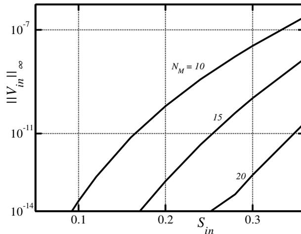
**Figure 2-20:** Variations of the norm  $\|V_{in}\|_{\infty}$  defined by Eq. (2.3.38) as a function of the ribs' inner amplitude  $S_{in}$  for the model configuration described by Eq. (2.3.37). Calculations have been carried out for the smooth outer cylinder ( $S_{out} = 0$ ) and the average radius of the inner cylinder  $R_1 = 1$  using  $N_T = 70$  Chebyshev polynomials and selected number of the Fourier modes  $N_M$ .
