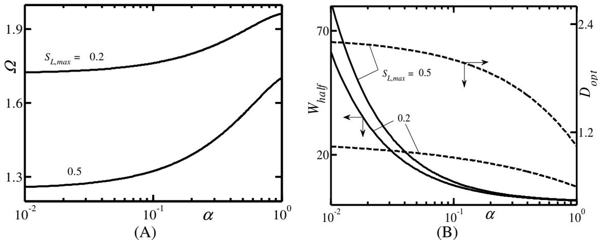
**Figure 4-25:** Variations of the thermal enhancement factor  $\Omega$  (Figure 4-25A) and the corresponding optimal depth  $D_{opt}$  and the width at half height  $W_{half}$  (Figure 4-25B) as a function of the groove wave number  $\alpha$  for the optimal geometry with grooves placed on both walls and moved by half wavelength with respect to each other.
