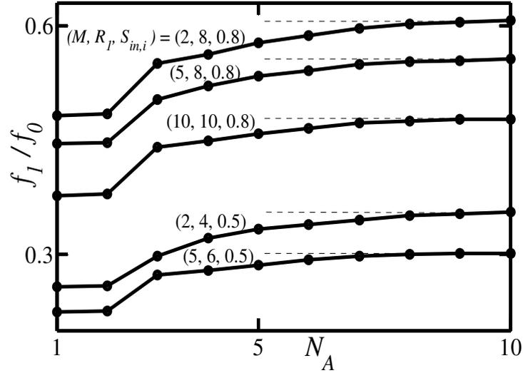
**Figure 3-16:** Variations of the normalized modification friction factor  $f_1/f_0$  as a function of the number of Fourier modes used for description of the optimal shape of the equal-depth grooves placed at the inner cylinder.
