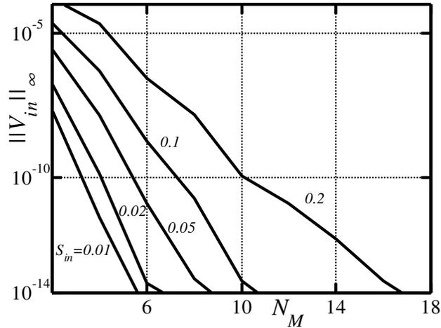
**Figure 2-19:** Variations of the norm  $\|V_{in}\|_{\infty}$  defined by Eq. (2.3.38) as a function of the number of Fourier modes  $N_M$  used in the computations for the model problem described by Eq. (2.3.37) for selected values of the inner ribs' amplitude  $S_{in}$ . Calculations have been carried out for the smooth outer cylinder ( $S_{out} = 0$ ) and the average radius of the inner cylinder  $R_1 = 1$  using  $N_T = 70$  Chebyshev polynomials.
