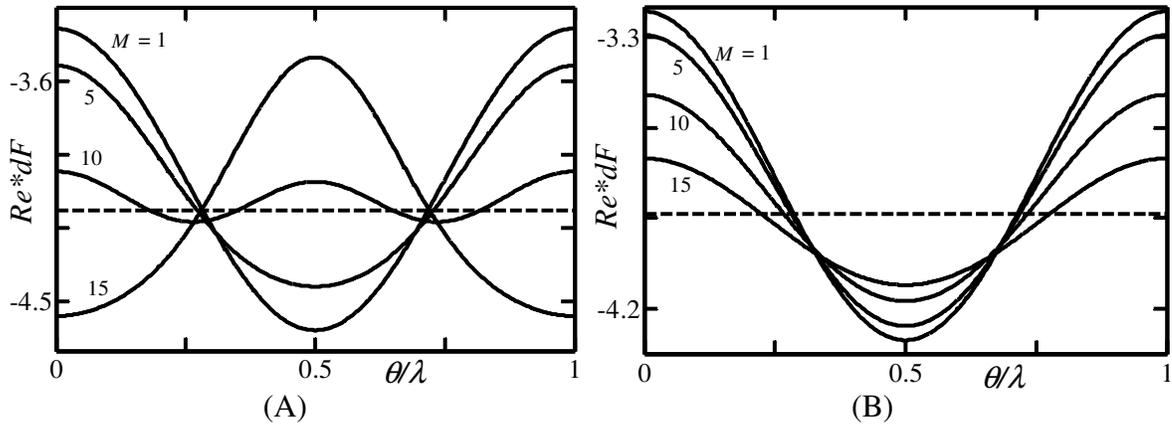
**Figure 3-13:** Distribution of the axial component of shear stress acting on the fluid at the inner (Figure 3-13A) and outer (Figure 3-13B) cylinders for grooves with the geometry defined by Eq. (3.5.3) with  $S_{in} = 0.3$ ,  $S_{out} = 0$ ,  $R_1 = 5$ , and  $S_{ave,out} = S_{ave,in} = 0$ . Dashed lines provide reference values for the smooth cylinders.
