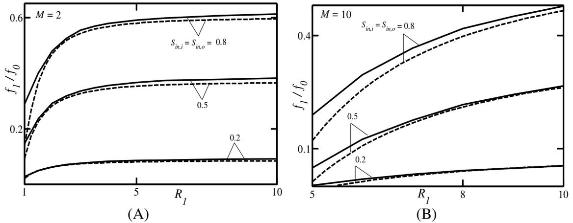
**Figure 3-18:** Variations of the normalized modification friction factor  $f_1/f_0$  for  $M = 2$  equal-depth optimal grooves (Figure 3-18A) and  $M = 10$  similar grooves (Figure 3-18B) placed at the inner cylinder (solid lines). Modification friction factors for the same grooves approximated using the universal trapezoid are marked using dashed lines. See text for details.
