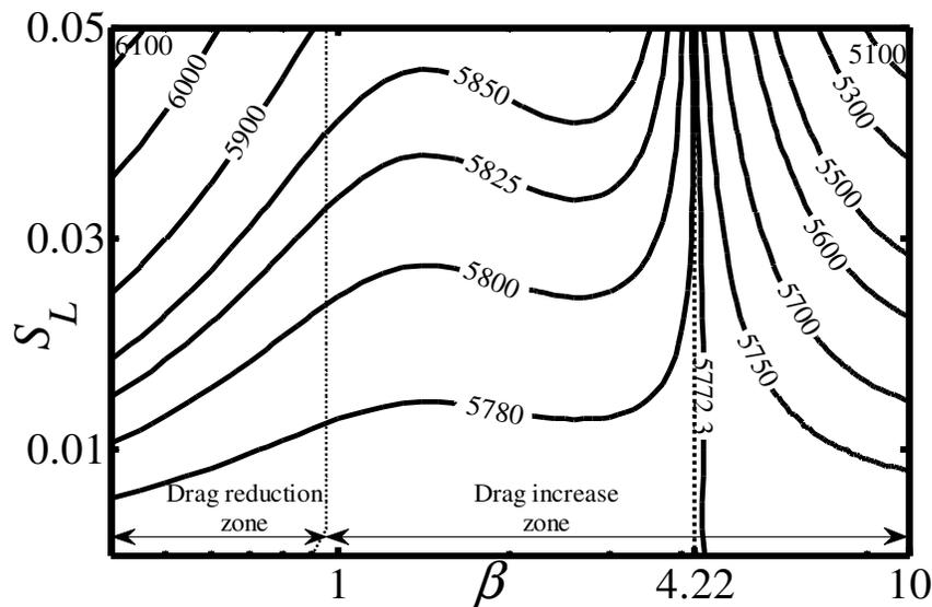
**Figure 5-15:** Variations of the critical Reynolds number  $Re_c$  as a function of the groove wave number  $\beta$  and the groove amplitude  $S_L$  for channel with geometry described by Eq. (5.2.21).
