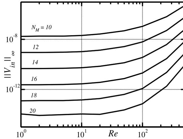
**Figure 2-11:** Variation of the norm  $\|V_{in}\|_{\infty}$  defined by Eq. (2.2.54) as a function of the flow Reynolds number  $Re$  for an annulus with geometry defined by Eq. (2.2.52) with the ribs' wave number  $\alpha = 4$ , the ribs' amplitude  $S = 0.04$  and the average radius of the inner cylinder  $R_1 = 1$  determined using different number of Fourier modes  $N_M$  and  $N_T = 70$  Chebyshev polynomials.
