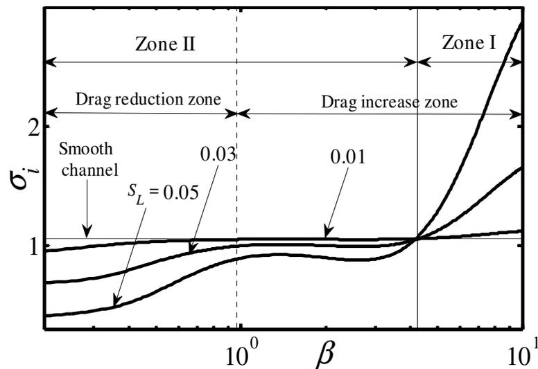
**Figure 5-9:** Variations of the growth rate  $\sigma_i \times 10^3$  of disturbances with the wave number  $\delta = 1.02$  as a function of the groove wave number  $\beta$  for the groove geometry described by Eq. (5.2.21) for flow with the Reynolds number  $Re = 6500$ . Dotted-line indicates the wave number that separates the drag reducing and drag increasing zones.
