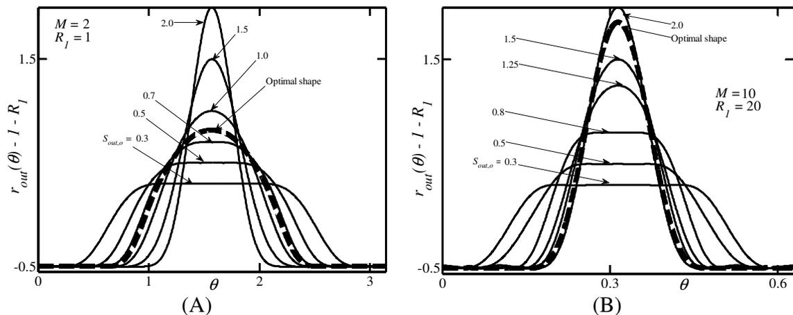
**Figure 3-23:** Evolution of the optimal shape of the unequal-depth grooves placed at the outer cylinder as a function of the depth of the groove  $S_{out,o}$ . The height of the groove is set at  $S_{out,i} = 0.5$ . The results presented in Figure 3-23A are for  $M = 2$ ,  $R_1 = 1$ , and in Figure 3-23B for  $M = 10$ ,  $R_1 = 20$ . Dashed lines illustrate shapes corresponding to the optimal depth.
