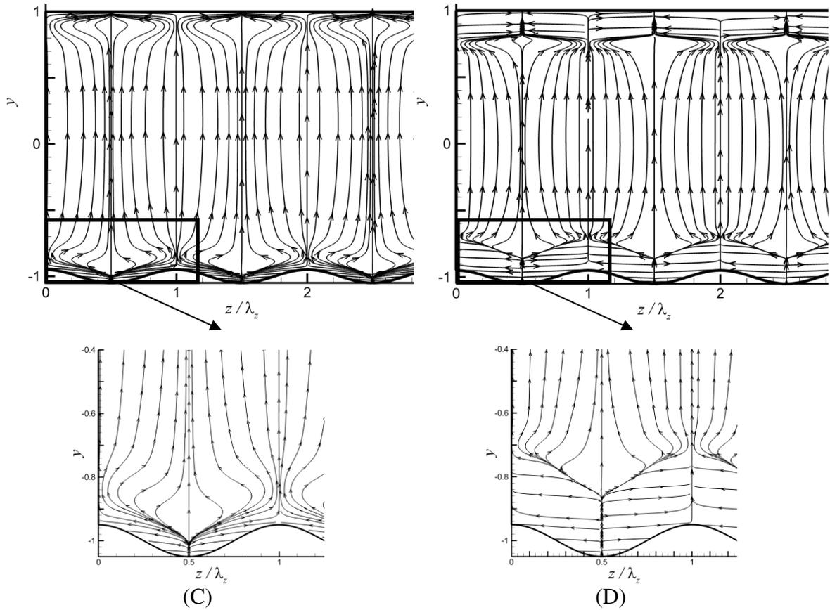
**Figure 5-11:** Pathlines in the  $y$ - $z$  plane for the disturbance flow field corresponding to “two-dimensional” disturbances with the wave number  $\delta = 1.02$  at the onset for flow in a channel with grooves described by Eq. (5.2.21) with  $S_L = 0.05$ . Figures 5-11A, B, C and D display results for  $(\beta, Re_c) = (10, 5028.5), (4.22, 5773.5), (1.0, 5886), (0.2, 6227.5)$ , respectively.
