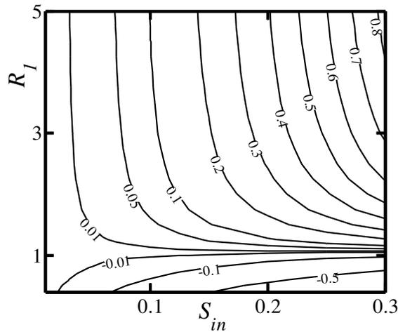
**Figure 2-24:** Variations of the additional pressure loss  $Re \partial p_1 / \partial z$  associated with the presence of the ribs at the inner cylinder while the outer cylinder is kept smooth ( $S_{out} = 0$ ) as a function of the ribs' amplitude  $S_{in}$  and the average radius of the inner cylinder  $R_1$ . The ribs' geometry is defined by Eq. (2.3.37). Computations were carried out using  $N_M = 20$  Fourier modes and  $N_T = 70$  Chebyshev polynomials.
