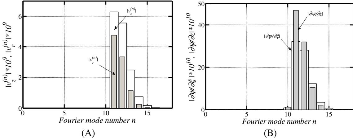
**Figure 2-8:** Fourier spectra of the velocity components  $v_z$  and  $v_r$  (Figure 2-8A) and of the stream function derivatives  $\partial\psi/\partial\xi$  and  $\partial\psi/\partial z$  (Figure 2-8B) evaluated at the surface of the inner cylinder. Other conditions as in Figure 2-7.
