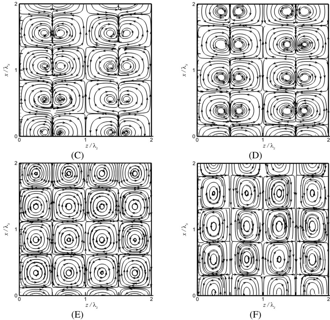
**Figure 5-12:** Pathlines in the  $x$ - $z$  plane at  $y = 0$  for the disturbance flow field corresponding to “two-dimensional” disturbances with the wave number  $\delta = 1.02$  at the onset for flow in a channel with grooves described by Eq. (5.2.21) with  $S_L = 0.05$ . Figures 5-12A, B, C, D, E and F display results for  $(\beta, Re_c) = (10, 5028.5), (5, 5652.4), (4.35, 5755), (4.22, 5773.5), (1.0, 5886), (0.5, 6073.1)$ , respectively.
