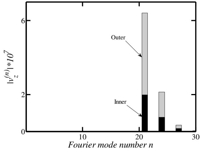
**Figure 2-22:** Fourier spectra of the axial velocity component  $v_z$  evaluated along the inner and outer cylinders for the model geometry described by Eq. (2.3.37). Other conditions as in Figure 2-21.
