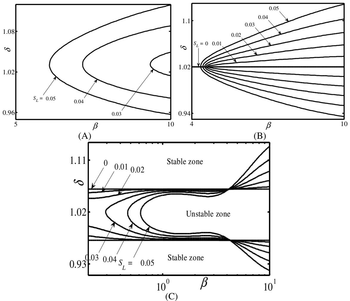
**Figure 5-14:** Neutral curves in the  $(\beta, \delta)$ -plane for the “two-dimensional” disturbances in a channel with grooves whose geometry is described by Eq. (5.2.21). Figures 5-14A, B and C display results for flow with  $Re = 5500, 5772.25, 6000$ , respectively.
