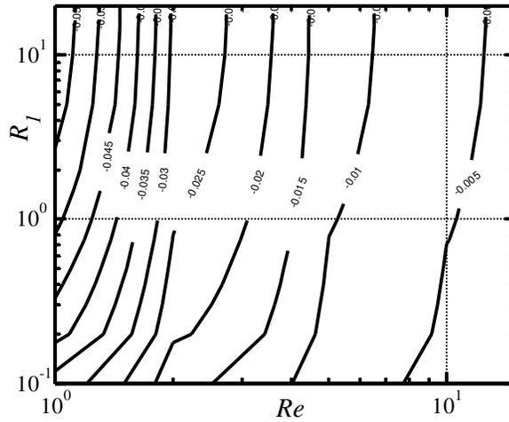
**Figure 2-14:** Variations of the additional pressure loss generated by the ribs with geometry given by Eq. (2.2.52) as a function of the flow Reynolds number  $Re$  and the average radius of the inner cylinder  $R_1$  for ribs with the wave number  $\alpha = 2$  and the amplitude  $S = 0.04$ .
