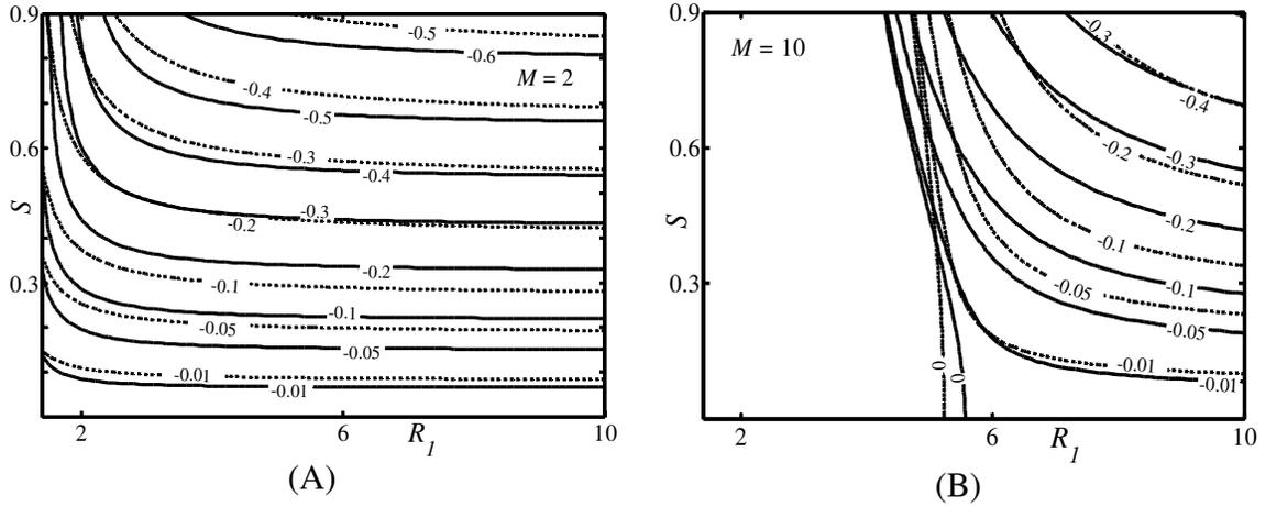
**Figure 3-19:** Variations of the normalized modification friction factor  $f_1/f_0$  as a function of the wall curvature  $R_1$  and the groove amplitude  $S_{in,i} = S_{in,o} = S$  for  $M = 2$  universal equal-depth trapezoidal grooves (Figure 3-19A) and  $M = 10$  similar grooves (Figure 3-19B) placed at the inner cylinder (see text for discussion). Dashed lines are for the sinusoidal grooves defined by
