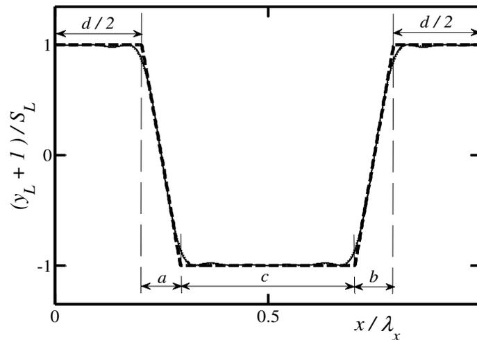
**Figure 4-13:** The optimal shapes of the equal-depth grooves. Solid line identifies a groove with  $S_L = 0.4$  and  $\alpha = 0.1$ , whilst dotted line is for  $S_L = 1.6$  and  $\alpha = 1$ . The y-coordinate is scaled using the groove depth. Thick line illustrates the best-fitted trapezoid characterized by  $a = b = \lambda/11$  and  $c = d = 4.5\lambda/11$ .
