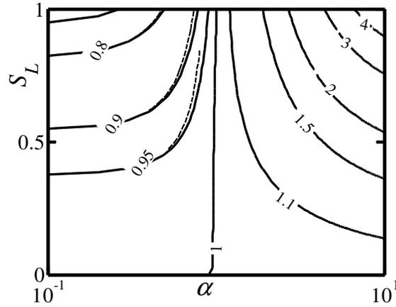
**Figure 4-7:** Variation of  $f/f_0$  as a function of the groove amplitude  $S_L$  and the wave number  $\alpha$  for the geometry described by Eq. (4.4.1). Dashed lines identify asymptotic values for  $\alpha \rightarrow 0$ .
