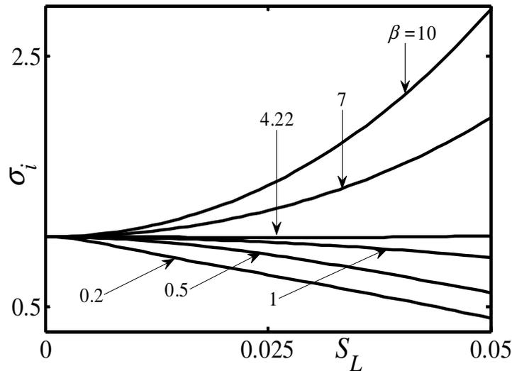
**Figure 5-7:** Variation of the growth rate  $\sigma_i \times 10^3$  of disturbances with the wave numbers  $\delta = 1.02$  and  $\mu = 0$  as a function of the groove amplitude  $S_L$  for the groove geometry described by Eq. (5.2.21) for flow with the Reynolds number  $Re = 6500$ .
