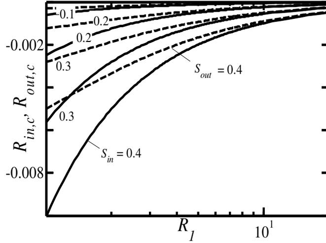
**Figure 3-3:** Variations of the geometric correction factors  $R_{in,c}$  and  $R_{out,c}$  as functions of  $R_1$  for the groove geometry described by Eq. (3.5.3) with  $S_{ave,in} = S_{ave,out} = \varphi = 0$  with the same grooves placed either at the inner cylinder (solid lines,  $S_{in} = 0.1$ ,  $S_{out} = 0$ ) or at the outer cylinder (dashed lines,  $S_{in} = 0$ ,  $S_{out} = 0.1$ ).
