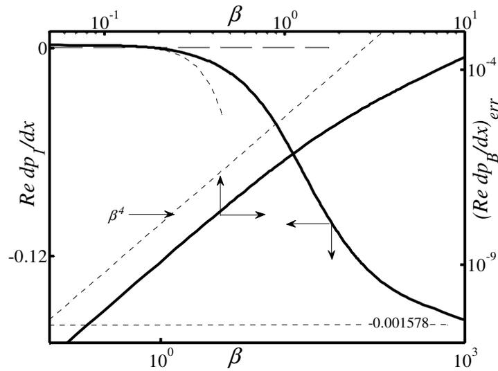
**Figure 5-2:** Variations of the error  $(dp/dx)_{err}$  of the small wave number approximation of the stationary state (see Eq. (5.2.23)) and variations of the pressure gradient correction  $Re dp_1/dx$  for grooves with geometry described Eq. (5.2.21) with  $S_L = 0.05$ . Dotted lines show the pressure-gradient asymptote for  $\beta \rightarrow 0$  and the lower bound for the pressure gradient for  $\beta \rightarrow \infty$ .
