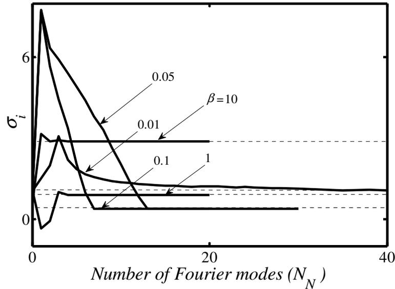
**Figure 5-6:** Variations of the growth rate  $\sigma_i \times 10^3$  of disturbances with the wave numbers  $\delta = 1.02$  and  $\mu = 0$  as a function of the number of Fourier modes used in the numerical solution of the stability problem for flow with the Reynolds number  $Re=6500$  in the grooved channel with the groove geometry described by Eq. (5.2.21) with  $S_L = 0.05$ .
