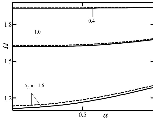
**Figure 4-17:** Variations of the thermal enhancement factor as a function of the groove wave number  $\alpha$  for the equal-depth grooves located on the lower wall. Solid and dashed lines correspond to grooves with the optimal and trapezoidal shapes, respectively.
