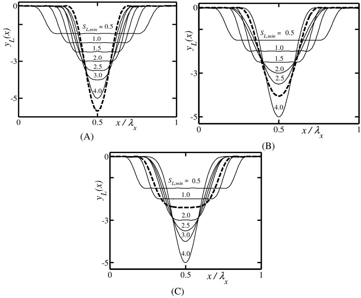
**Figure 4-21:** Evolution of the shape of the optimal, unequal-depth grooves with height  $S_{L,max} = 1$  placed on the lower wall as a function of the groove depth  $S_{L,min}$ . Results for  $\alpha = 0.1, 0.5, 1$  are displayed in Figure 4-21A, B and C, respectively. Dashed lines identify shapes corresponding to the optimal depth.
