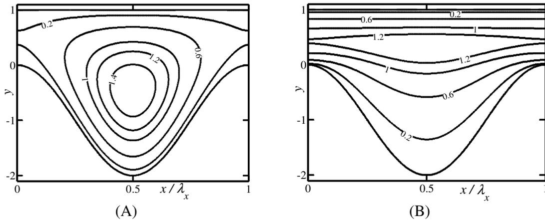
**Figure 4-8:** Distribution of the  $w$ -velocity component for grooves described by Eq. (4.4.1) with amplitude  $S_L = 2$  and the wave numbers  $\alpha = 0.5$  (Figure 4-8A) and  $\alpha = 5$  (Figure 4-8B).
