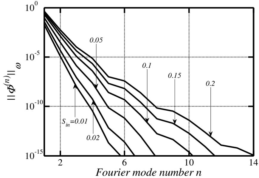
**Figure 2-18:** Variations of the Chebyshev norm  $\|\phi^{(n)}\|_{\omega}$  as a function of the Fourier mode number  $n$  for the model geometry described by Eq. (2.3.37) for selected values of the inner ribs' amplitude  $S_{in}$ . Calculations have been carried out for the smooth outer cylinder ( $S_{out} = 0$ ) and the average radius of the inner cylinder  $R_1 = 2$  using  $N_M = 20$  Fourier modes and  $N_T = 70$  Chebyshev polynomials.
