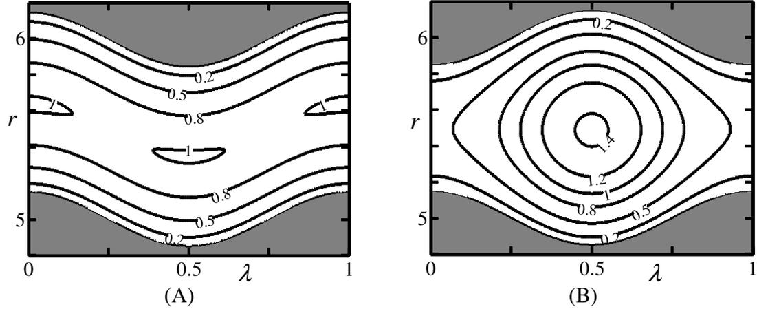
**Figure 3-15:** Distribution of the axial velocity component in an annulus with the geometry defined by Eq. (3.5.3) with  $S_{in} = S_{out} = 0.3$ ,  $R_1 = 5$ ,  $S_{ave,out} = S_{ave,in} = 0$ ,  $M = 5$ , and  $\varphi = 0$  (Figure 3-15A) and  $\varphi = \pi$  (Figure 3-15B).
