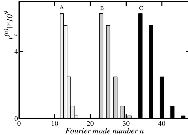
**Figure 2-9:** Fourier spectra of the axial velocity component  $v_z$  evaluated at the surface of the inner cylinder for ribs with the wavelength  $\lambda = 2\pi/3$ . Other conditions as in Figure 2-7. Solution have been obtained with  $\alpha = 3$  and  $N_M = 10$  in case A,  $\alpha = 1.5$  and  $N_M = 20$  in case B, and  $\alpha = 1$  and  $N_M = 30$  in case C.
