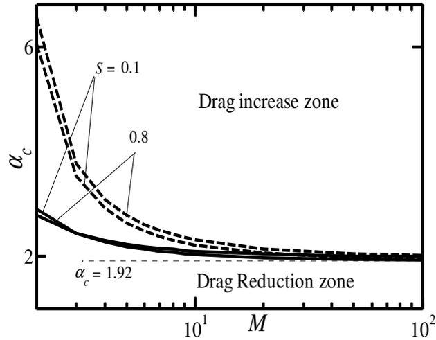
**Figure 3-11:** Variations of the critical groove wave number  $\alpha_c$  as a function of the number of grooves  $M$  for an annulus with geometry described by Eq. (3.5.3) with  $S_{ave,out} = S_{ave,in} = 0$ . Solid (dashed) line corresponds to the grooves placed only at the inner (outer) cylinder with  $S_{in} = 0.1$  and  $0.8$ ,  $S_{out} = 0$  ( $S_{in} = 0, S_{out} = 0.1$  and  $0.8$ ).
