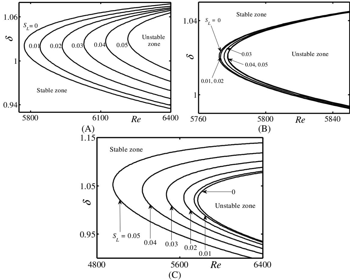
**Figure 5-13:** Neutral curves in the  $(Re, \delta)$ -plane for the “two-disturbances” with the wave numbers  $\delta = 1.02$  in a channel with grooves whose geometry is described by Eq. (5.2.21).
