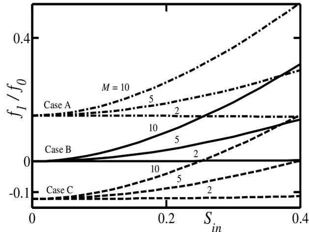
**Figure 3-5:** Variations of the normalized modification friction factor  $f_1/f_0$  as a function of the groove amplitude  $S_{in}$  for  $R_1 = 1$ . Four grooves ( $M = 4$ ) are placed at the inner cylinder with their geometry described by Eq. (3.5.3) with  $S_{ave,out} = S_{out} = 0$  and  $S_{ave,in} = 0.05, 0, -0.05$  in Cases A, B, C, respectively.
