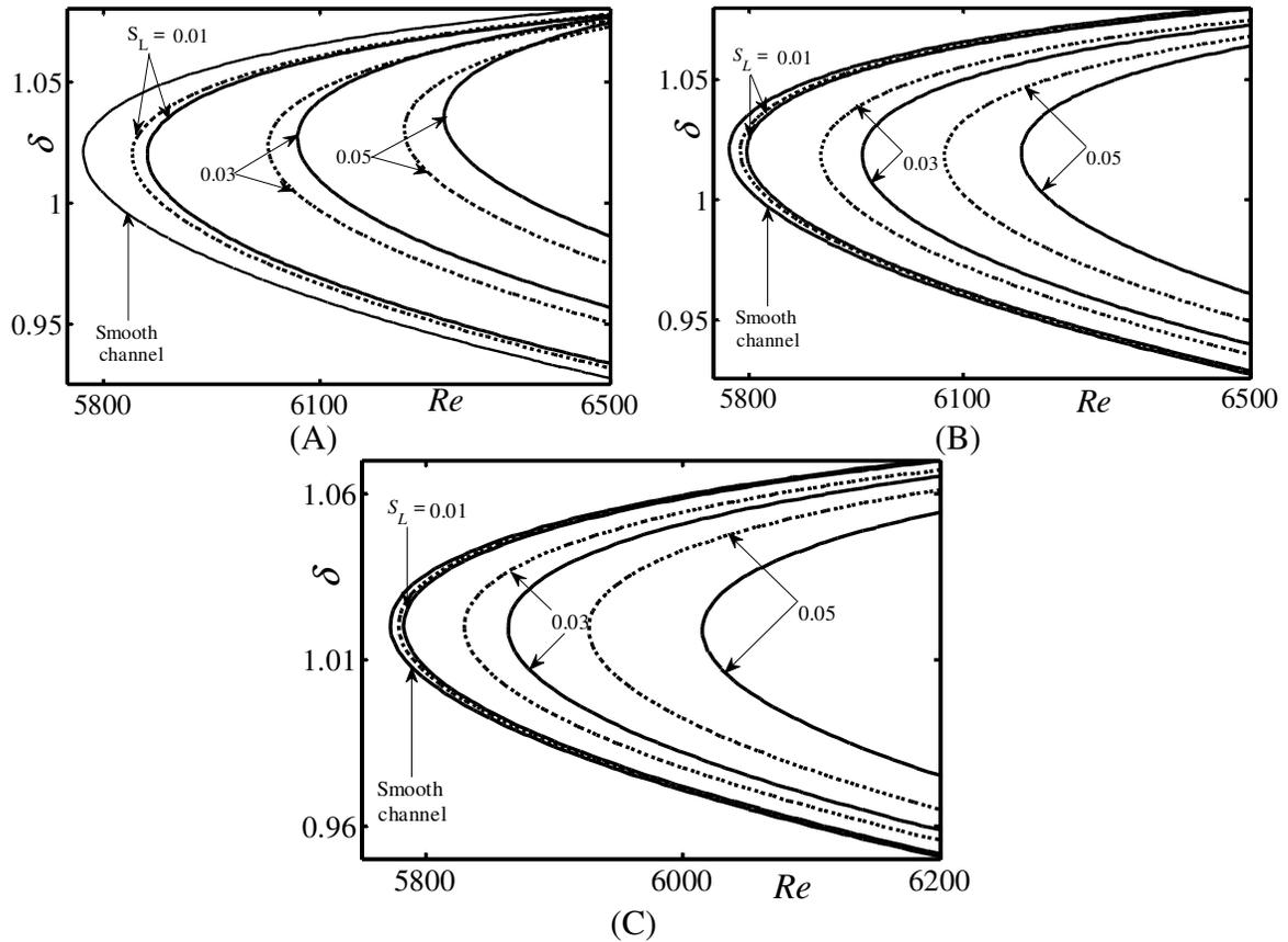
**Figure 5-19:** Neutral curves in the  $(Re, \delta)$ -plane for channel fitted with optimal, equal-depths grooves at the lower wall. Groove geometry is represented by the universal trapezoid with  $a = b = \lambda/8$  and  $c = d = 3\lambda/8$  (see Figure 5-18A for notation). Results for sinusoidal grooves are given for reference (dashed lines). Figure 5-19A, Figure 5-19B and Figure 5-19C provide results for the groove wave numbers  $\beta = 0.2, 0.5,$  and  $0.8,$  respectively.
