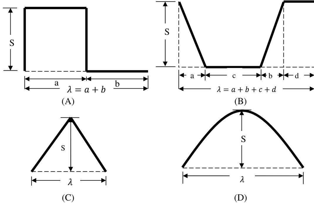
**Figure 3-6:** Shapes of the grooves used in this study: A- rectangular groove, B- trapezoidal groove, C- triangular groove, D- rectified groove ( $|\sin M\theta|$ ).  $\lambda$  denotes the length of one groove segment.
