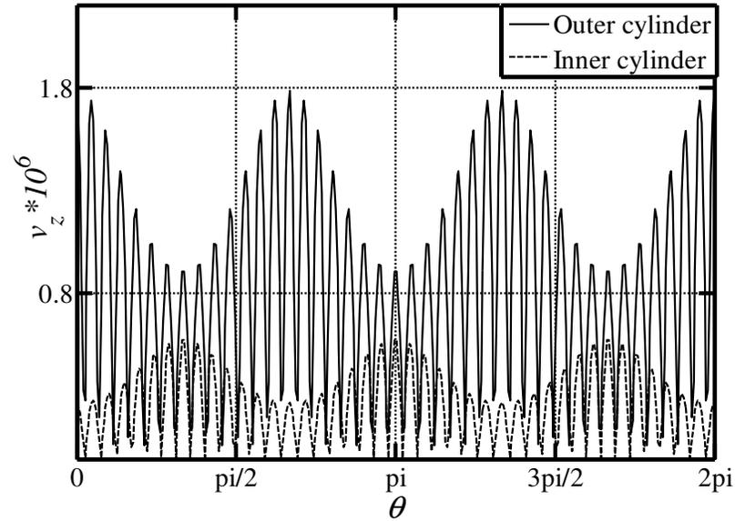
**Figure 2-21:** Distributions of the axial velocity component  $v_z$  evaluated along the inner and outer cylinders for the model geometry described by Eq. (2.3.37) with the ribs' inner and outer amplitudes  $S_{in} = 0.05$  and  $S_{out} = 0.1$ , respectively, and  $\theta$  replaced by  $3\theta$ . Calculations have been carried out for the average radius of the inner cylinder  $R_1 = 1$  using  $N_M = 20$  Fourier modes and  $N_T = 70$  Chebyshev polynomials.
