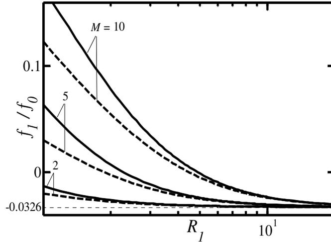
**Figure 3-8:** Variation of the normalized modification friction factor  $f_1/f_0$  as a function of  $R_1$  for the geometry described by (3.5.3) with  $S_{ave,out} = S_{out} = 0$  and  $M = 2, 5$  and  $10$ . Solid (dashed) lines correspond to the same grooves placed only on the inner (outer) cylinder with  $S_{in} = 0.3, S_{out} = 0$  ( $S_{out} = 0.3, S_{in} = 0$ ). Dotted line shows the normalized modification friction factor asymptote for  $R_1 \rightarrow \infty$ .
