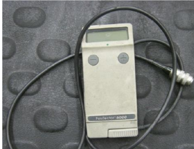
Figure 3.14 Coating Thickness Gauge
