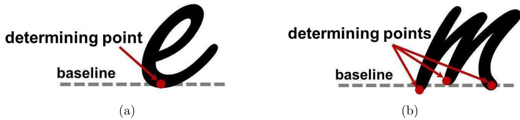
Figure 5.2: Baseline with (a) one determining point (b) multiple determining points.
