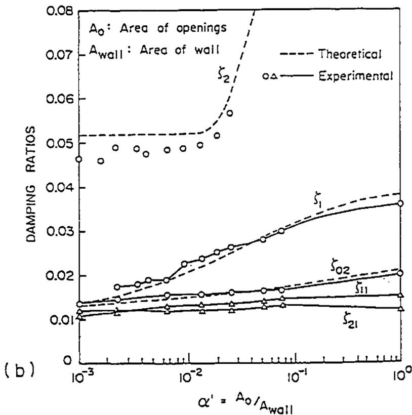
Fig. (4.8): Effect of wall openings on (a) frequencies and (b) damping ratios of the plate roof.
