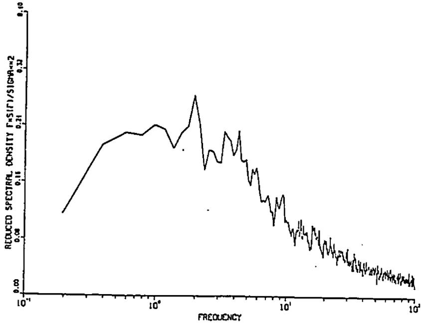
Fig. (7.11): Velocity spectrum for urban exposure
