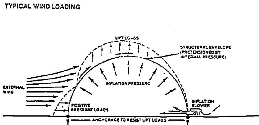
Fig. (5.3): Wind load distribution on a cylindrical roof (AFSI, 1977)
