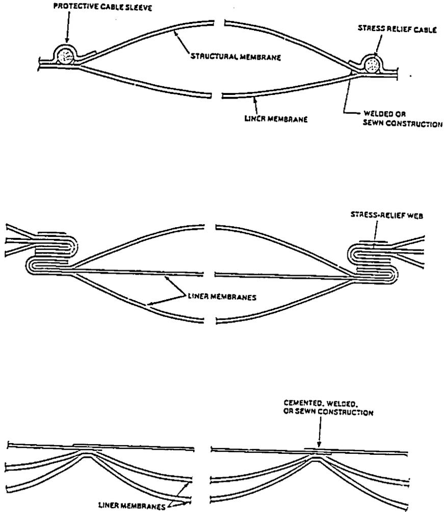
Fig. (5.1): Multiple membrane systems (AFSI, 1977)
