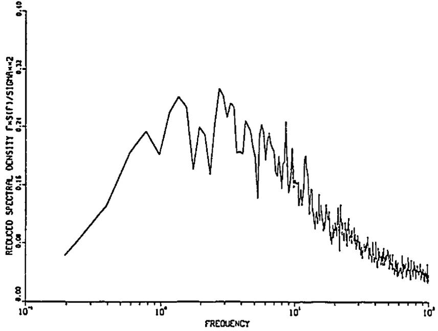
Fig. (7.7): Velocity spectrum for open country exposure
