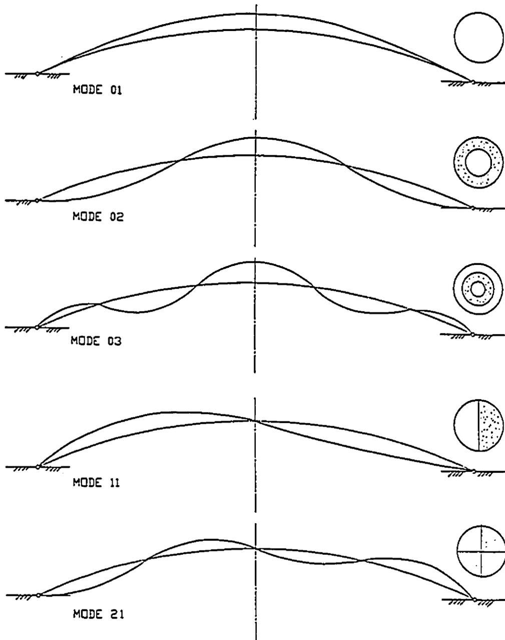
Fig. (6.16): Mode shapes of the shallow spherical air-supported structure
