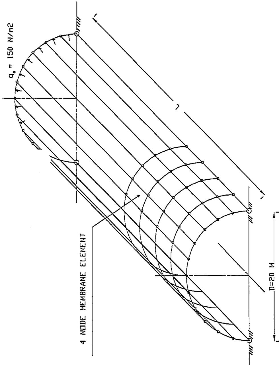
Fig. (6.10): Finite element mesh of the cylindrical air-supported structure with variable  $L/D$  (4 node element, S4R)
