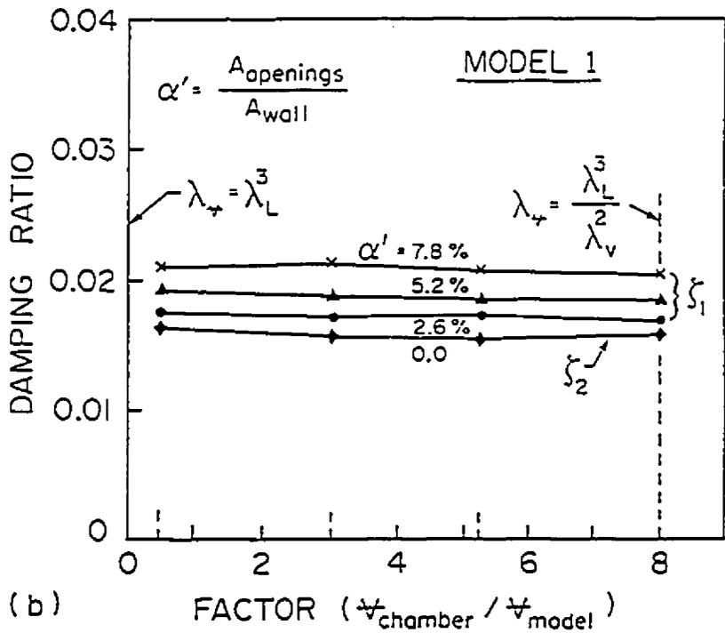
Fig. (4.9): Effect of cavity volume on (a) fundamental frequencies and (b) damping ratios of fundamental modes of the membrane roof
