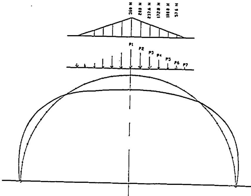
Fig. (6.7): Displaced shape of the cylindrical air-supported structure under snow load
