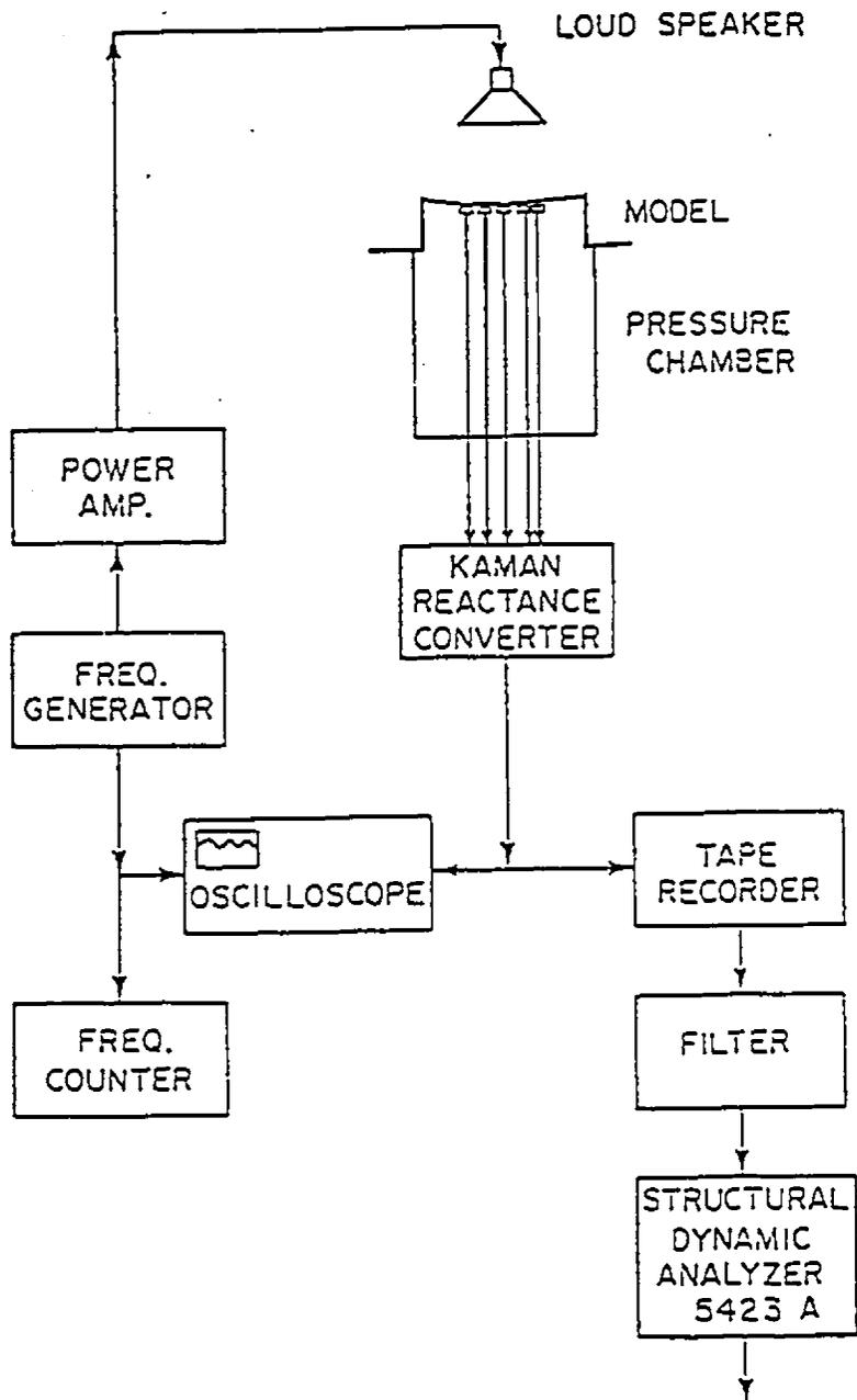
Fig. (4.5): Free vibration experimental set-up
