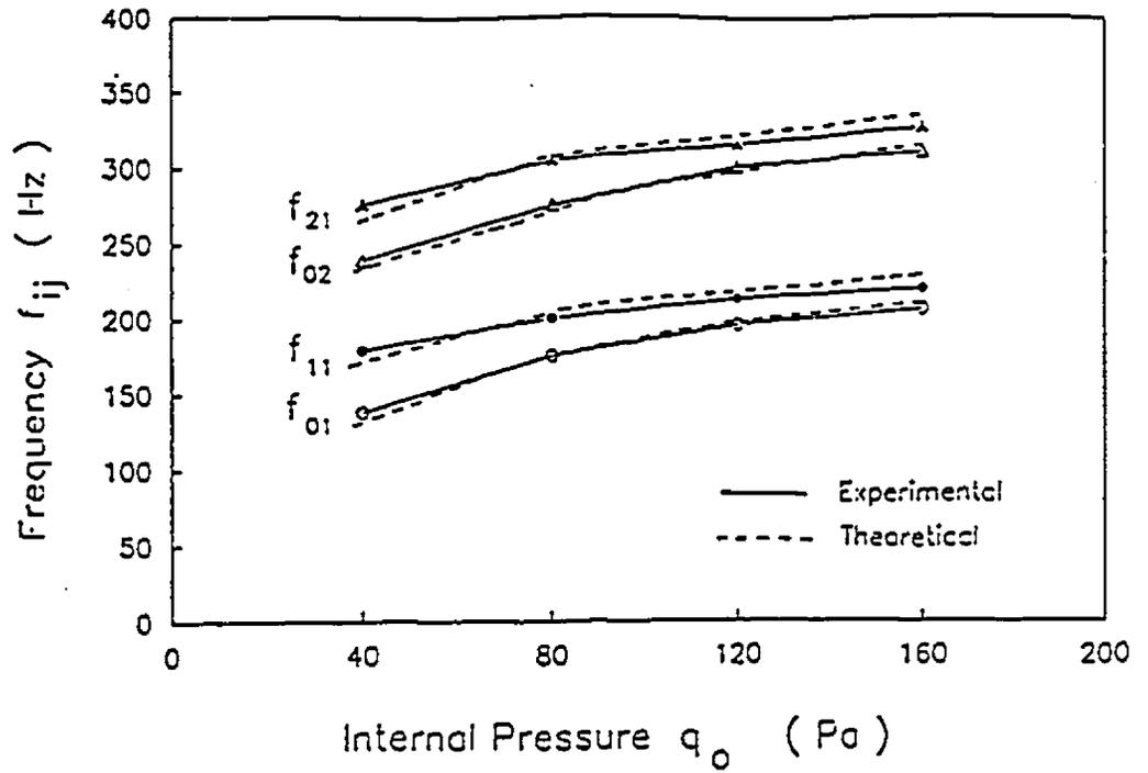
Fig. (7.4) : Effect of internal pressure on frequencies of free vibration
