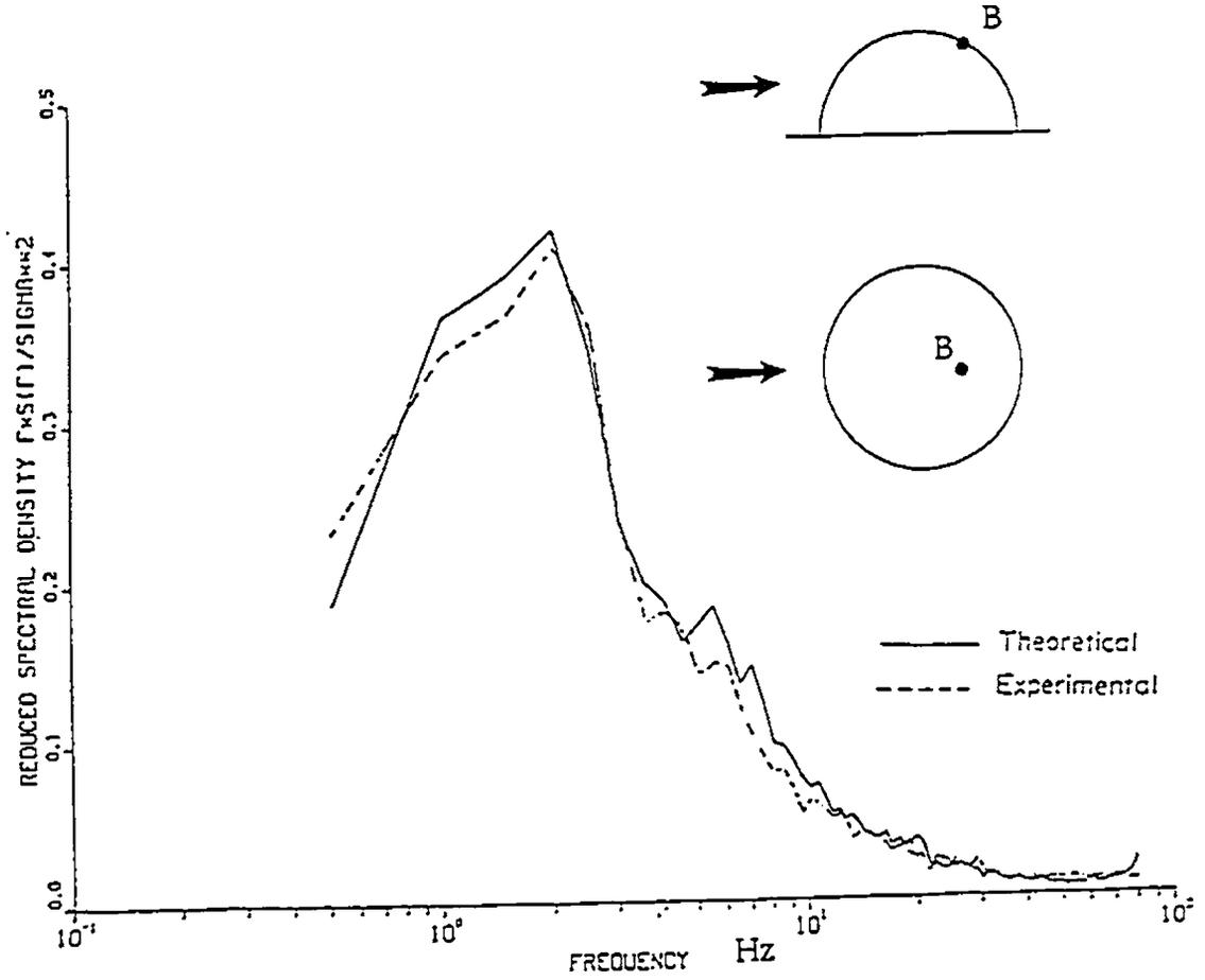
Fig. (8.12): Predicted and measured response spectra at point B (suburban exposure,  $q_0 = 40 \text{ Pa}$ )
