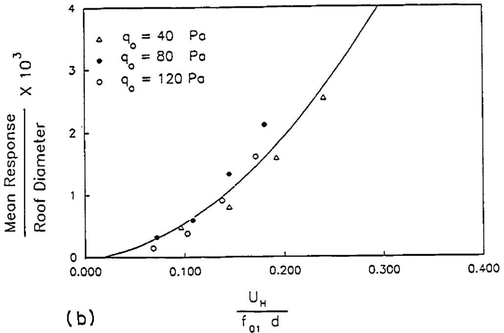
Fig. (7.19) : Mean response at roof center for different internal pressures (open country exposure)
