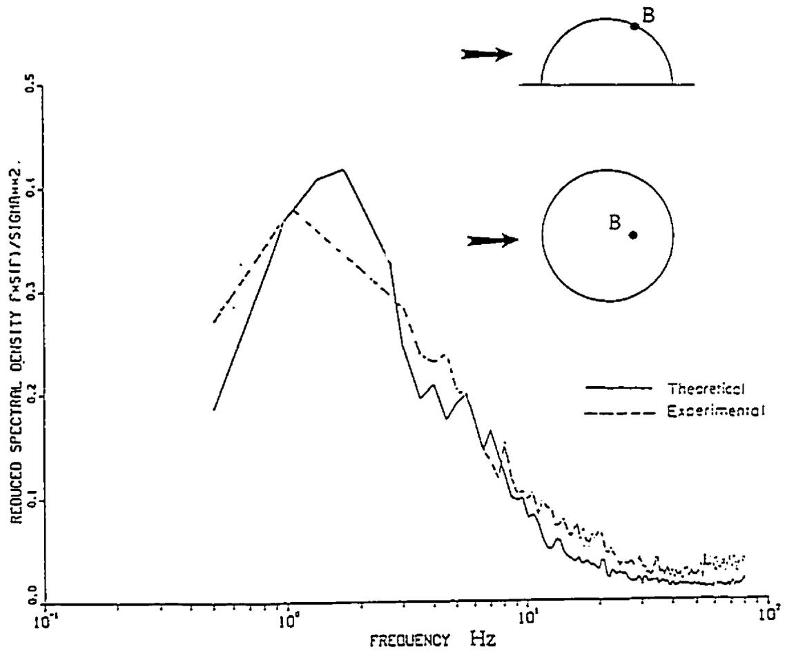
Fig. (8.13): Predicted and measured response spectra at point B
