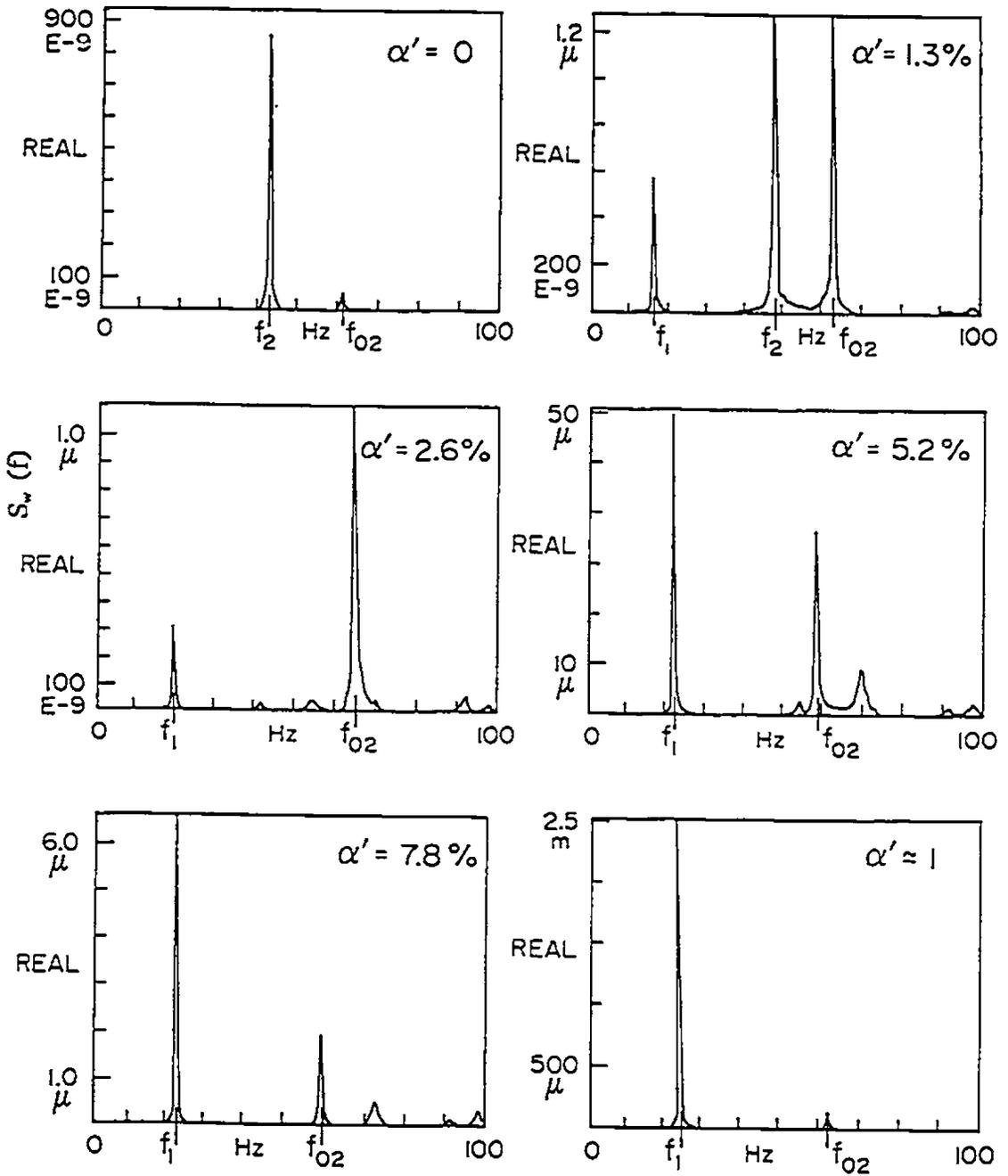
Fig. (4.6): Power spectra of response of the membrane roof to a white noise excitation
