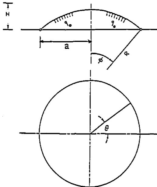
Fig. (6.12): A shallow spherical air-supported structure
