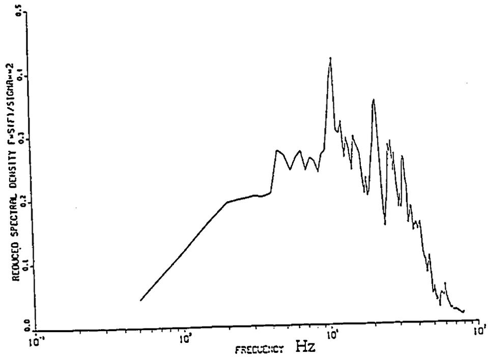
Fig. (7.21) : Power spectrum of internal pressure (open country exposure,  $U = 15 \text{ m/sec}$ , and  $q_0 = 40 \text{ Pa}$ )
