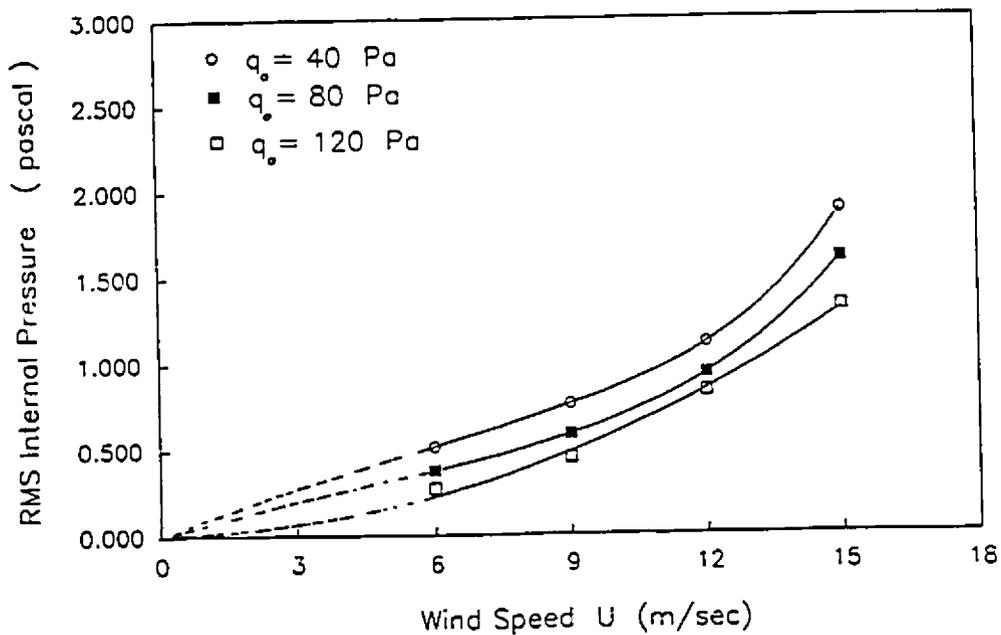
Fig. (7.24) : RMS internal pressure for different internal pressures (open country exposure)
