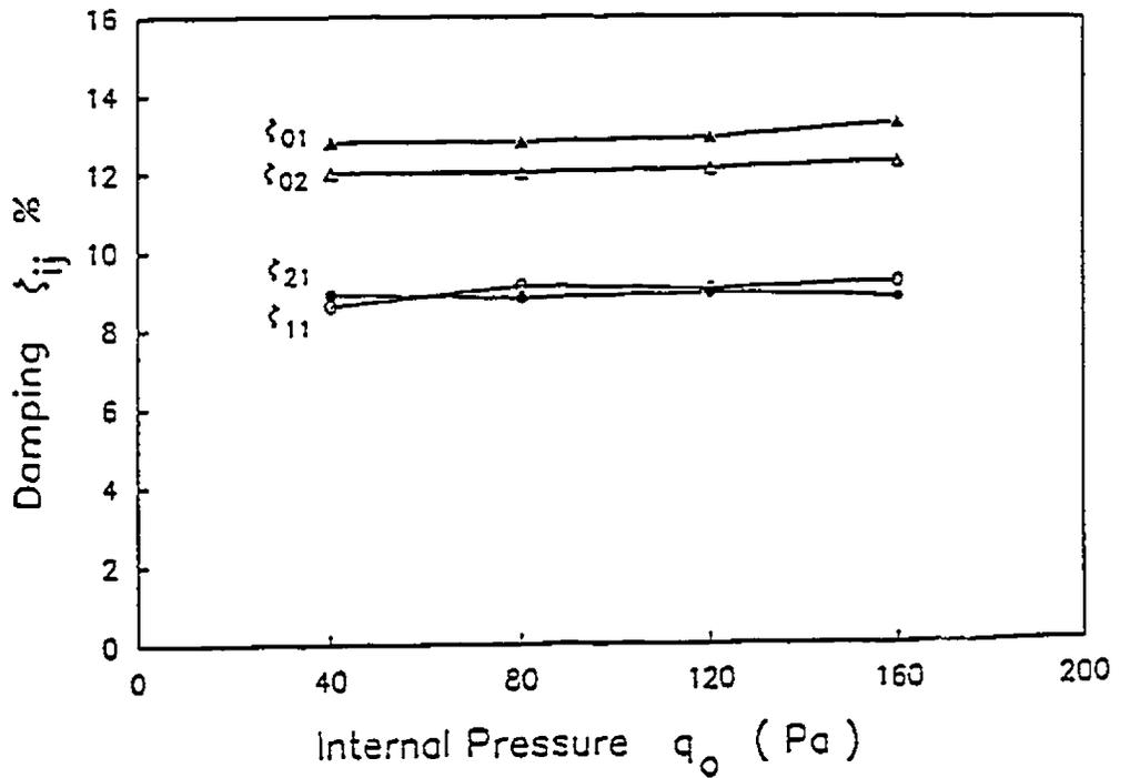
Fig. (7.5) : Effect of internal pressure on damping of free vibration
