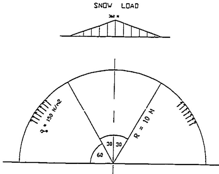
Fig. (6.6): The cylindrical air-supported structure under snow load
