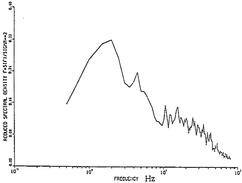
Fig. (A.1): Power spectrum of response at roof center (suburban exposure,  $U = 15$  m/sec, and  $q_0 = 40$  Pa)
