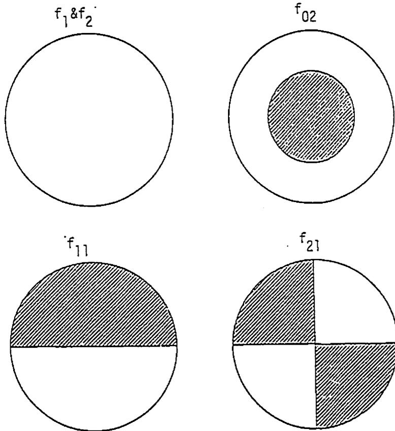
Fig. (4.4): Kaman displacement sensors arrangement and mode shapes
