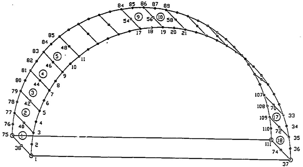
Fig. (6.5): Finite element mesh of the cylindrical air-supported structure (8 node element, S8R)
