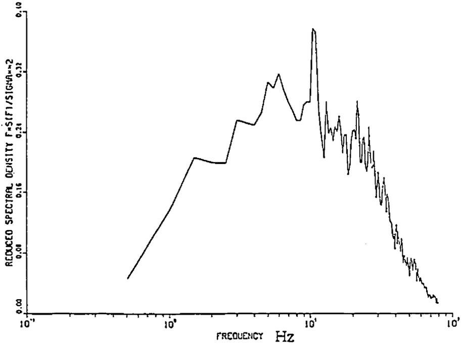
Fig. (A.6): Power spectrum of internal pressure (urban exposure,  $U = 15$  m/sec, and  $q_0 = 40$  Pa)
