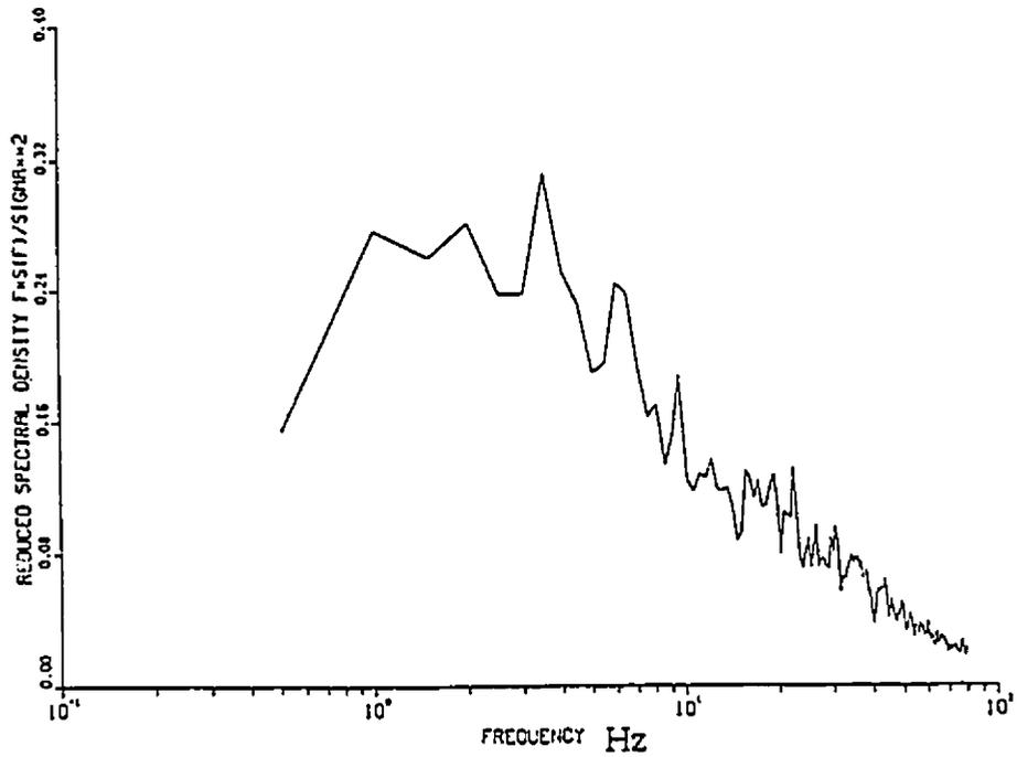
Fig. (A.3): Power spectrum of response at probe 2 (suburban exposure,  $U = 15$  m/sec, and  $q_o = 40$  Pa)
