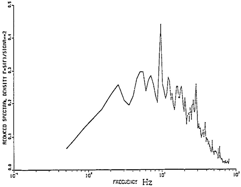
Fig. (7.22) : Power spectrum of internal pressure (open country exposure,  $U = 15$  m/sec, and  $q_0 = 80$  Pa)
