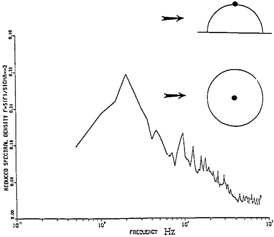
Fig. (7.16): Power spectrum of response at roof center
