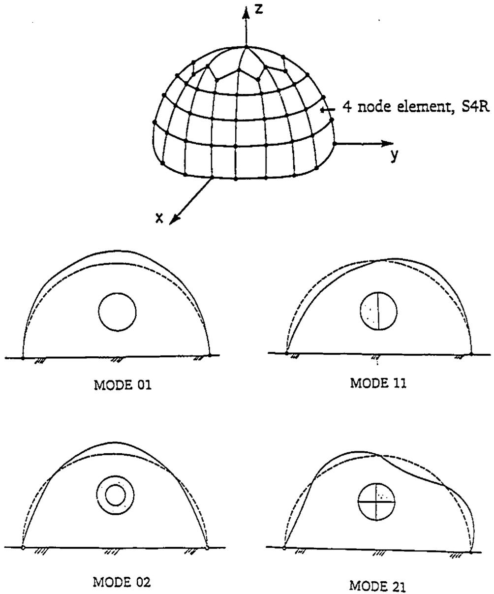
Fig. (7.3): Mode shapes of the hemispherical air-supported structure
