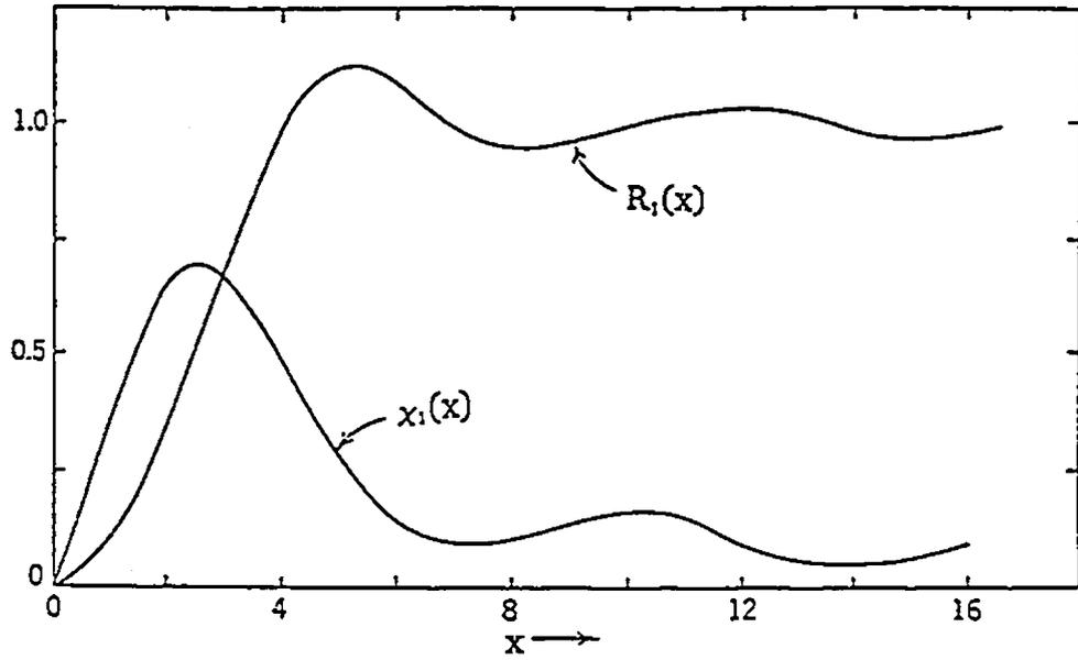
Fig. (2.1): Functions  $R_1(x)$  and  $x_1(x)$  Piston impedance functions
