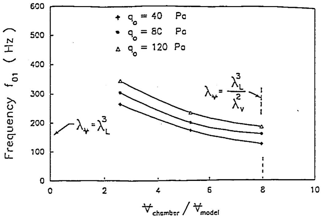
Fig. (7.6) : Effect of cavity volume on fundamental frequency of the hemispherical model
