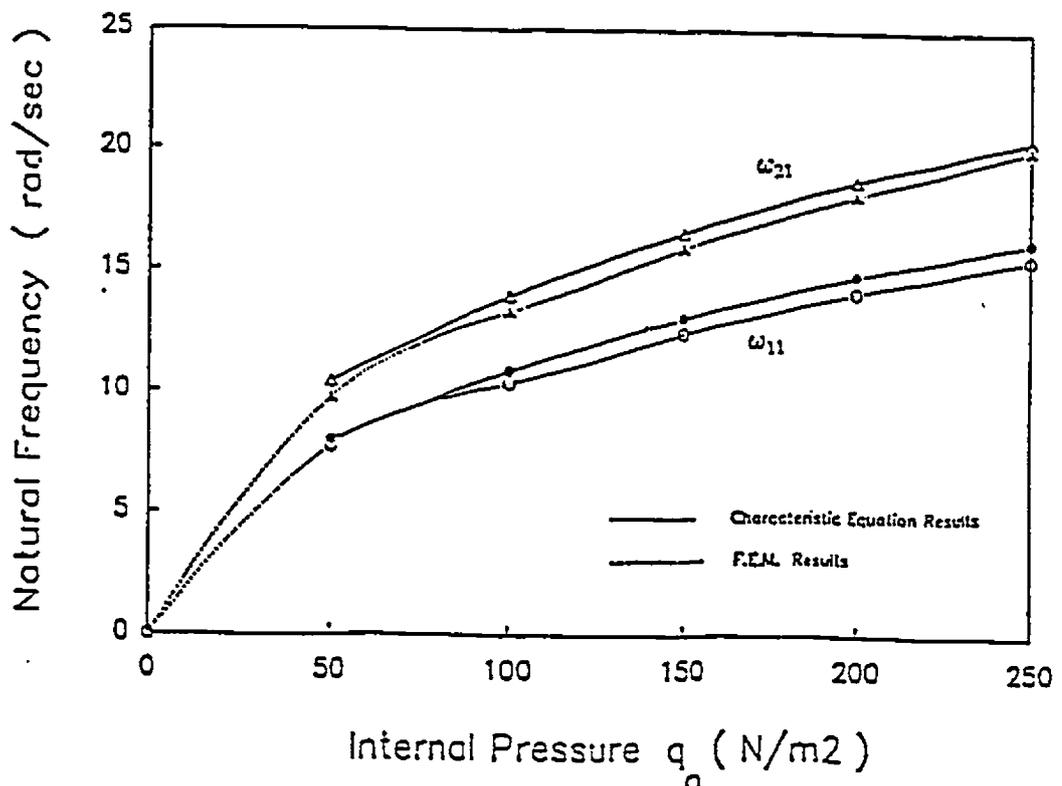
Fig. (6.15b): Internal pressure effect on frequencies of the shallow spherical air-supported structure (antisymmetrical modes)
