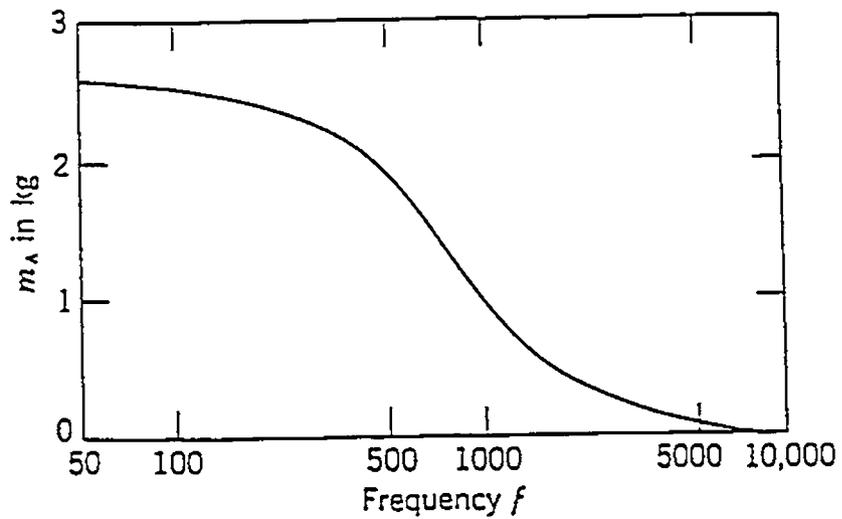
Fig. (2.2): Added mass of a vibrating piston radiating into water
