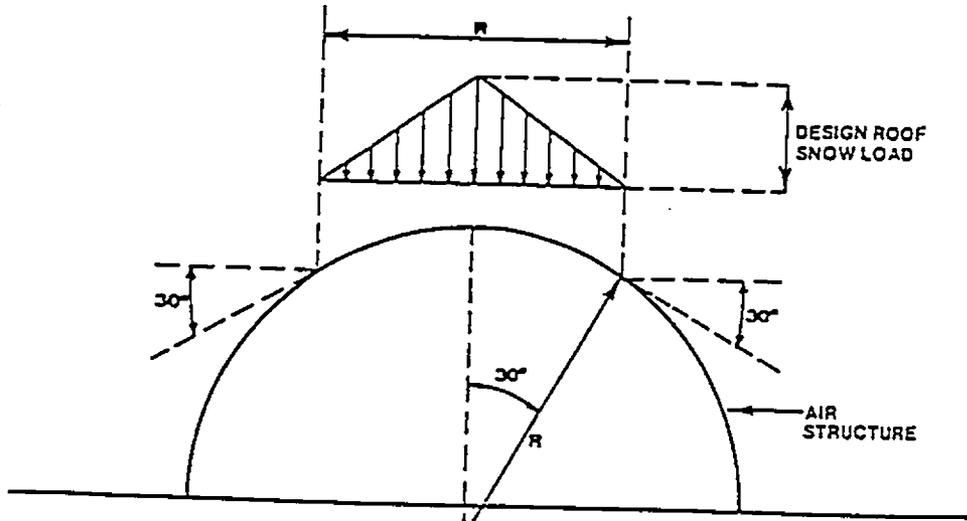
Fig. (5.2): Standard snow load on air-supported structures (AFSI, 1977)
