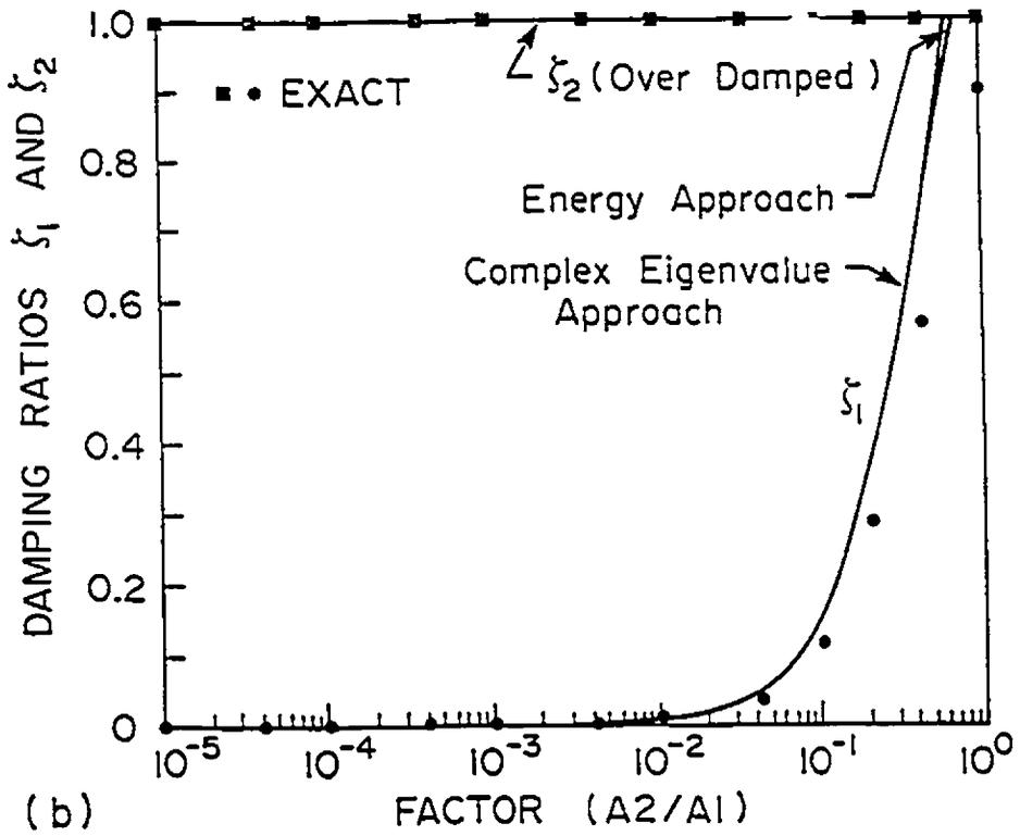
Fig. (3.4): Leakage effect on roof total damping: (a) the simplified Calgary Olympic Coliseum roof and (b) the lighter roof
