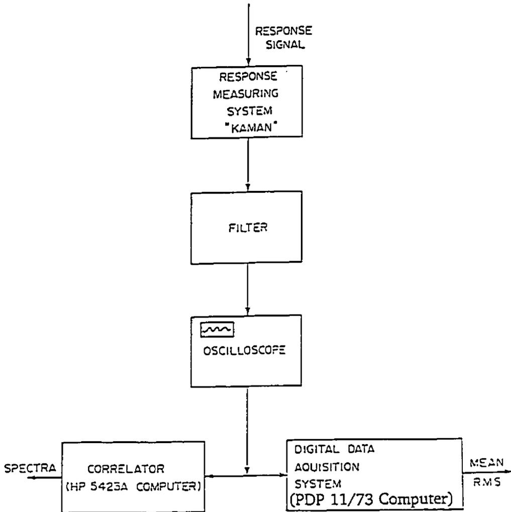
Fig. (7.13): Wind tunnel experimental set-up
