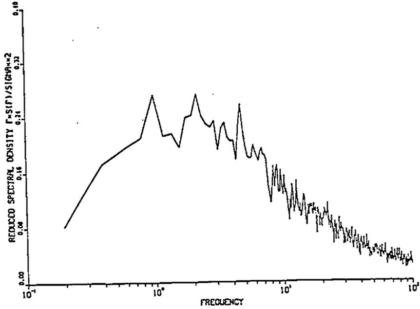
Fig. (7.9): Velocity spectrum for suburban exposure
