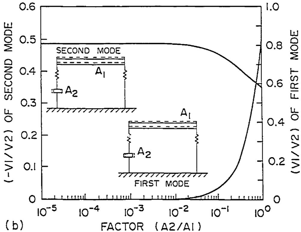
Fig. (3.2): Leakage effect on roof undamped vibration modes: (a) the simplified Calypso Olympic Coliseum roof and (b) the lighter roof
