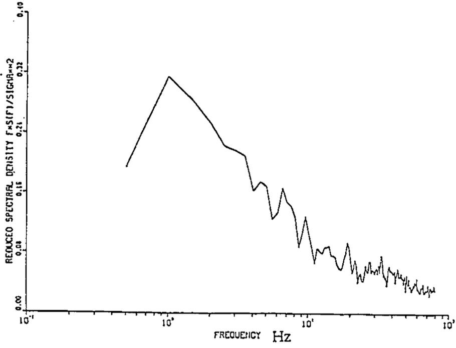
Fig. (A.2): Power spectrum of response at roof center (urban exposure,  $U = 15$  m/sec, and  $q_0 = 40$  Pa)
