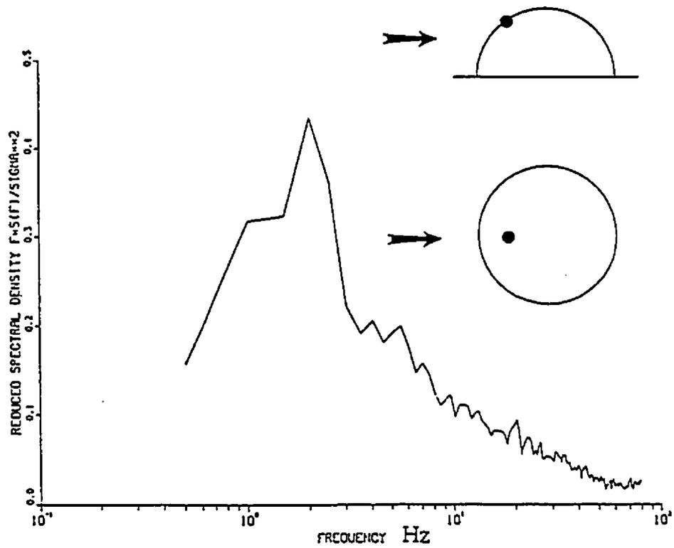
Fig. (7.17) : Power spectrum of response at probe 2 (open country exposure,  $U = 15$  m/sec, and  $q_0 = 40$  Pa)
