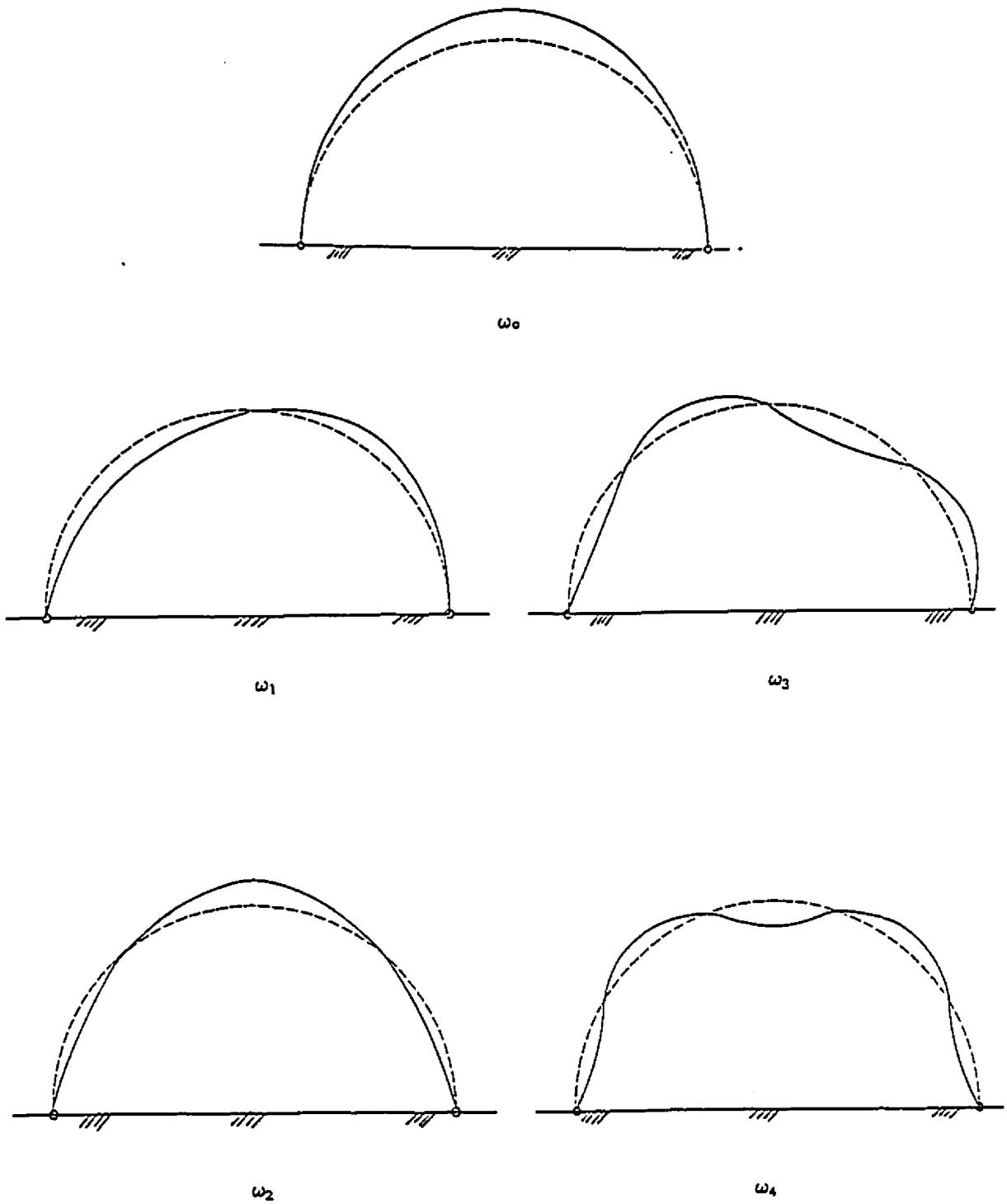
Fig. (6.9): Mode shapes of the cylindrical air-supported structure
