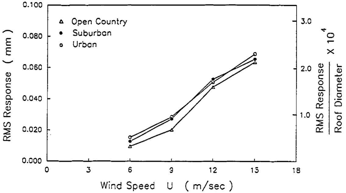
Fig. (7.15) : RMS response at roof center for different exposures ( $q_s = 40 \text{ Pa}$ )
