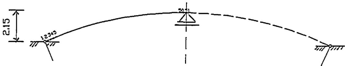
Fig. (6.14): Finite element mesh of the shallow spherical air-supported structure (antisymmetrical modes)
