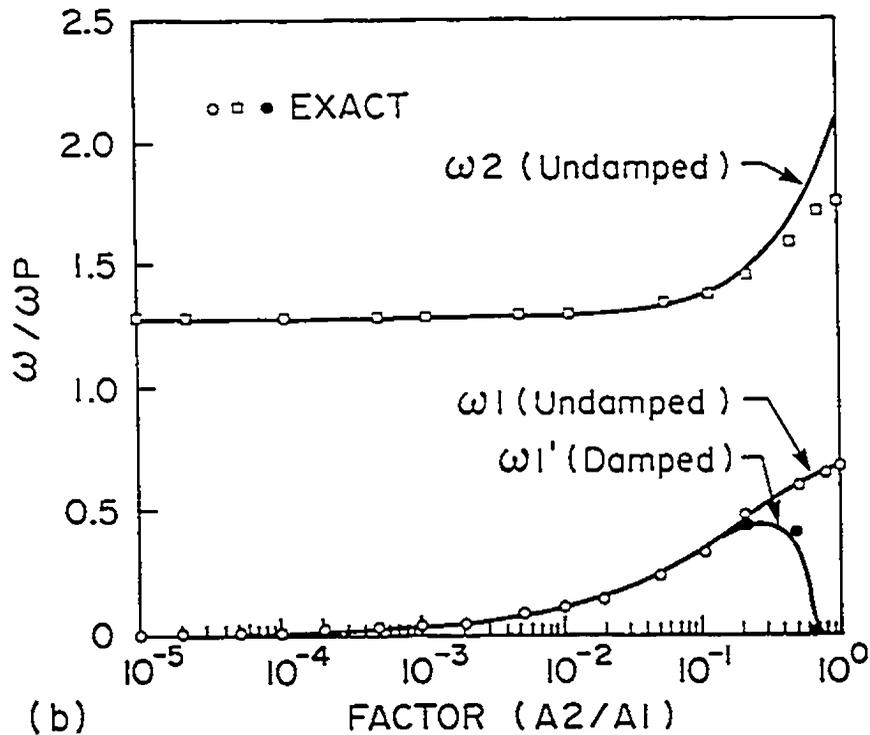
Fig. (3.3): Leakage effect on roof fundamental frequencies: (a) the simplified Calgary Olympic Coliseum roof and (b) the lighter roof
