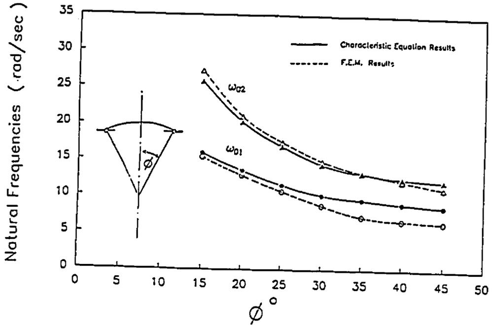
Fig. (6.17a): Comparison of the analytical and FEM results of the shallow spherical air-supported structure (axisymmetrical modes)
