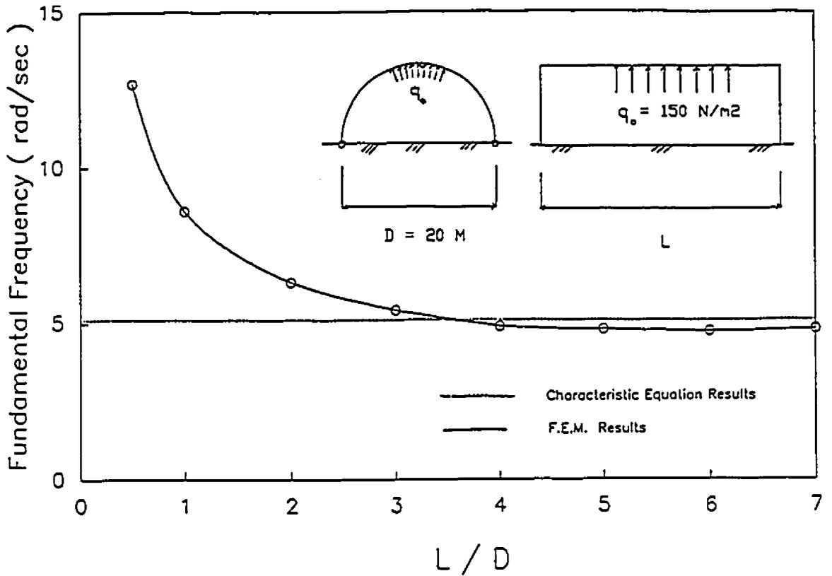
Fig. (6.11): Effect of varying the L/D ratio on the fundamental frequency of the cylindrical air-supported structure
