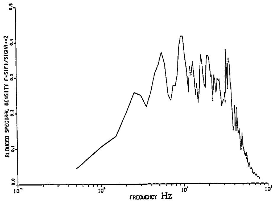
Fig. (A.5): Power spectrum of internal pressure (suburban exposure,  $U = 15$  m/sec, and  $q_0 = 40$  Pa)
