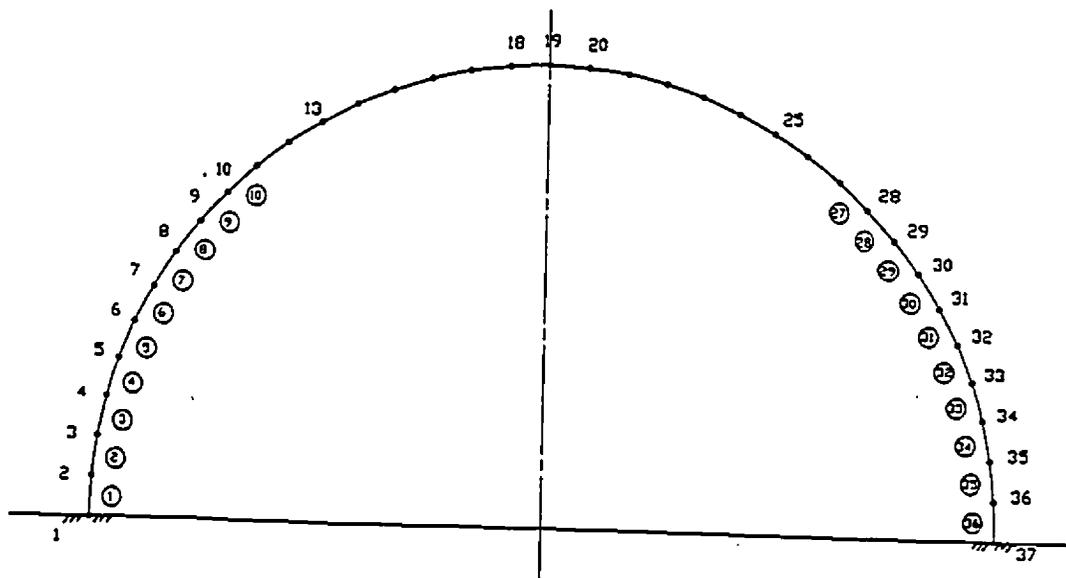
Fig. (6.4): Finite element mesh of the cylindrical air-supported structure (2 node element, B23)
