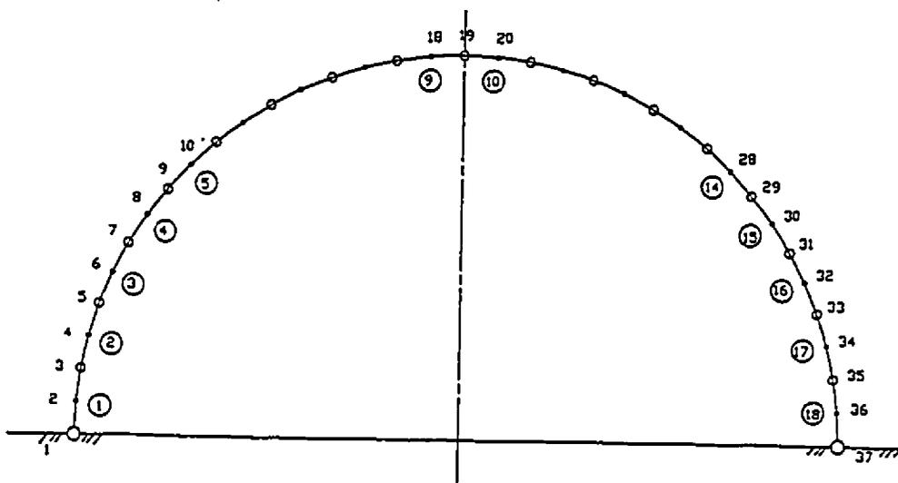
Fig. (6.3): Finite element mesh of the cylindrical air-supported structure (3 node element, B22)
