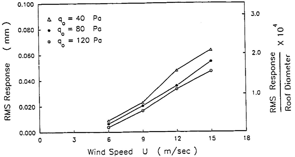
Fig. (7.20) : RMS response at roof center for different internal pressures (open country exposure)
