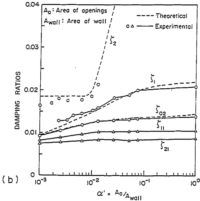
Fig. (4.7): Effect of wall openings on (a) frequencies and (b) damping ratios of the membrane roof.
