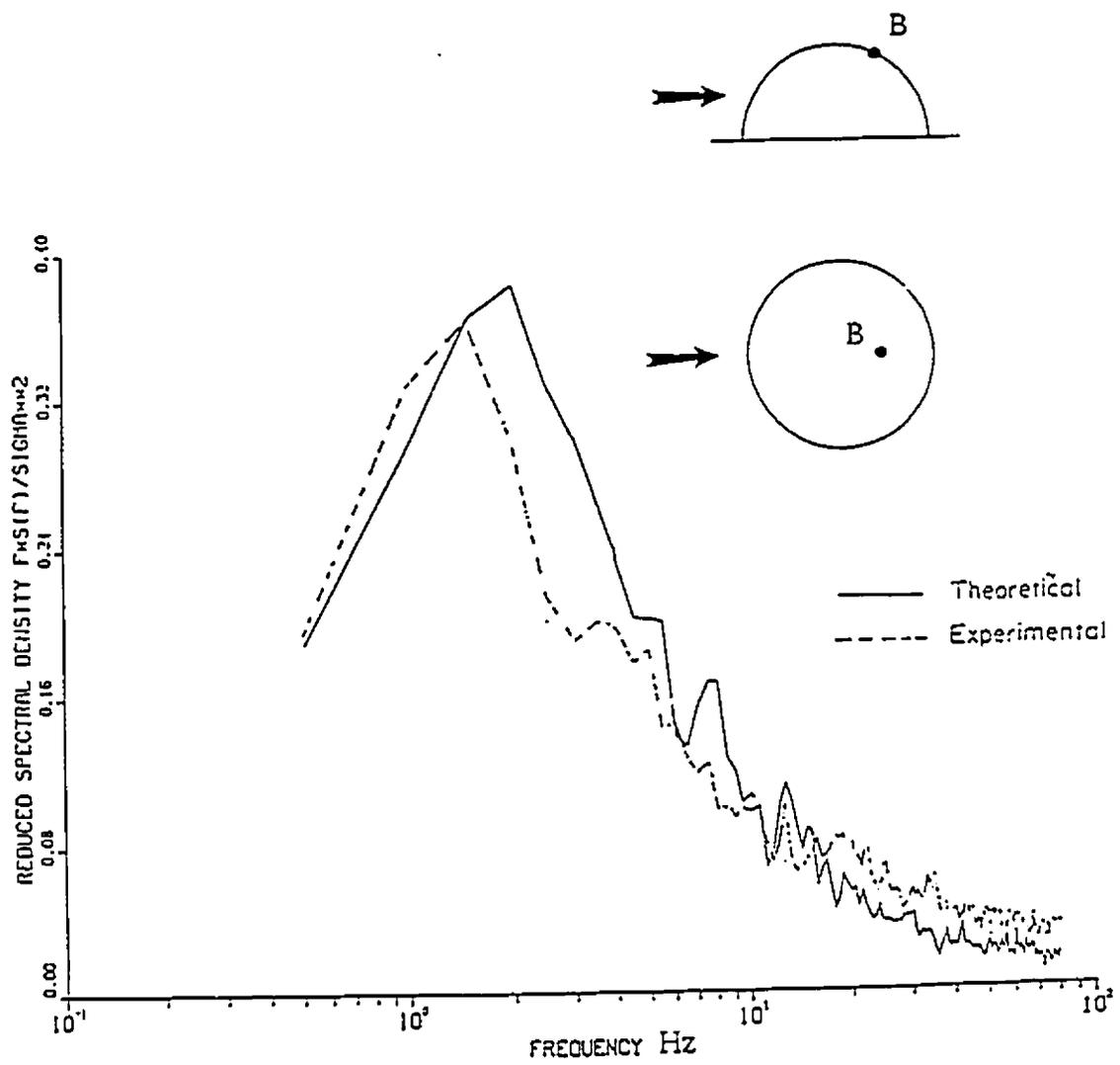
Fig. (8.11): Predicted and measured response spectra at point B (open country exposure,  $q_0 = 40$  Pa)
