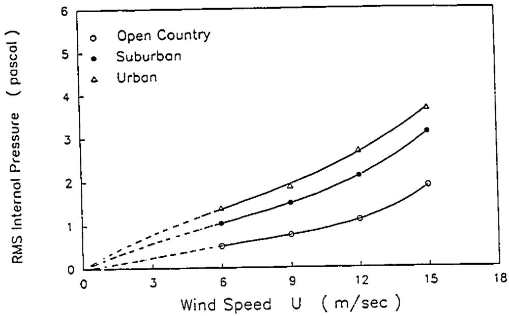
Fig. (7.23) : RMS internal pressure for different exposures ( $q_o = 40$  Pa)
