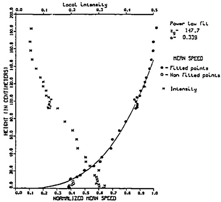
Fig. (7.12): Velocity profile for urban exposure
