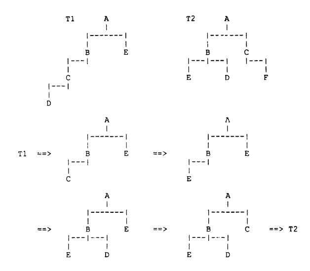
Given  $C_I = C_D = 1$ , the transformation cost or the distance is 7 for this example. The similarity of these two trees can be calculated by
