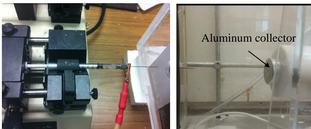
Figure 18: Horizontal coaxial electrospinning configuration
