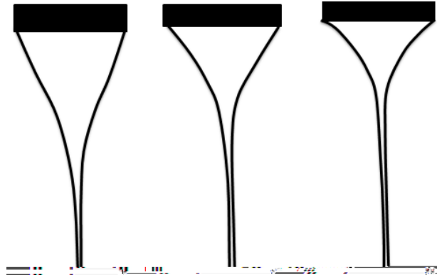
Figure 1: Glycerol jets profile at 0.5mL/min. Left to right: 3.67kV/cm, 4.33kV, 5.0kV/cm (adapted from [18])
