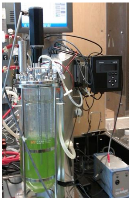
Figure 3-1: Labfors 5 bioreactor for large volume cultivation
