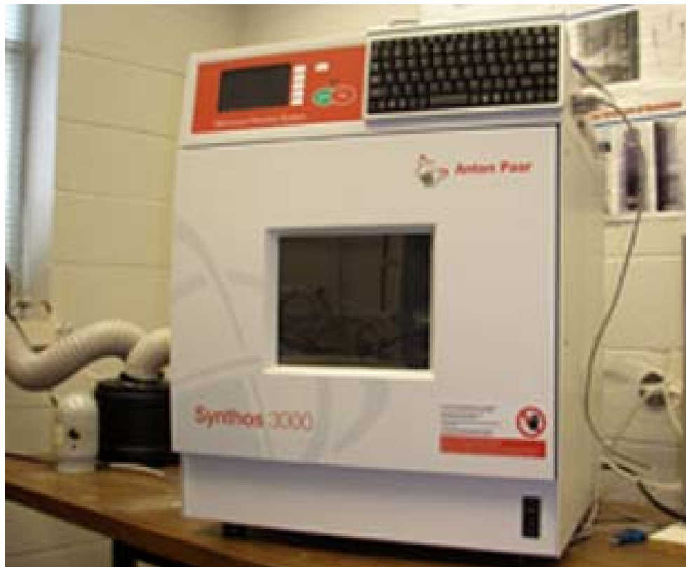
Figure 2.2 A photo of an Anton Paar Synthos 3000 microwave synthesis system in our lab.
