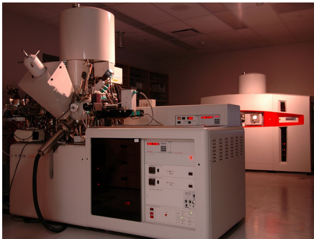
Figure 2.6 A photo of a Kratos Axis Ultra X-ray photoelectron spectrometer [15].
