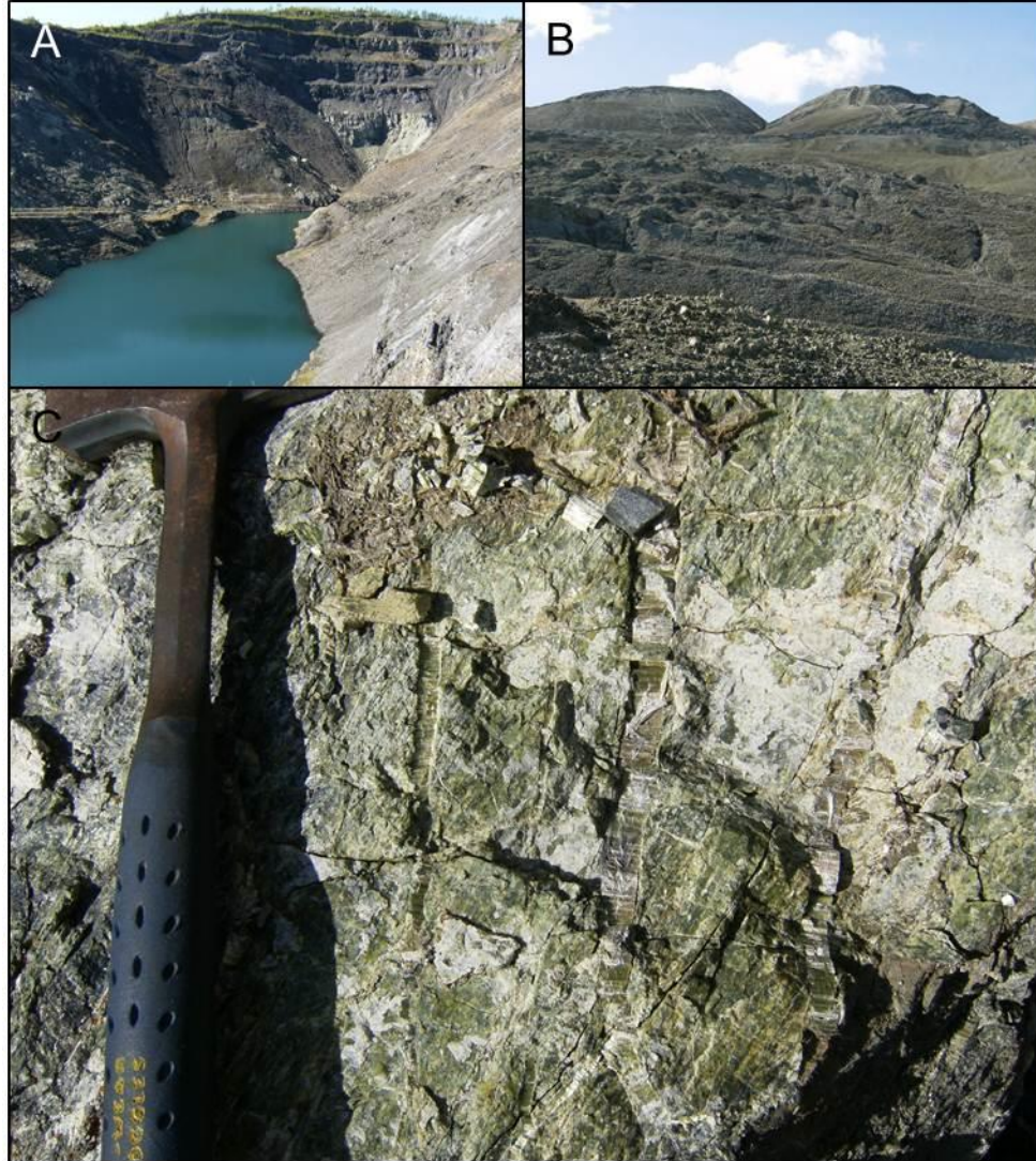
Figure 3.2 A) The Porcupine open pit and B) tailings pile at Clinton Creek Mine, Yukon, Canada. C) Veins of chrysotile fibres cutting through the serpentine wall rock at Clinton Creek.
