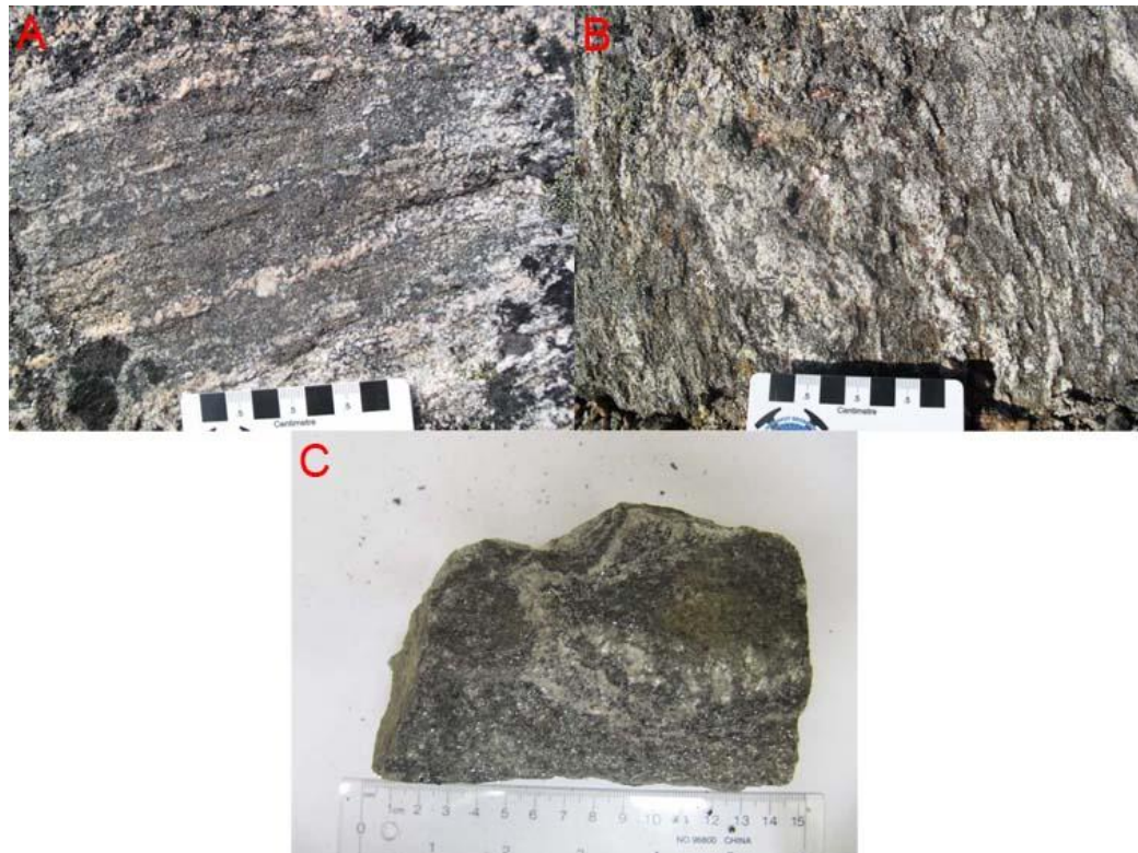
Figure 4.16 A: Field photo of sample 10645 showing the strong foliation and leucocratic pockets of quartzo-feldspathic composition. B: Field photo showing a group of leucocratic quartzo-feldspathic lenses rich in garnet. C: Hand sample photo, G067A1.
