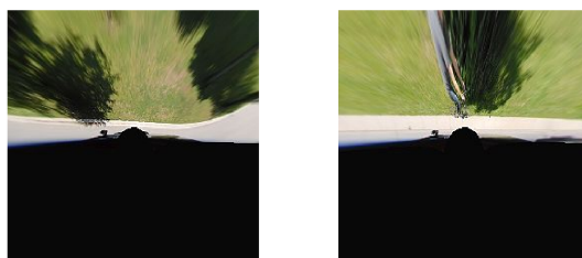
Figure 6.6: Image selection algorithm may fail, due to shadows that generate road-like features.
