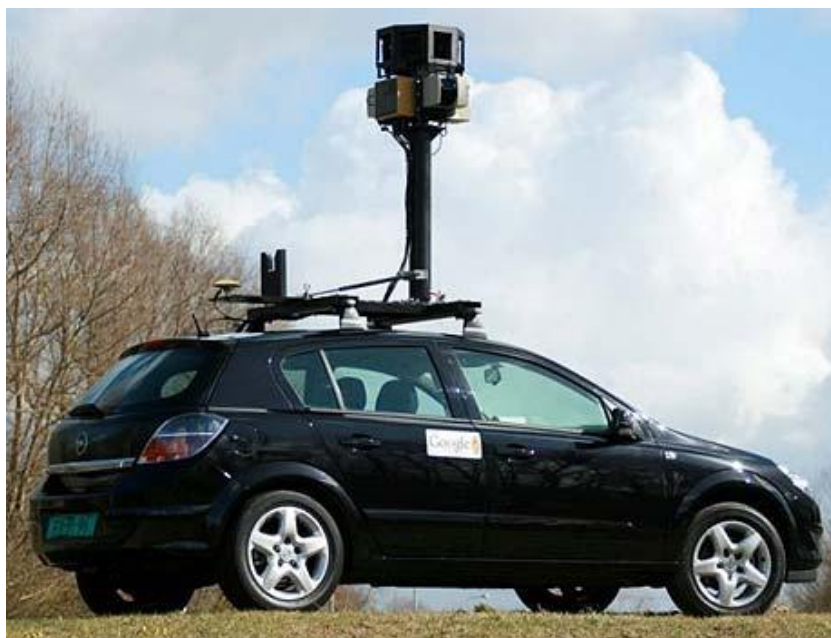
Figure 1.3: Street-level imaging car (Image courtesy of Telegraph website 4 )
