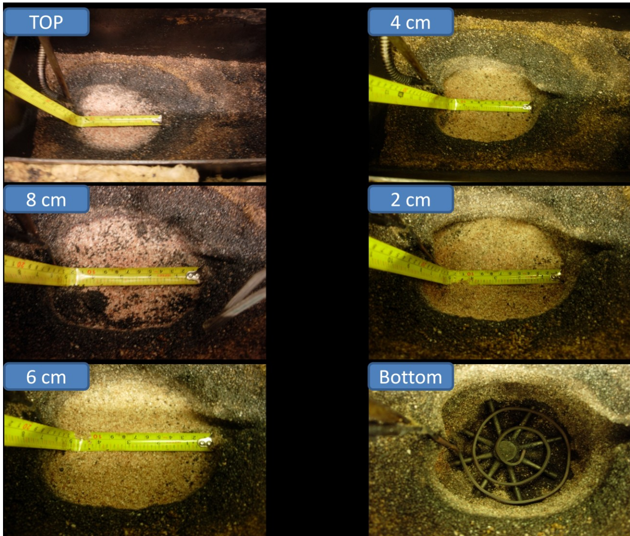
Figure M4: Post-mortem of the 50 L/min experiment. Figure from top left to right bottom represent the height from top to bottom. Horizontal spreading was measured at the center of the box across the heater.
