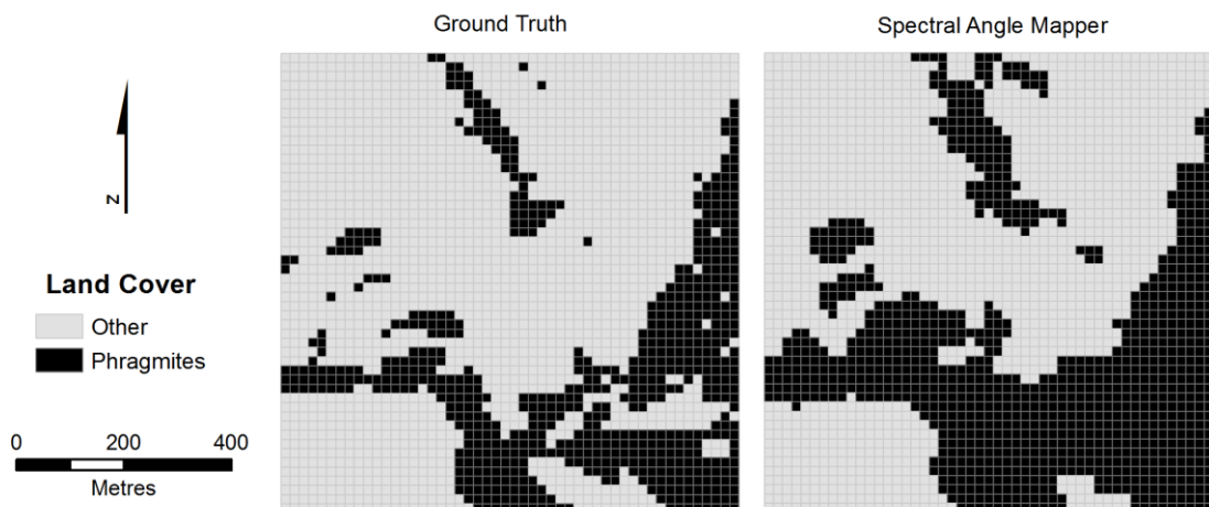
Figure 3.16 Spectral angle mapper (SAM) classification of Phragmites and Other land cover class map.
