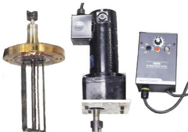
**Figure 4.2** Mechanical stirrer used in the fluidized bed
