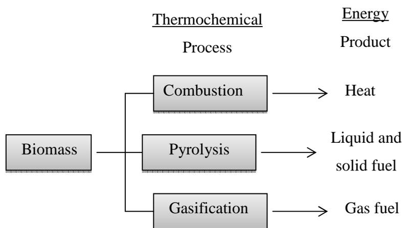
Figure 1-1. Biomass Thermochemical Conversion Processes and Products (14)
