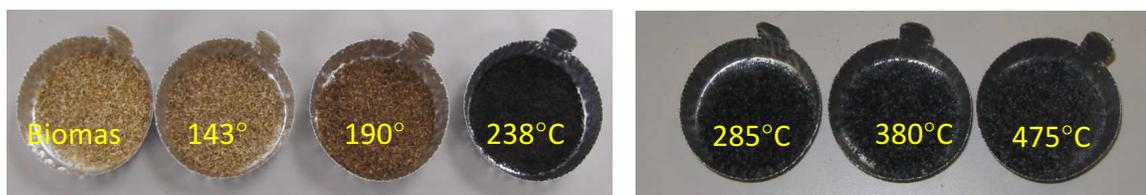
Figure 2-8. Bio-coal products at the various temperatures studied
