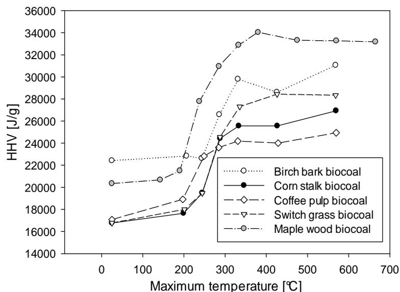
Figure 4-6 Biomass and Bio-coal High Heating Values for Different Biomasses
