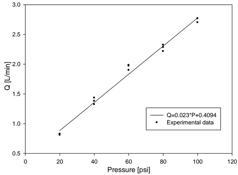
Figure 6-2. Nitrogen flow calibration through pressure regulator
