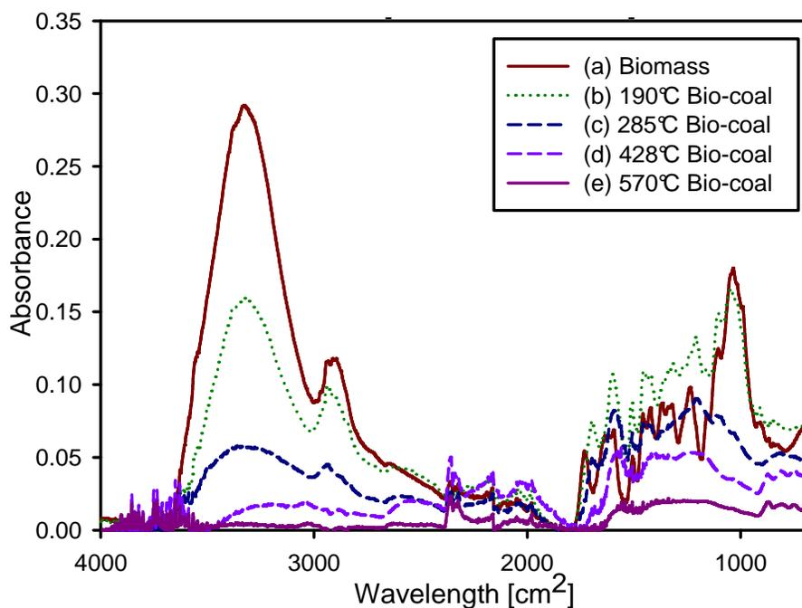
Figure 2-15. FTIR spectra for (a) feedstock biomass; and bio-coals produced at reaction temperatures of (b) 190 °C, (c) 285 °C, (d) 428 °C and (e) 570 °C
