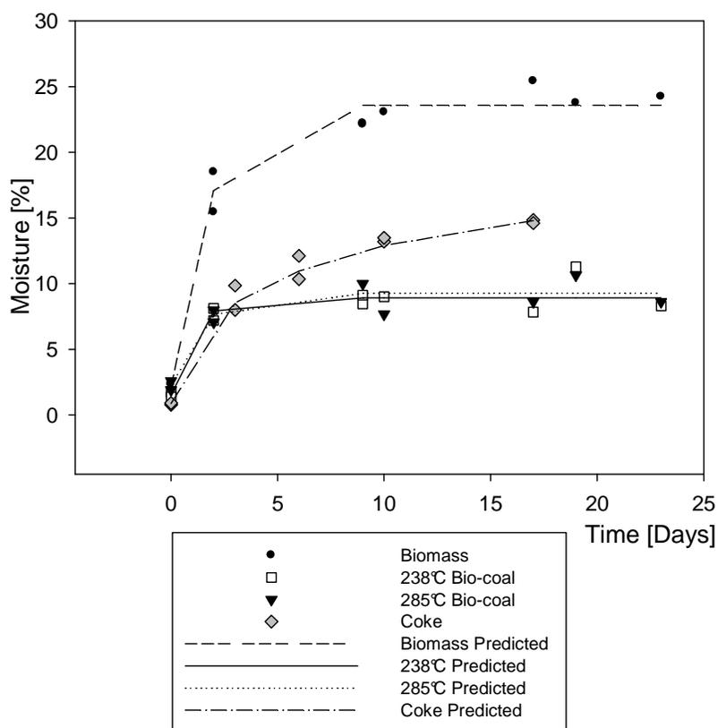
Figure 2-16. Hygrosopy of biomass, torrefied bio-coals and coke, reported in units of moisture at different tested times
