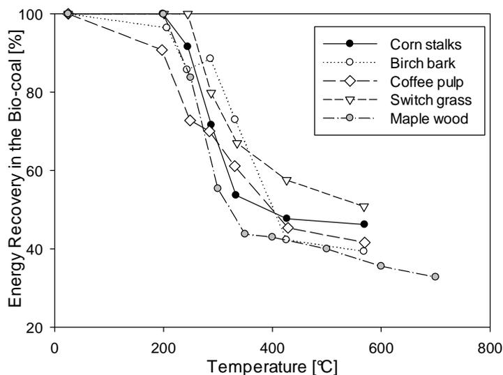
Figure 4-7 Percentage of Energy Recovery in Bio-coal from Different Biomasses
