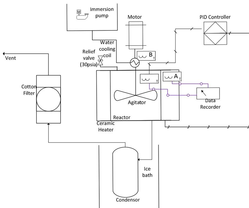
Figure 2-2. Detailed schematic of the MFR reactor
