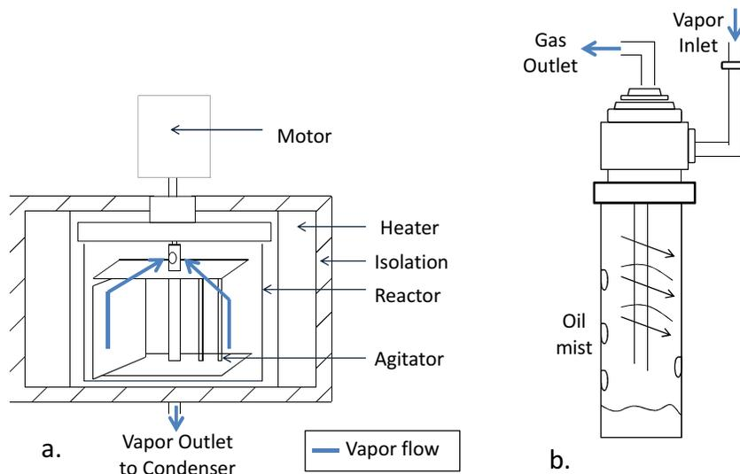
Figure 2-1. (a) MFR Reactor; (b) Condenser
