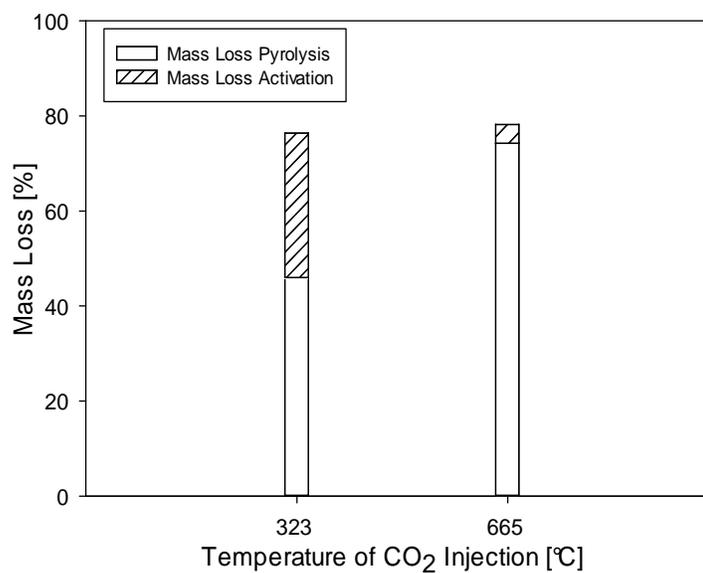
Figure 3-14. Overall Mass Loss during Pyrolysis and Activation with CO<sub>2</sub> Injection Points at different Temperatures (Figure 3-13)
