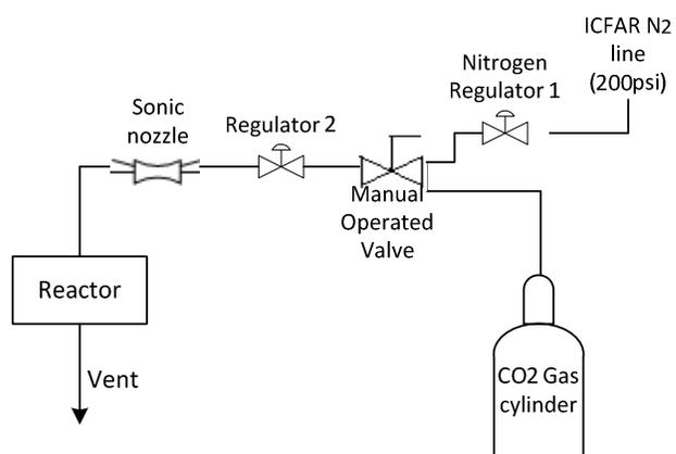
Figure 6-1. Gas Flow Diagram
