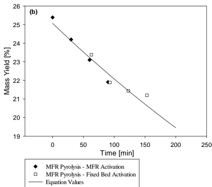
Figure 3-11. (a) Activated Carbon Mass Yield from a Consecutive Pyrolysis - Activation in the MFR (Figure 3-6) and pyrolysis in the MFR with Activation in the Fixed Bed (Error! Reference source not found.) (Activation Temperature: 665 °C, CO<sub>2</sub> injection 0.59 L/min, holding times during activation of: 30min, 1h, 1h:30min) (b) Activated Carbon Mass Yield Presenting all data from Figure 3-11(a), Shifting Time on the x-axis for the Fixed Bed Activation
