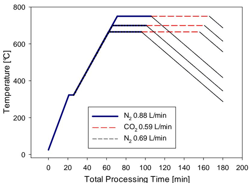
Figure 3-15. Pyrolysis and Activation Experiments Description at Different Temperatures (Fixed Bed Reactor, activation holding time 1h, injection 0.59 L/min )
