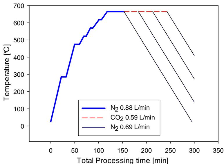
Figure 3-6. Temperature history for the consecutive Pyrolysis – Activation Experiments at 665°C carried out in the MFR (holding times during activation of: 30min, 1h, 1h:30min, , CO<sub>2</sub> injection 0.59 L/min).
