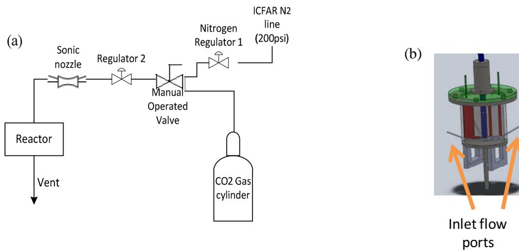
Figure 3-2. Detail of the MFR flow feeding system
