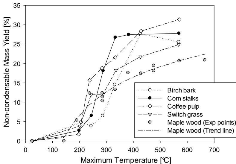
Figure 4-5. Non-condensable Gases Mass Yield from Different Biomasses
