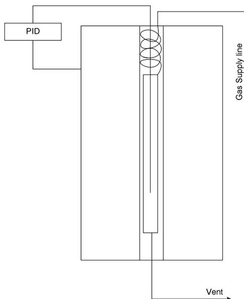
Figure 4-2. Fixed bed reactor in a tubular furnace (1093 °C, 110V, 8 Amp)
