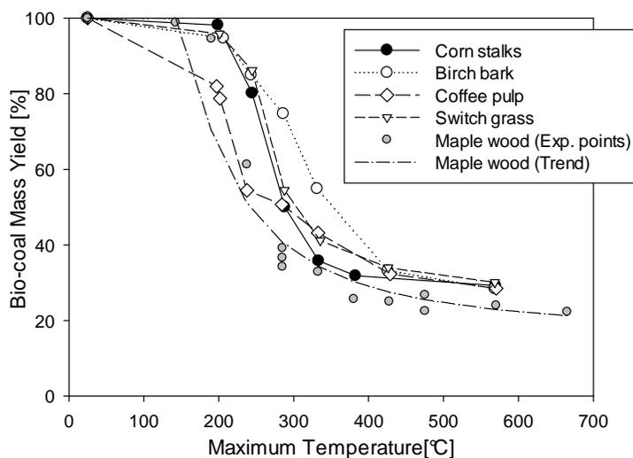
Figure 4-3 Bio-coal Mass Yields from Different Biomasses
