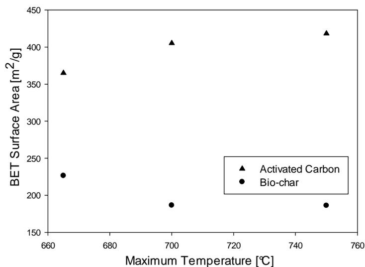
Figure 3-16. Activated carbons and bio-chars surface areas at different temperatures (Pyrolysis; maximum temperature holding time: 30 min, Activation; 1 h holding time at maximum temperature, 0.059 L/min CO<sub>2</sub>, Figure 3-15)
