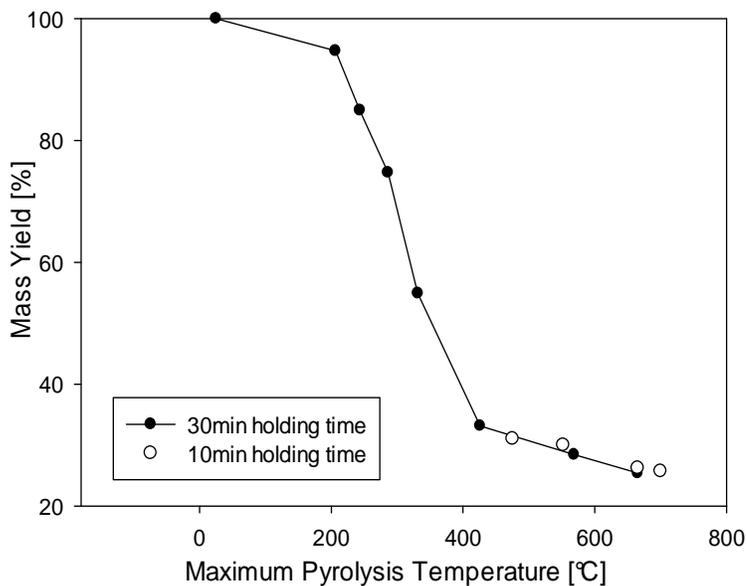
Figure 3-9. Bio-char Mass Yields at Different Maximum Process Temperatures in the MFR (Biomass load:100 g, Holding Time at a Maximum Temperature: 10 or 30 min, Agitator velocity: 49.5 rpm)
