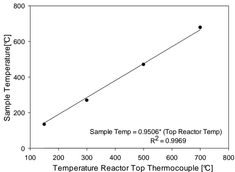
Figure 2-3. Relationship between the sample temperature and the thermocouple reading at the top of the reactor
