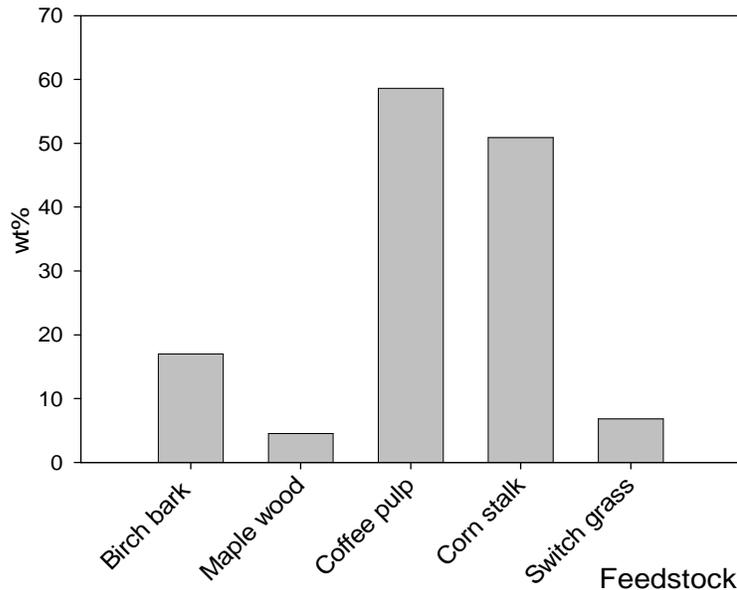
Figure 4-16. Mass loss during activation for different feed biomasses
