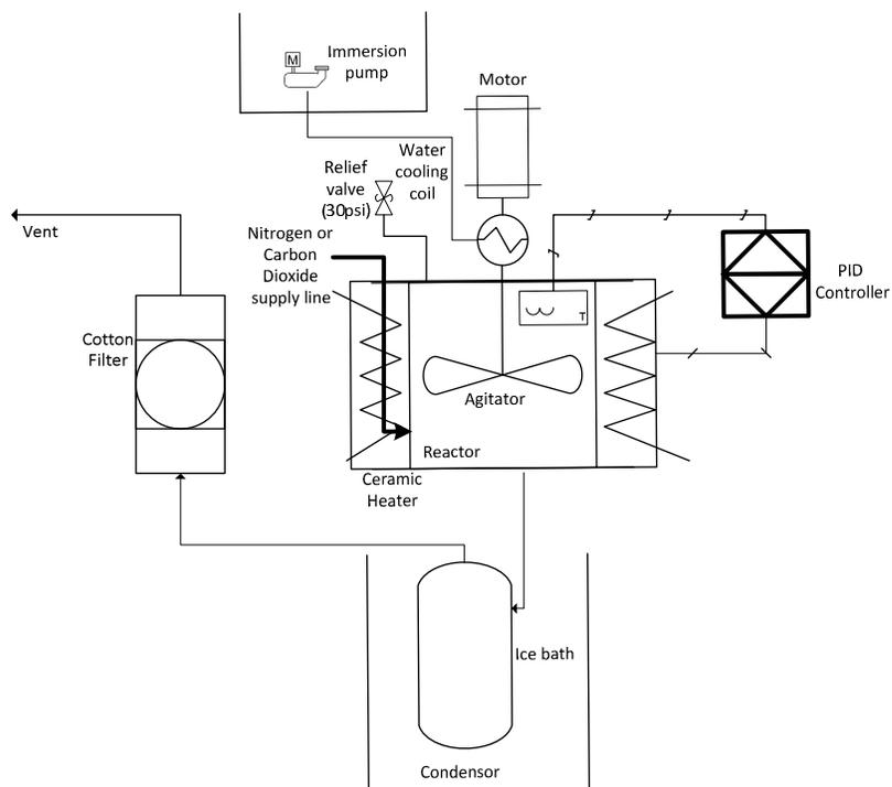
Figure 3-1. MFR; General reactor diagram
