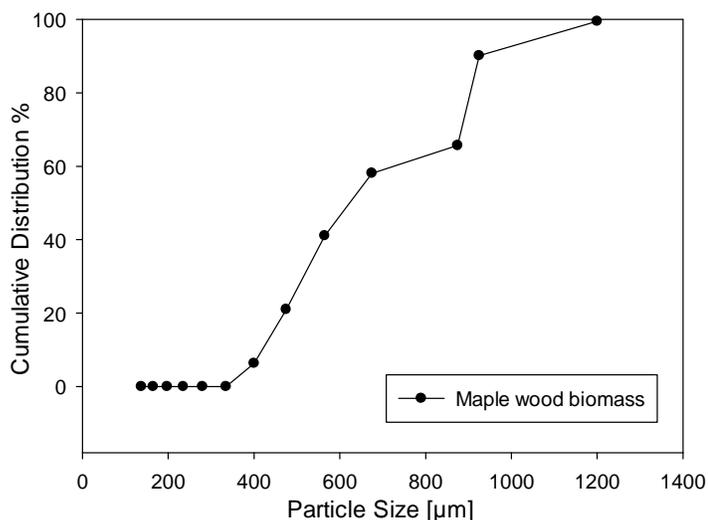
Figure 2-4. Maple wood cumulative particle size distribution as feed in the reactor
