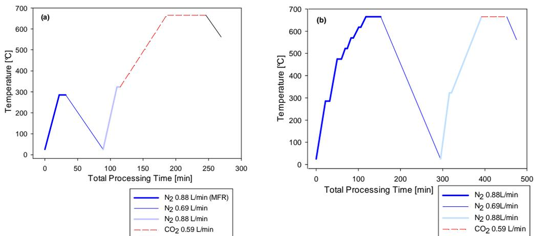
Figure 3-13. Activation Experiments Description; CO<sub>2</sub> Injection from a Low Temperature and CO<sub>2</sub> Injection only at a Maximum Process Temperature for Activation (Fixed Bed Reactor) (Maximum activation Temperature: 665 °C, CO<sub>2</sub> injection 0.59 L/min)
