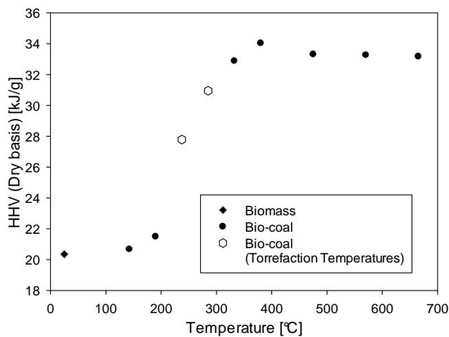
Figure 2-10. High heating values on a dry basis (biomass load = 100 g; holding time = 30 min; heating rate = 12 °C/min; agitator velocity = 49.5 rpm)
