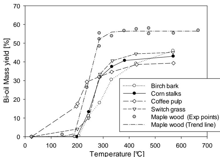
Figure 4-4 Bio-oil Mass Yields from Different Biomasses
