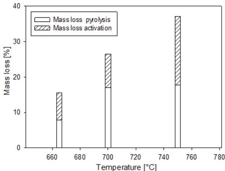
Figure 3-17. Mass loss distribution on the fixed bed reactor; during pyrolysis and activation
