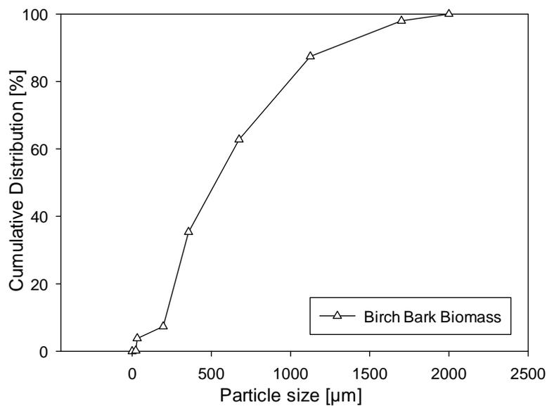
Figure 3-5. Birch bark biomass cumulative particle size distribution as feed in the reactor
