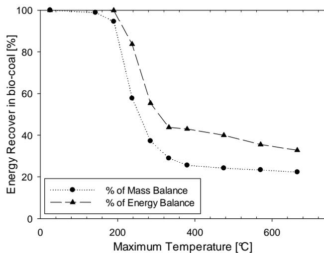
Figure 2-11. Percentage energy recovery in bio-coal (biomass load = 100 g; holding time = 30 min; heating rate = 12 °C/min; agitator velocity = 49.5 rpm)
