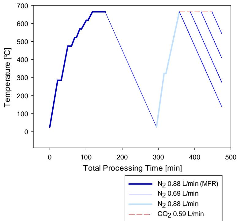
Figure 3-8. Temperature history for MFR bio-char production (with a maximum temperature of 665 °C) followed by fixed bed activation at 665 °C (holding times during activation of: 30min, 1h, 1h:30min, , CO<sub>2</sub> injection 0.59 L/min).
