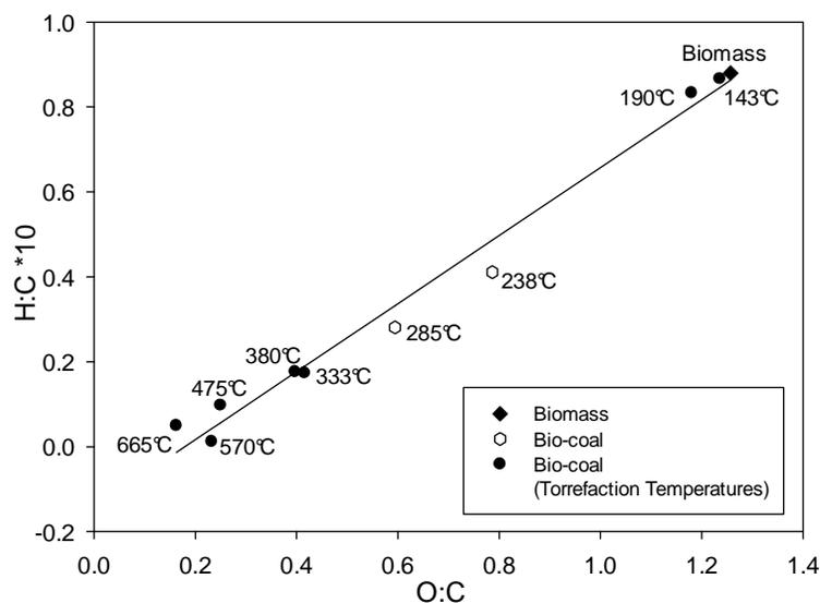
Figure 2-14. Van Krevelen diagram; variation on elemental composition
