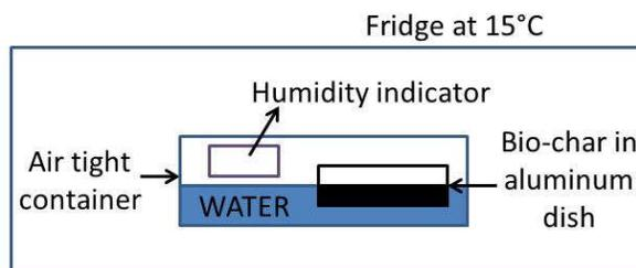
Figure 2-5. Set up for hygroscopy measurement in a controlled saturated atmosphere
