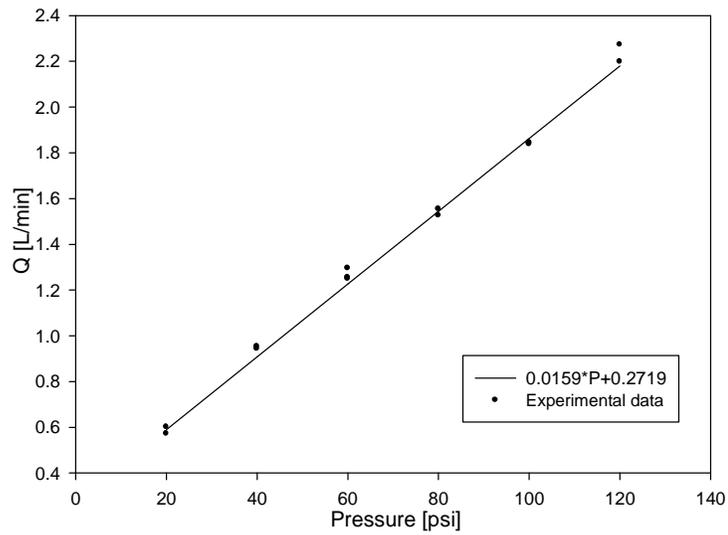
Figure 6-3 Carbon Dioxide Calibration through pressure regulator
