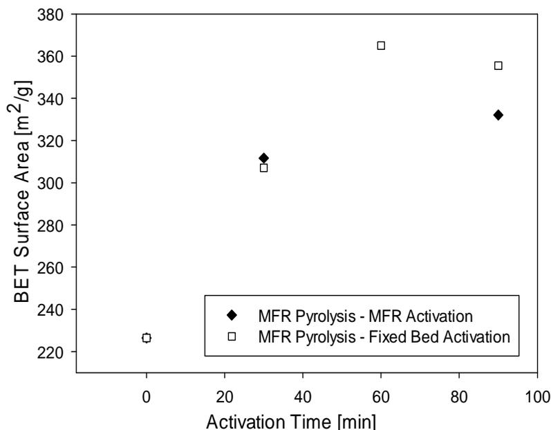
Figure 3-12. Activated Carbon Surface Areas with Consecutive Pyrolysis - Activation in the MFR (Figure 3-6) and Activation in the Fixed Bed (Figure 3-8) (Activation Temperature: 665 °C, CO<sub>2</sub> injection 0.59 L/min, holding times during activation of: 30min, 1h, 1h: 30min)
