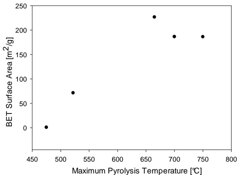
Figure 3-10. Bio-char Surface Areas at Different Maximum Pyrolysis Temperatures
