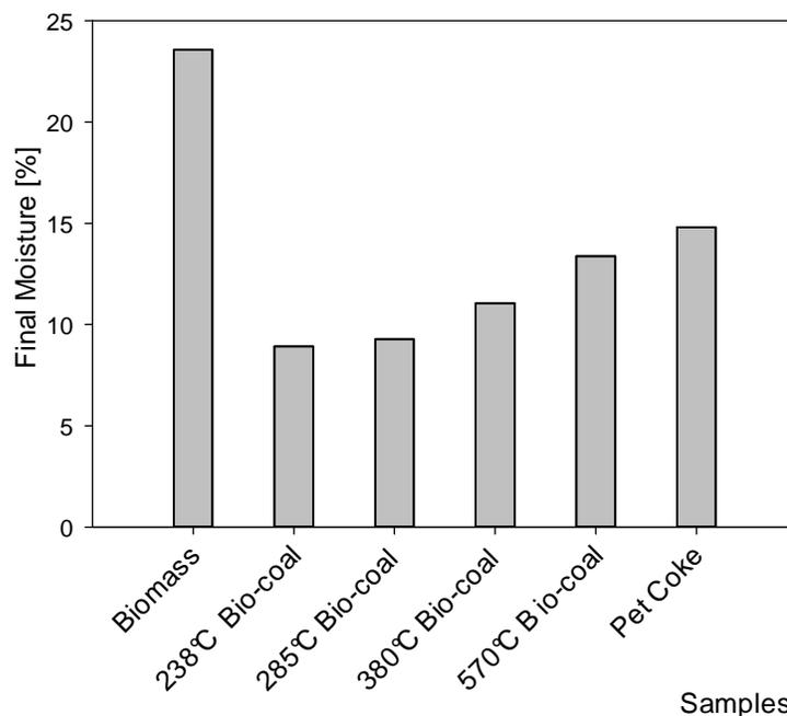
Figure 2-17 Asymptotic hygroscopic values, reported in units of moisture when it has stabilized with time
