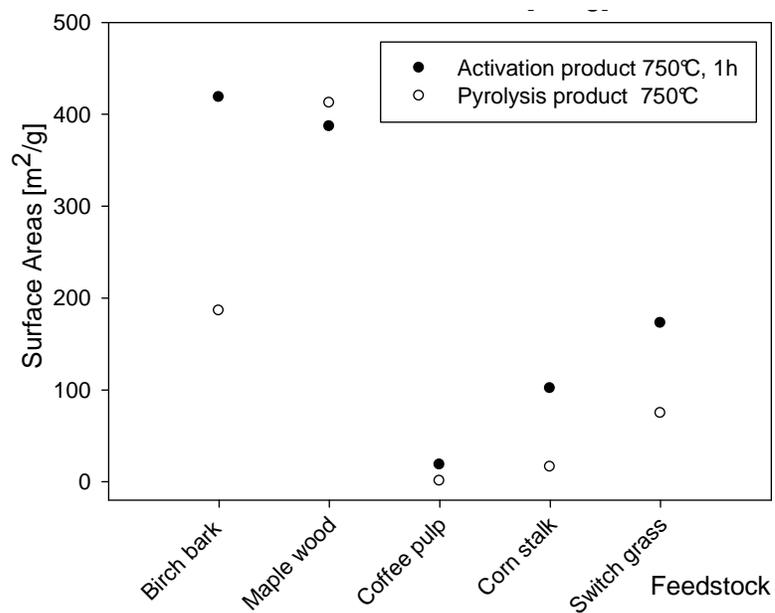
Figure 4-15. Bio-char and activated carbon surface areas for different processed biomasses
