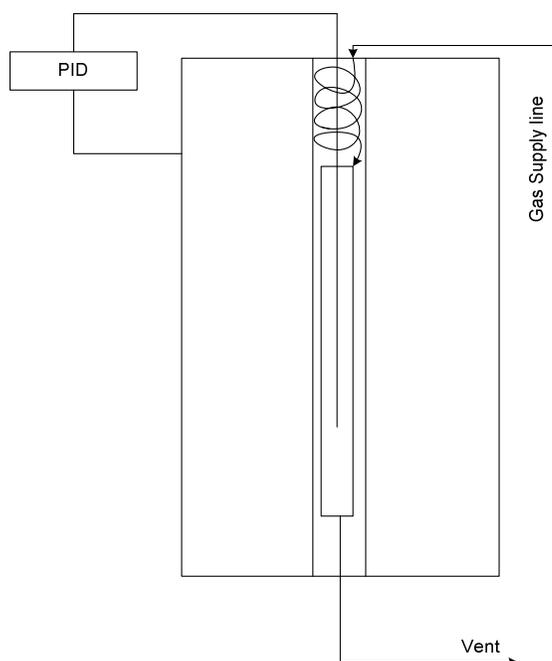
Figure 3-3. Fixed bed reactor diagram in a tubular furnace (1093 °C, 110 V, 8 Amp)
