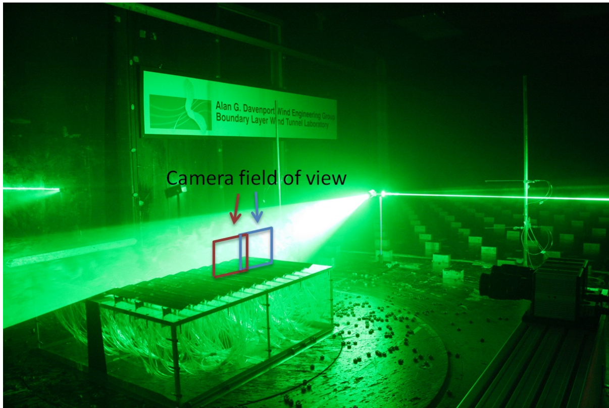
Figure 2.5: Photograph of experimental setup showing positioning of the two fields of view and the laser sheet.
